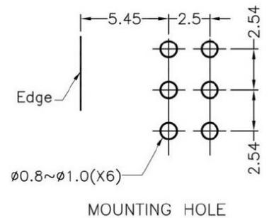
To weld  $\phi 3$  3PIN LED on board with 90 degrees, and same height, but avoid pins broken.
