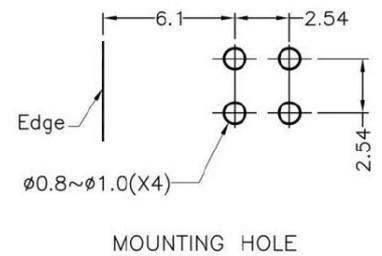
To weld  $\phi 3$  LED on board with 90 degrees, and same height, but avoid pins broken.
