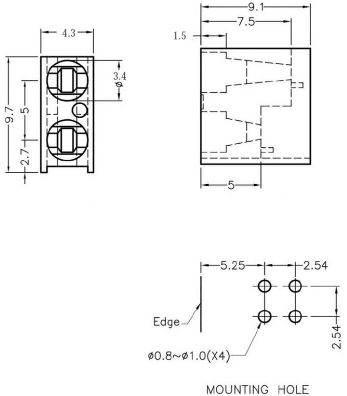
To weld  $\phi 3$  LED on board with 90 degrees, and same height, but avoid pins broken.
