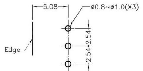
To weld  $\phi 3$  3PIN LED on board with 90 degrees, and same height, but avoid pins broken.
