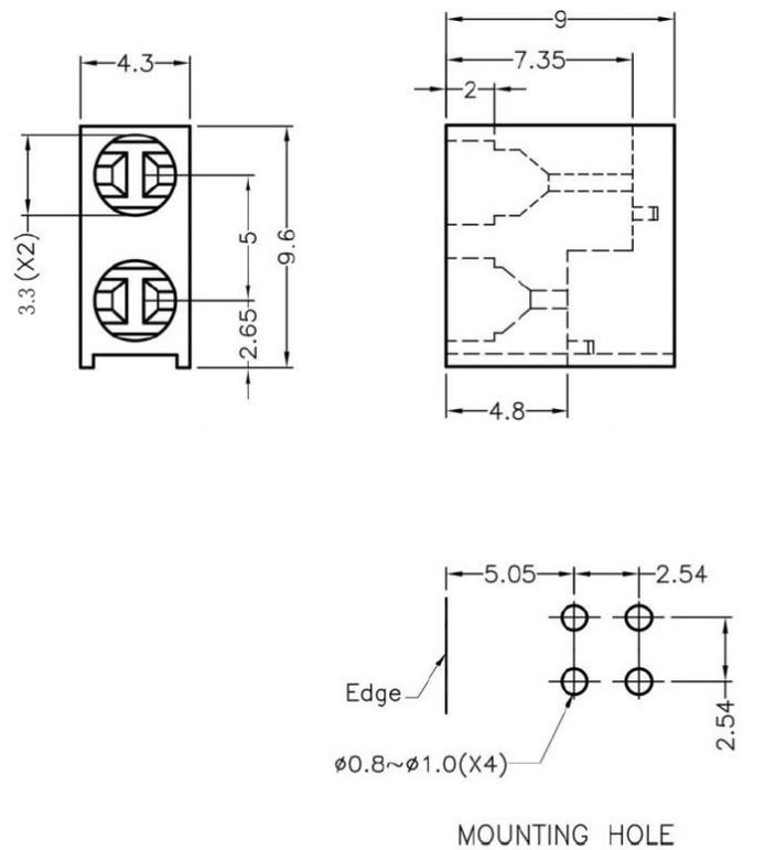
To weld  $\phi 3$  LED on board with 90 degrees, and same height, but avoid pins broken.
