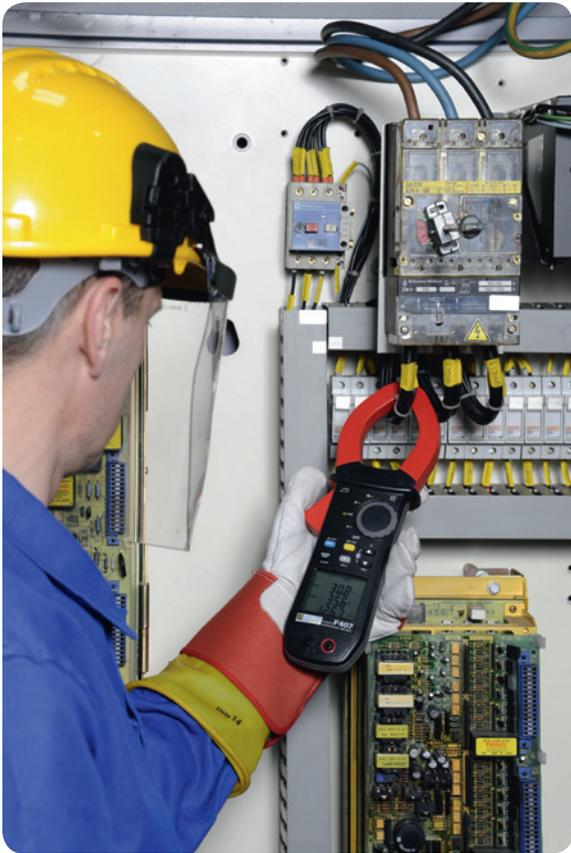
The F407 and F607 clamps can be clamped around a conductor **with just one hand**.
