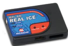
MPLAB REAL ICE In-Circuit Emulator is Microchip's high-speed emulator for PIC MCUs and dsPIC DSCs. It debugs and programs these devices with the easy-to-use but powerful graphical user interface of the MPLAB X IDE.
