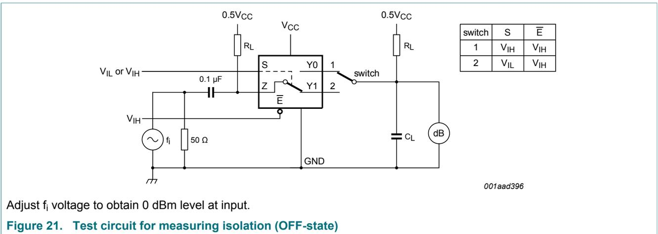
Adjust  $f_i$  voltage to obtain 0 dBm level at input.
