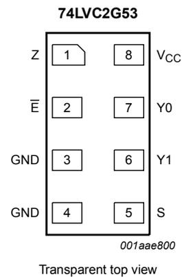
Figure 4. Pin configuration SOT833-1, SOT1089, SOT1116 and SOT1203
