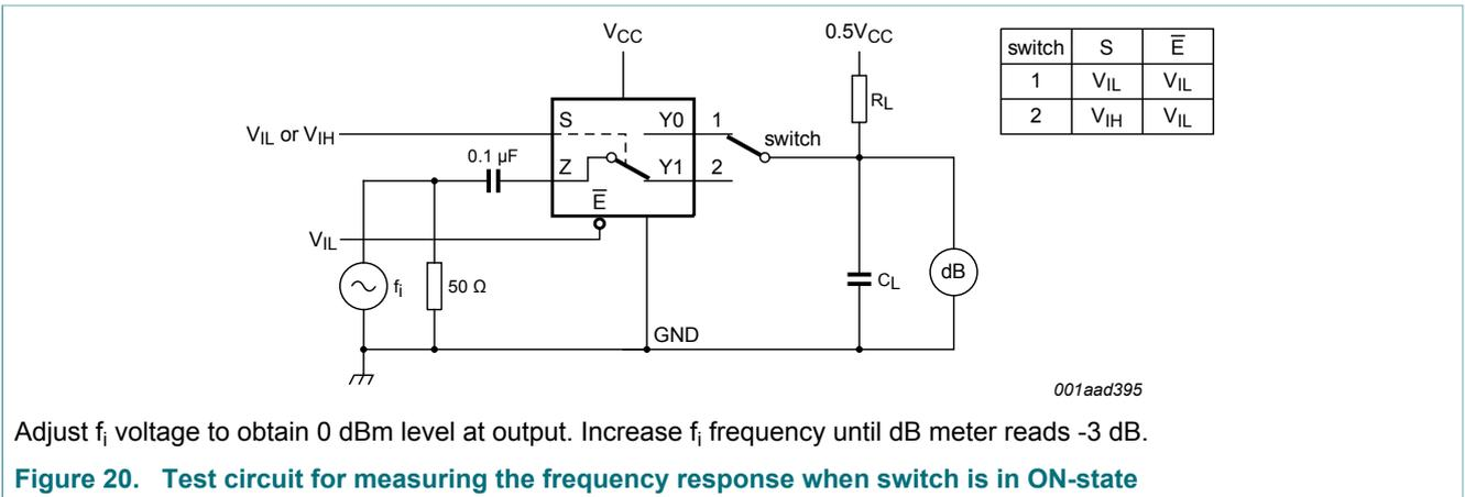
Adjust  $f_i$  voltage to obtain 0 dBm level at output. Increase  $f_i$  frequency until dB meter reads -3 dB.
