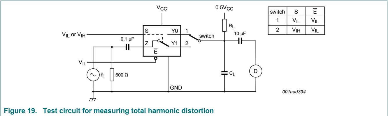
Figure 19. Test circuit for measuring total harmonic distortion
