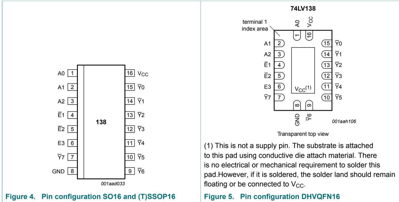
Figure 4. Pin configuration SO16 and (T)SSOP16
