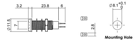
Anode termination indicated by red sleeve. Mounting hole to be clean and burr free.
