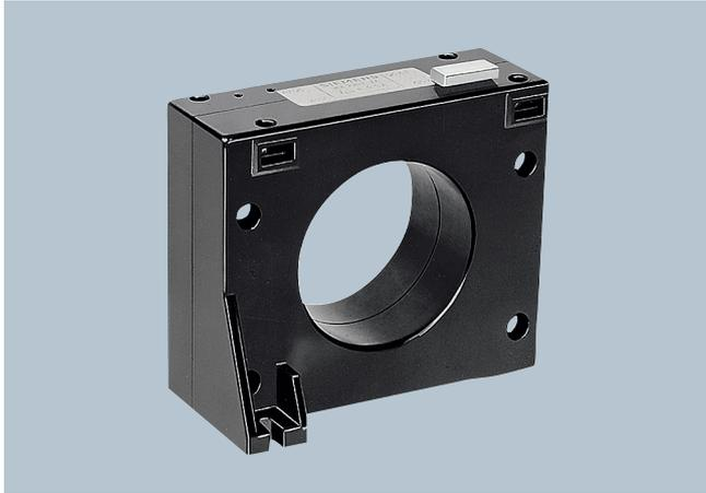
The 3UL22 summation current transformers detect fault currents in machines and plants. Together with the 3UG46 24 residual current monitoring relay or the SIMOCODE 3UF motor management and control device they enable residual-current and ground-fault monitoring.
