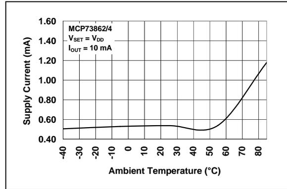
**FIGURE 2-22:** Supply Current ( $I_{SS}$ ) vs. Ambient Temperature ( $T_A$ ).
