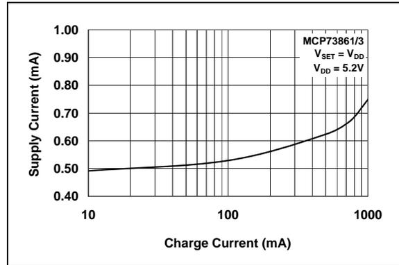
**FIGURE 2-4:** Supply Current ( $I_{SS}$ ) vs. Charge Current ( $I_{OUT}$ ).
