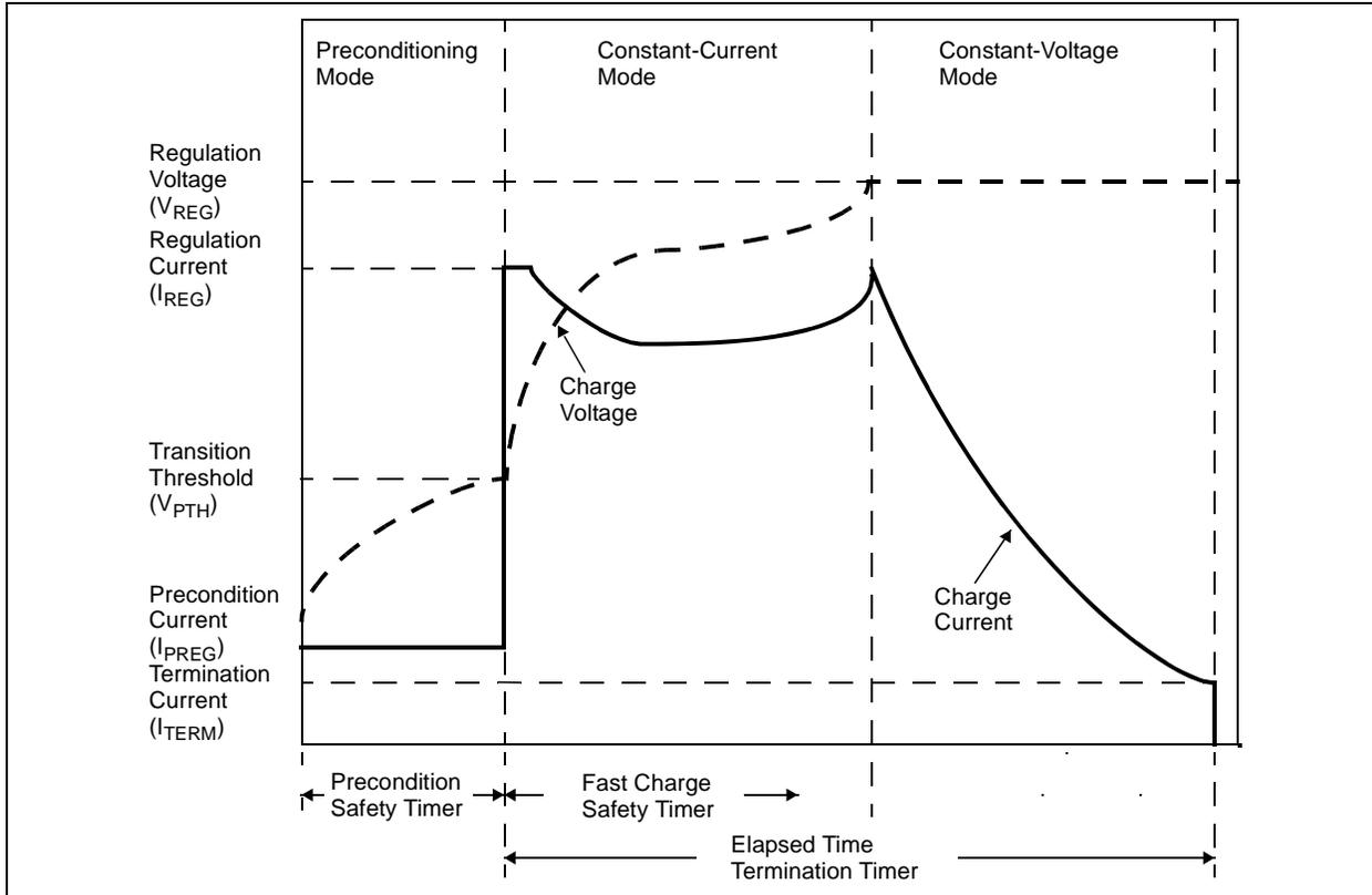
**FIGURE 6-3:** Typical Charge Profile in Thermal Regulation.
