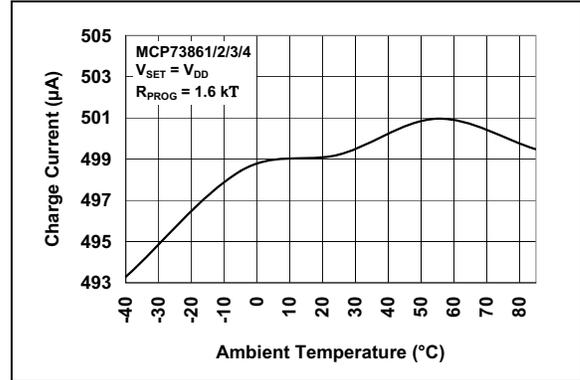
**FIGURE 2-32:** Charge Current ( $I_{OUT}$ ) vs. Ambient Temperature ( $T_A$ ).
