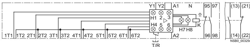
A1, A2, A3 Connections of the control voltage
