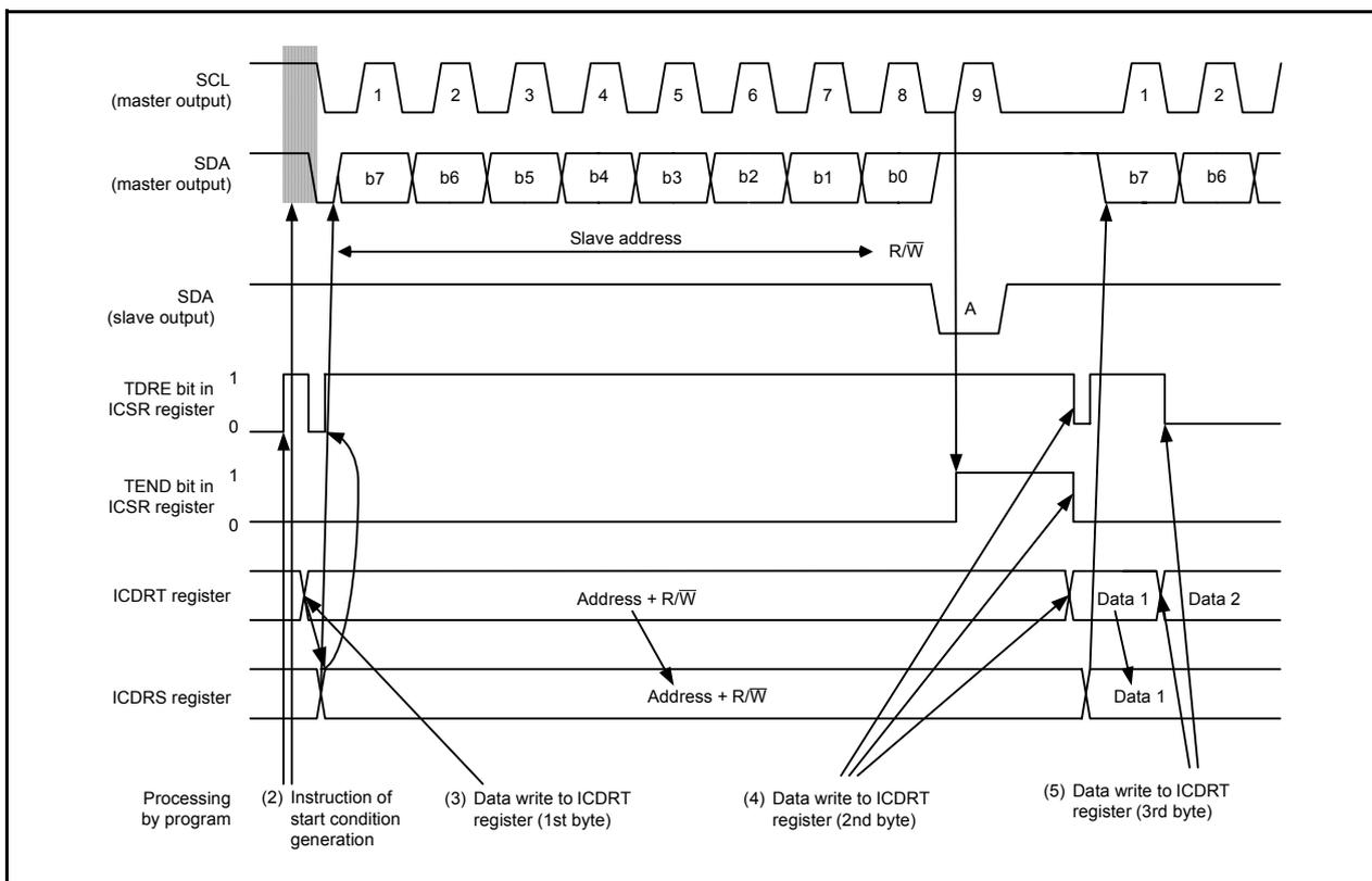
Figure 16.35 Operating Timing in Master Transmit Mode (I<sup>2</sup>C bus Interface Mode) (1)
