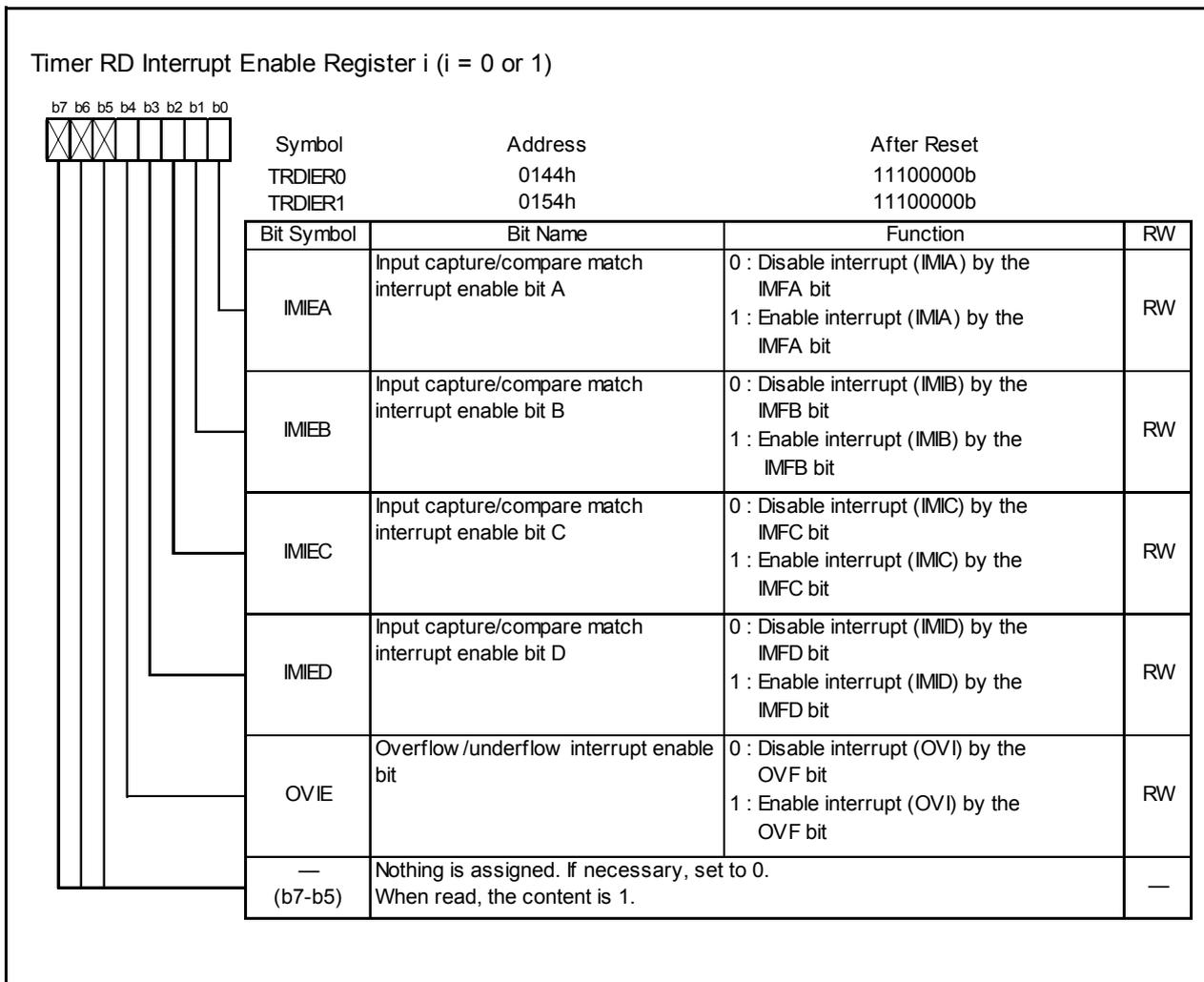
Figure 14.108 Registers TRDIER0 to TRDIER1 in PWM Mode
