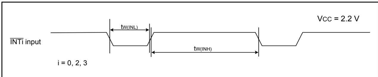
**Figure 21.22 External Interrupt  $\overline{INTi}$  Input Timing Diagram when  $V_{cc} = 2.2 V$**
