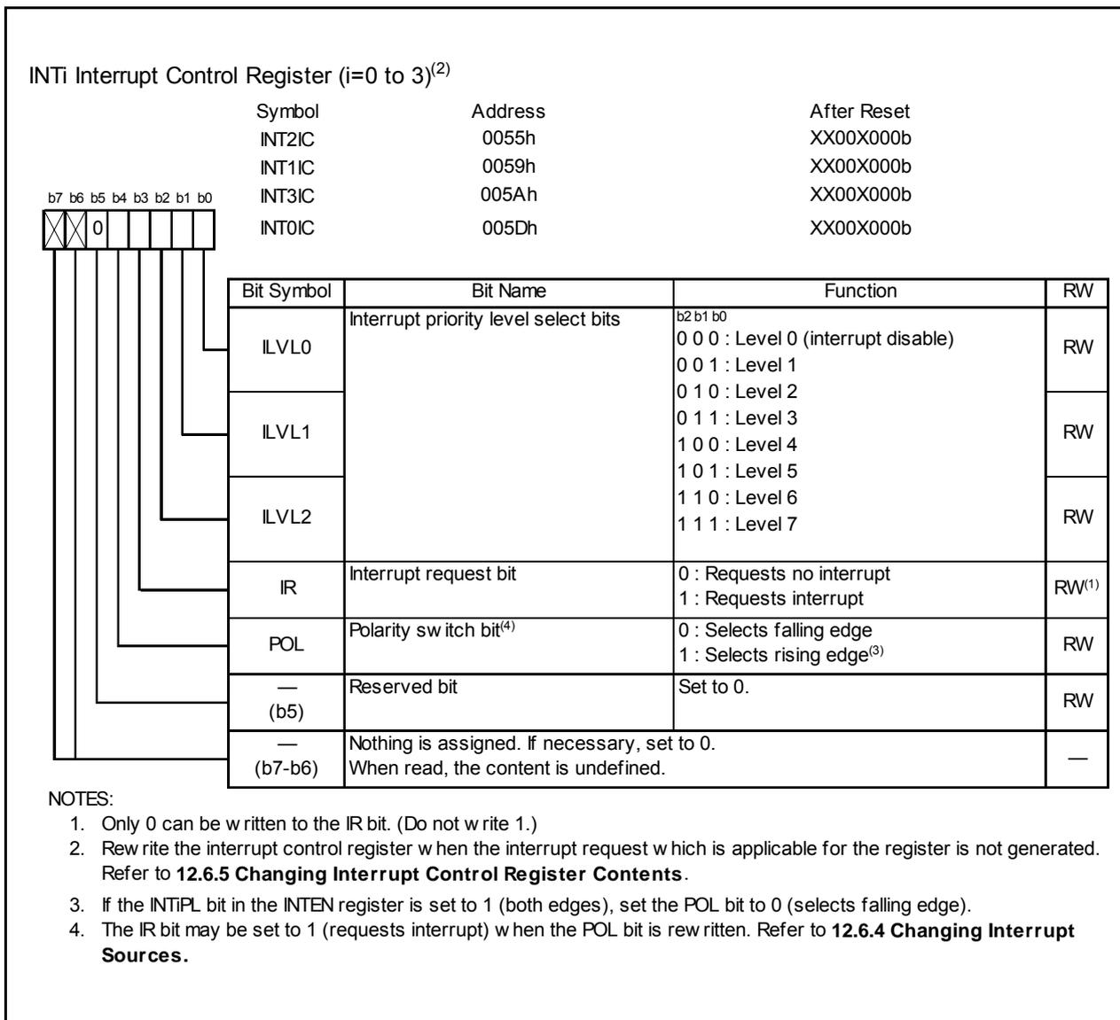
Figure 12.5 INT<sub>i</sub>IC Register
