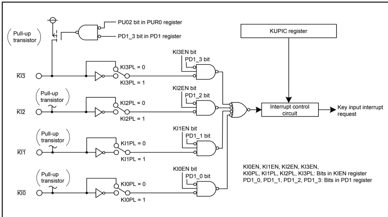
Figure 12.18 Block Diagram of Key Input Interrupt
