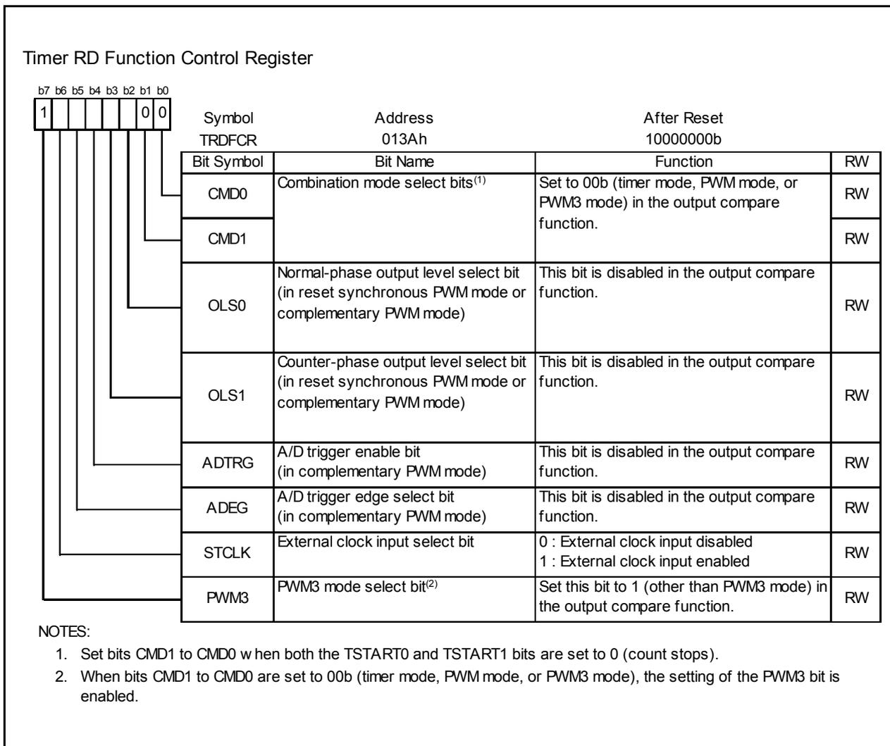
Figure 14.87 TRDFCR Register in Output Compare Function
