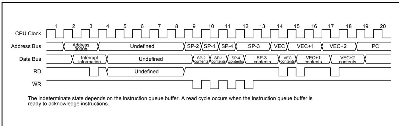
**Figure 12.6 Time Required for Executing Interrupt Sequence**
