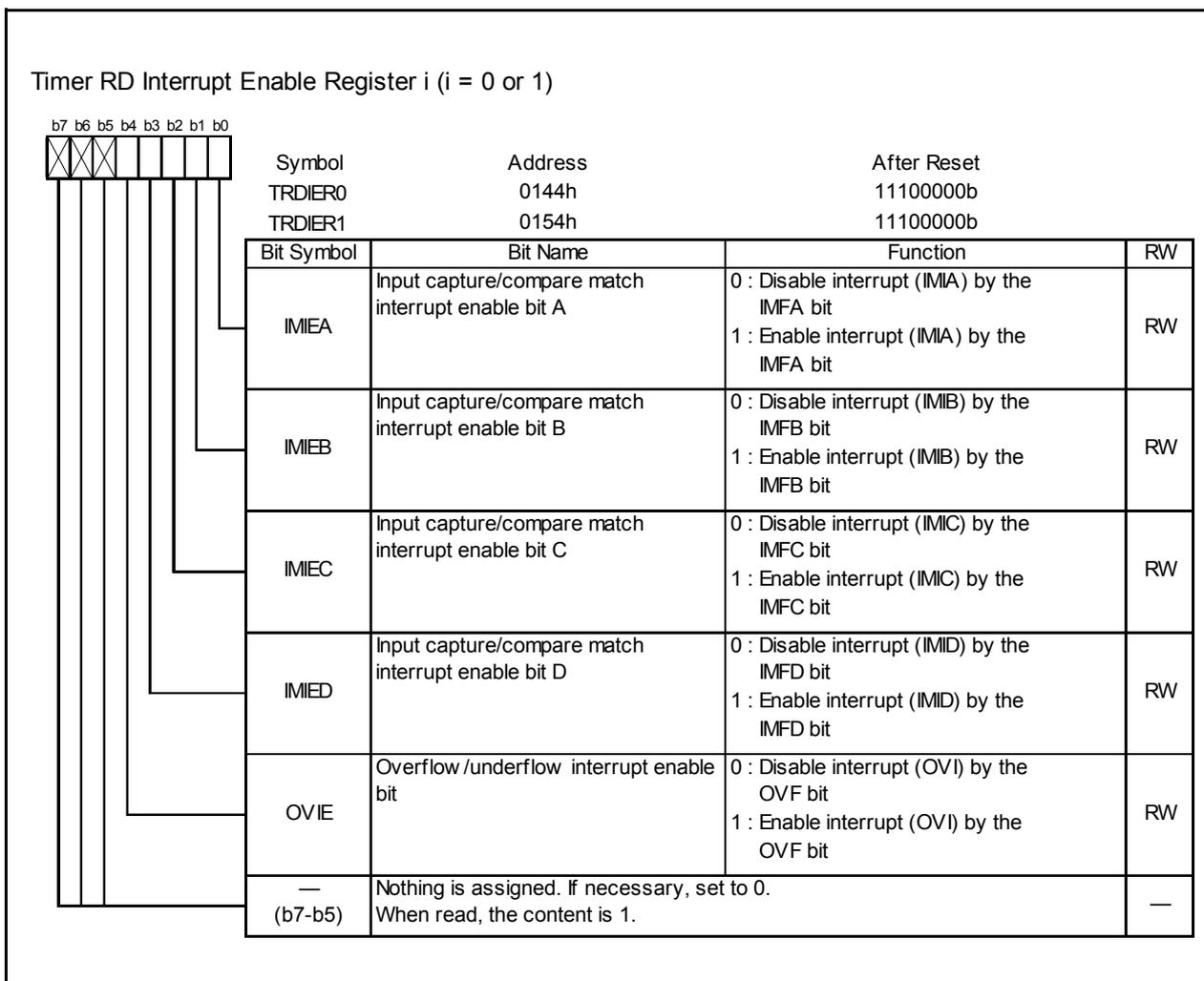
Figure 14.147 Registers TRDIER0 to TRDIER1 in PWM3 Mode
