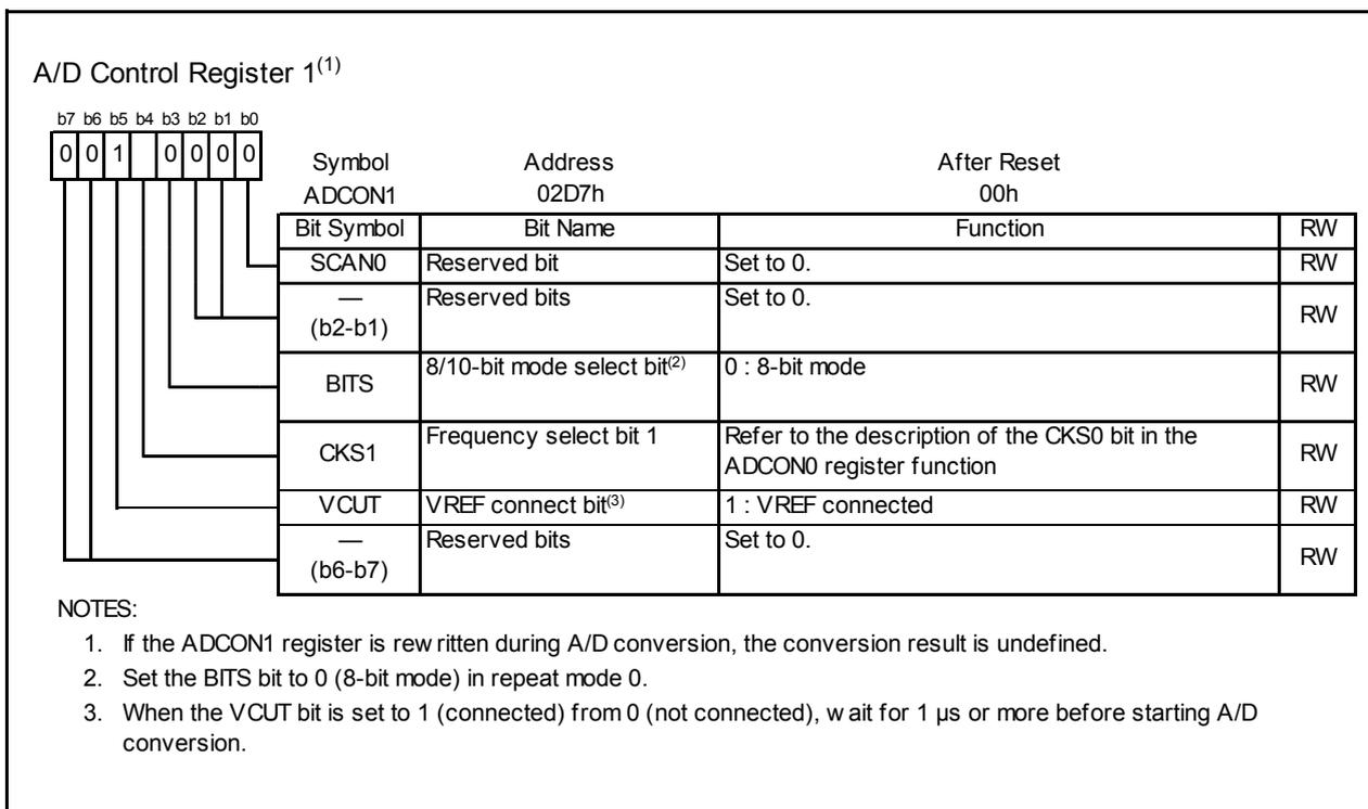
**Figure 18.8 ADCON1 Register in Repeat Mode 0**
