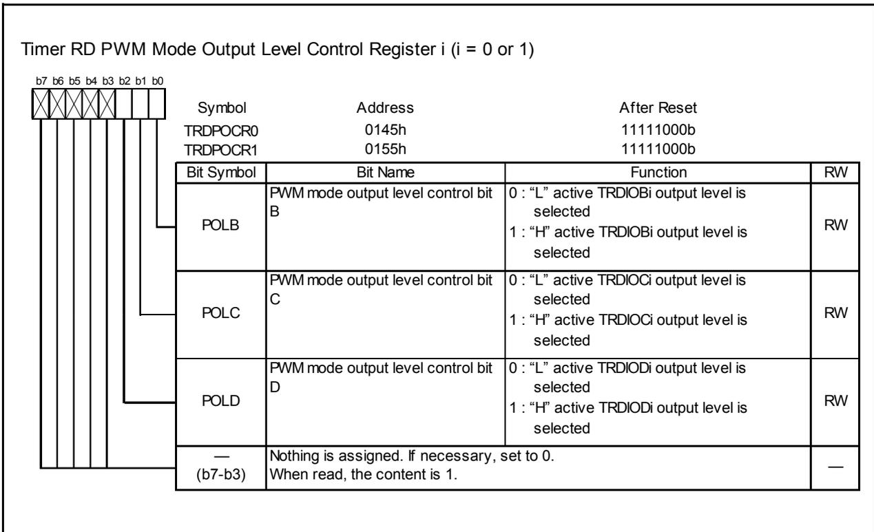
Figure 14.109 Registers TRDPOCR0 to TRDPOCR1 in PWM Mode
