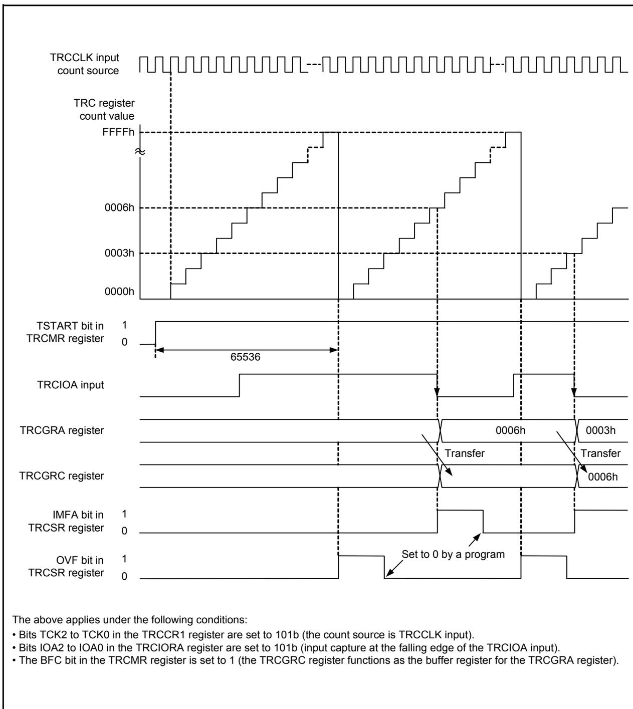
Figure 14.46 Operating Example of Input Capture Function
