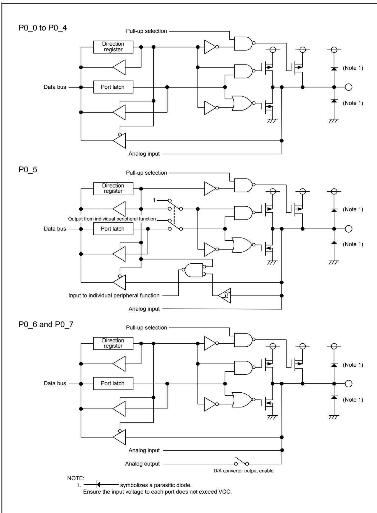
Figure 7.1 Configuration of Programmable I/O Ports (1)
