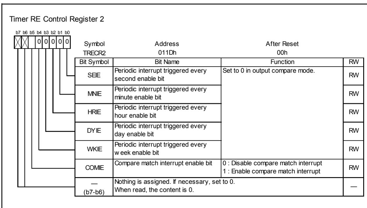
Figure 14.170 TREC2 Register in Output Compare Mode
