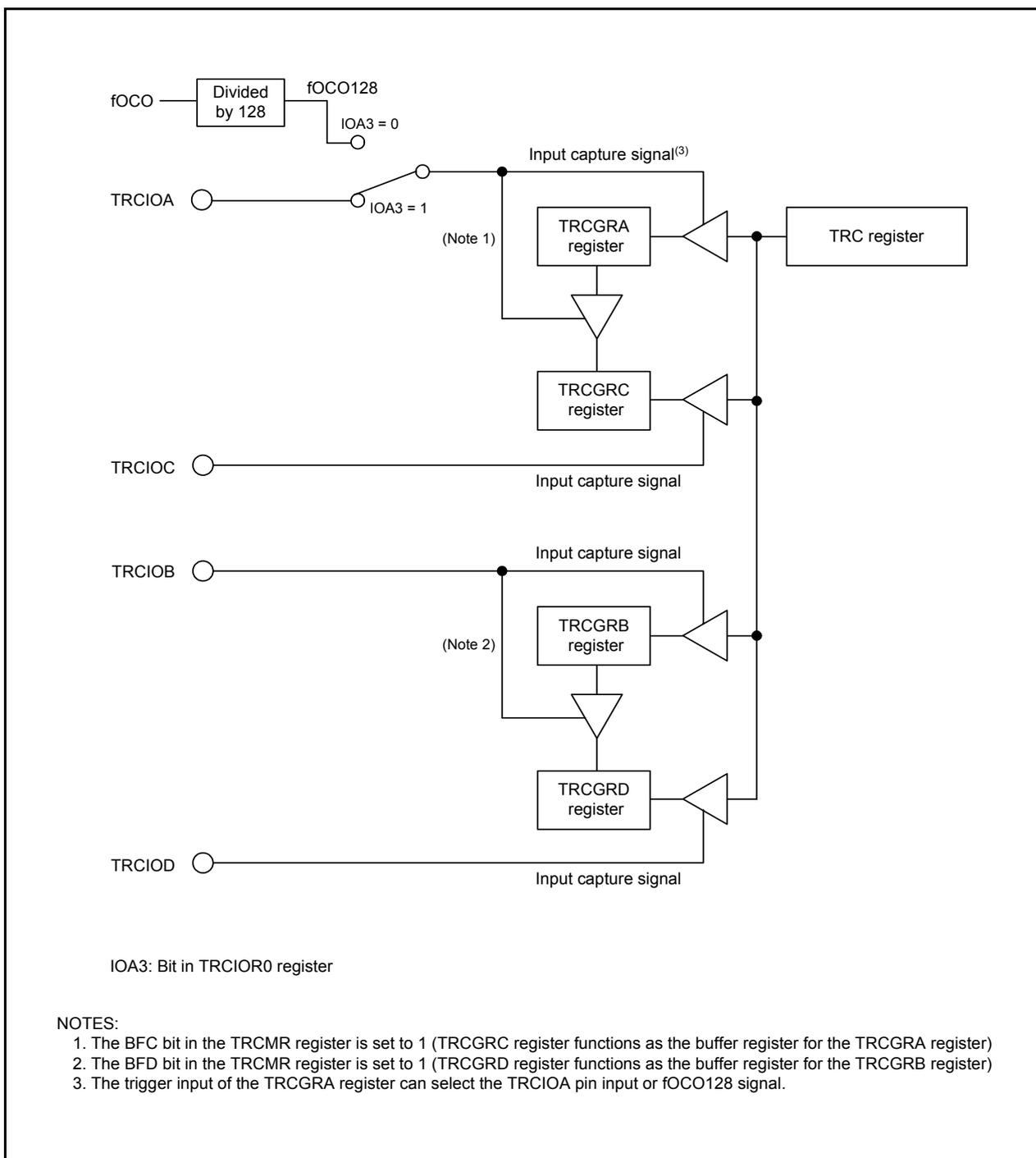
Figure 14.43 Block Diagram of Input Capture Function
