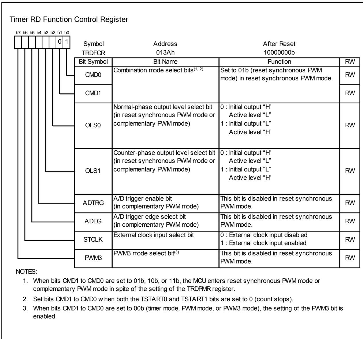
Figure 14.117 TRDFCR Register in Reset Synchronous PWM Mode
