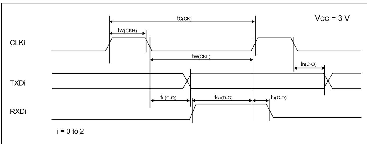
**Figure 21.16 Serial Interface Timing Diagram when Vcc = 3 V**
