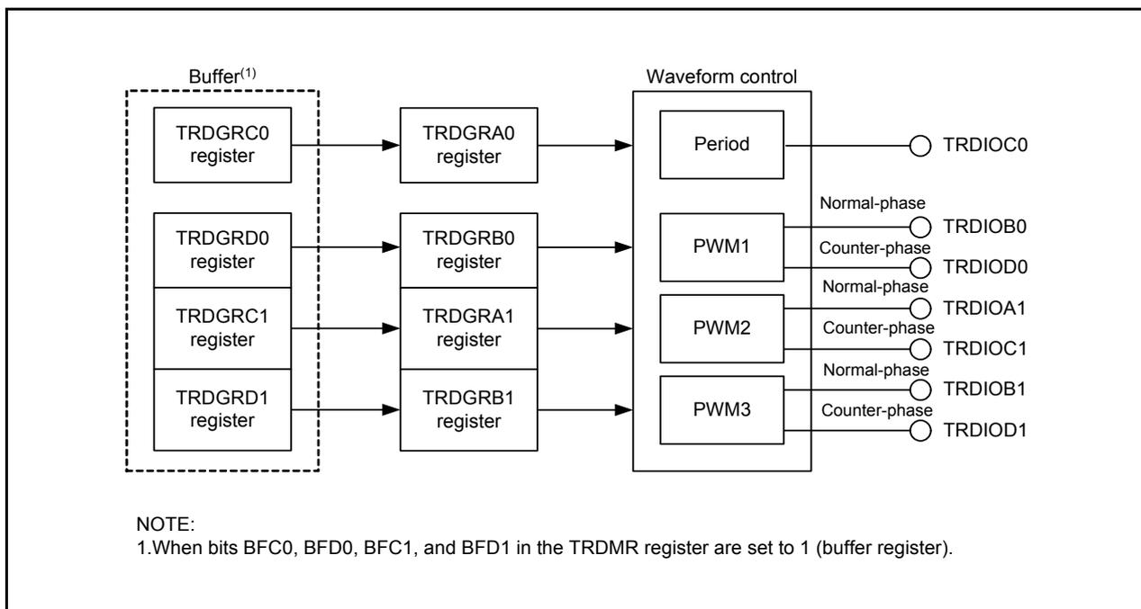
Figure 14.114 Block Diagram of Reset Synchronous PWM Mode
