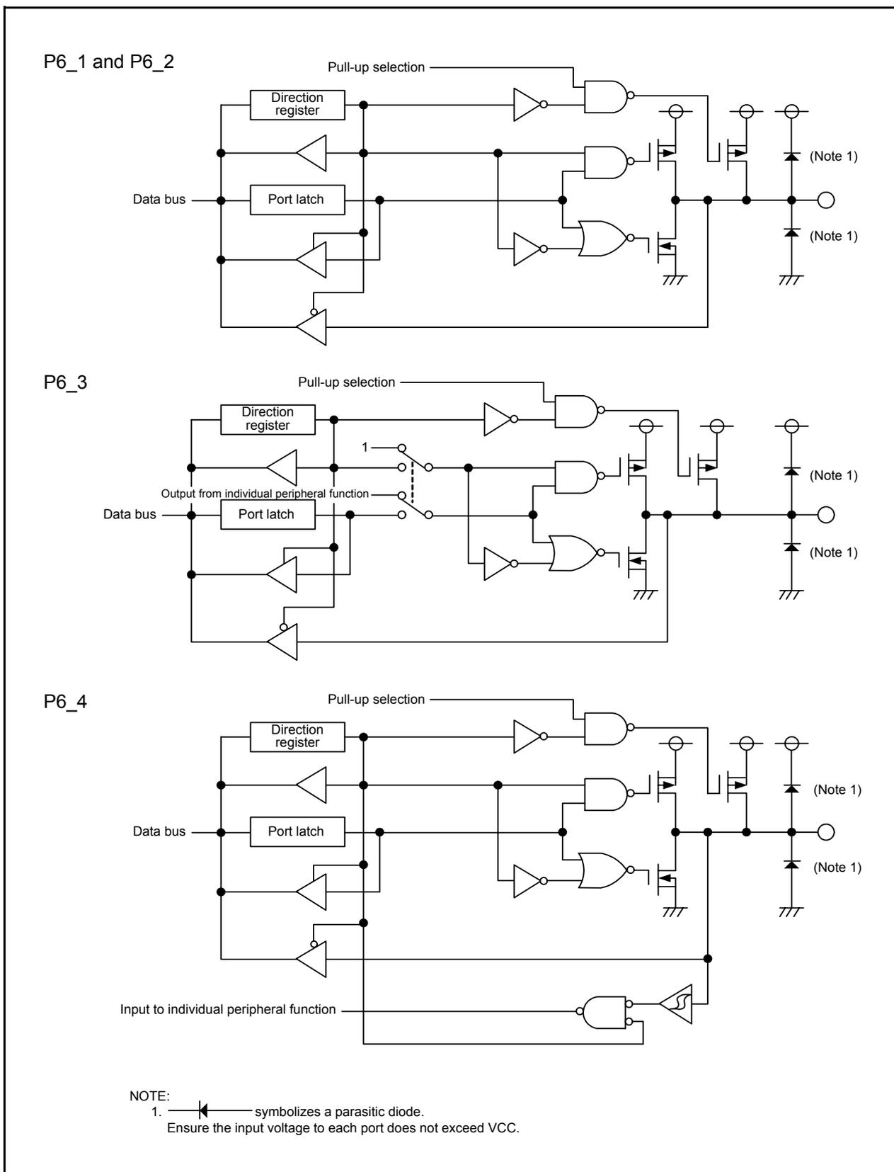
Figure 7.8 Configuration of Programmable I/O Ports (8)
