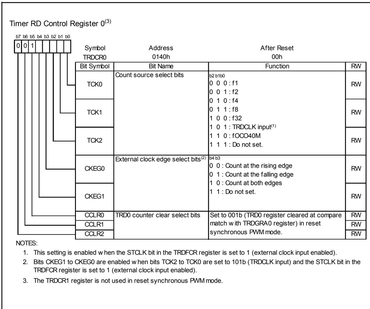
Figure 14.119 TRDCR0 Register in Reset Synchronous PWM Mode
