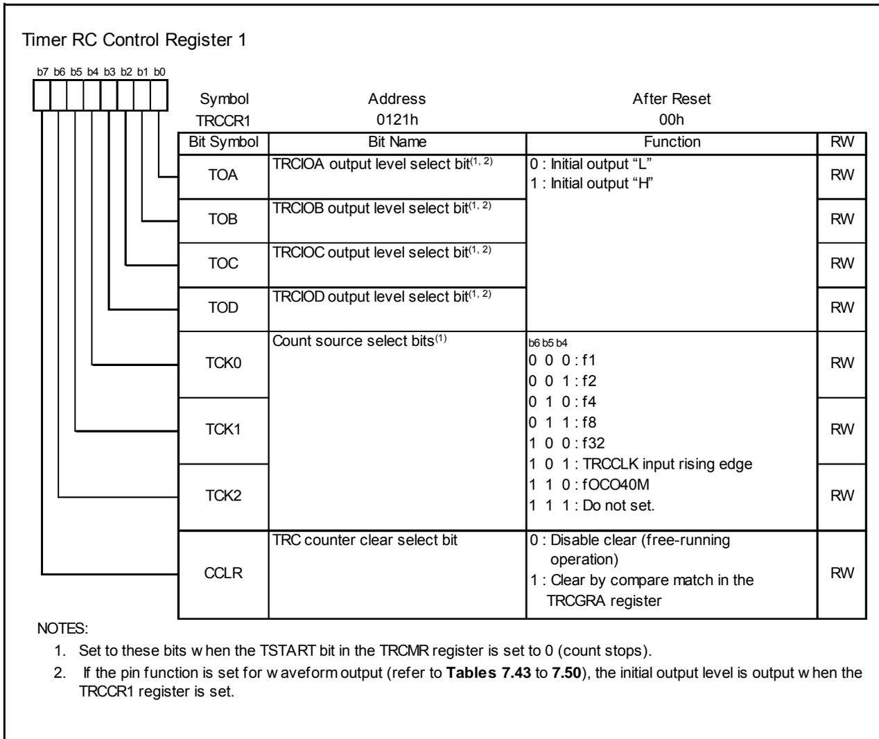
Figure 14.50 TRCCR1 Register for Output Compare Function
