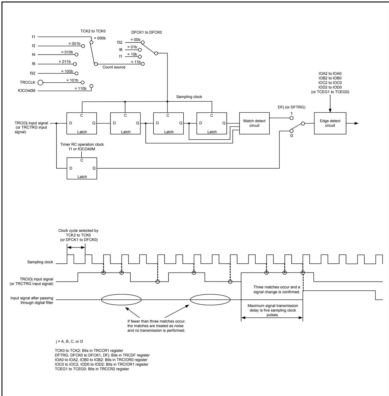
Figure 14.41 Block Diagram of Digital Filter
