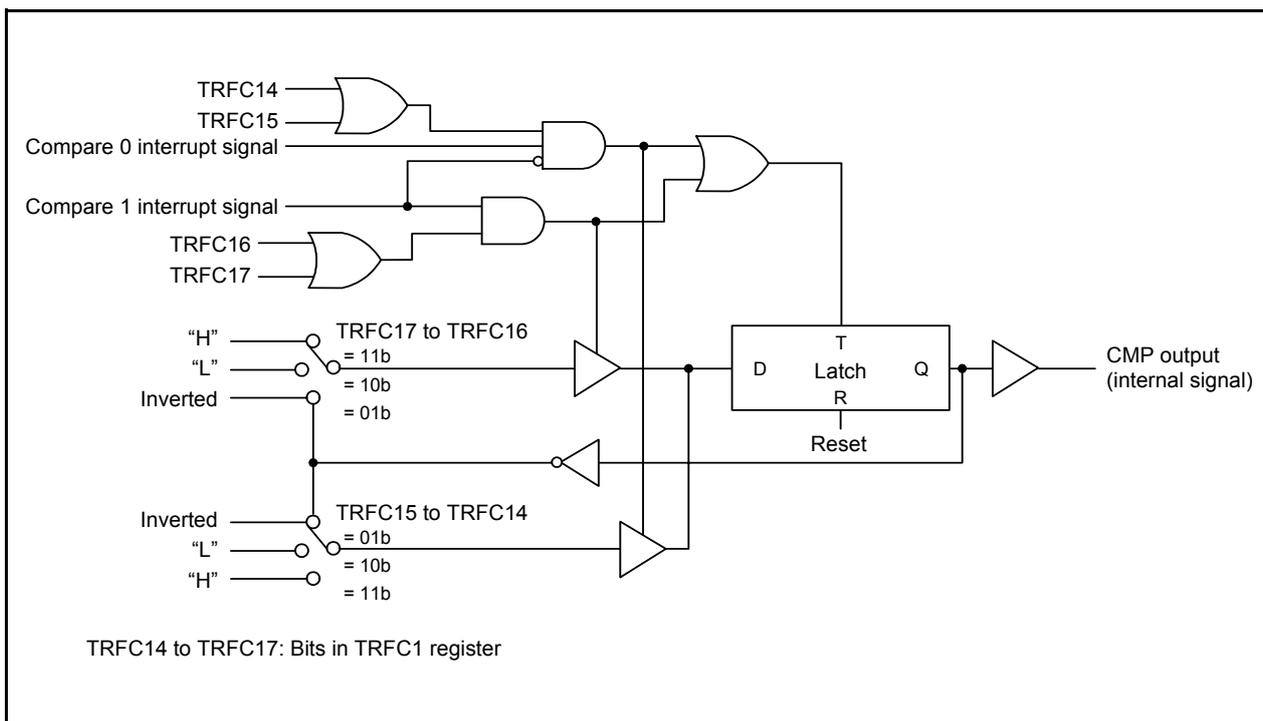
Figure 14.175 Block Diagram of CMP Waveform Generation Unit
