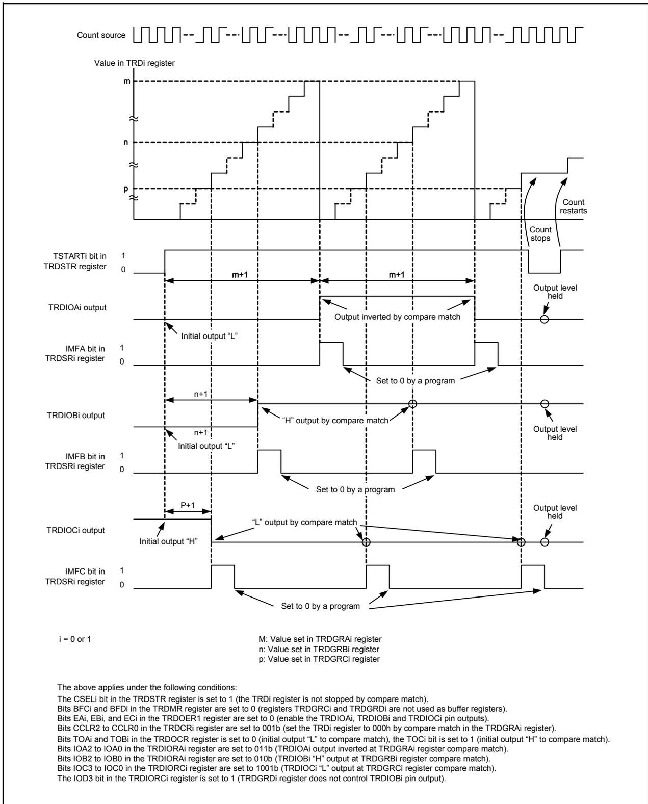
Figure 14.97 Operating Example of Output Compare Function
