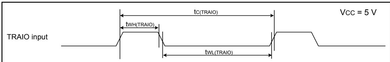
**Figure 21.9 TRAIO Input and  $\overline{\text{INT1}}$  Input Timing Diagram when  $V_{CC} = 5\text{ V}$** **Table 21.20 TRFI Input**
