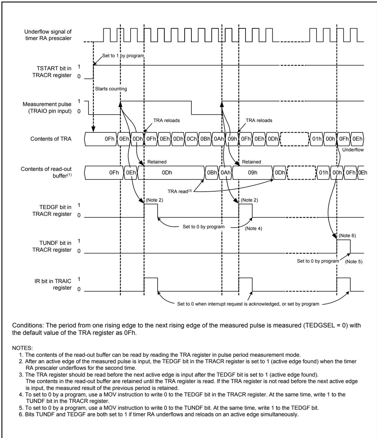
**Figure 14.11 Operating Example of Pulse Period Measurement Mode**
