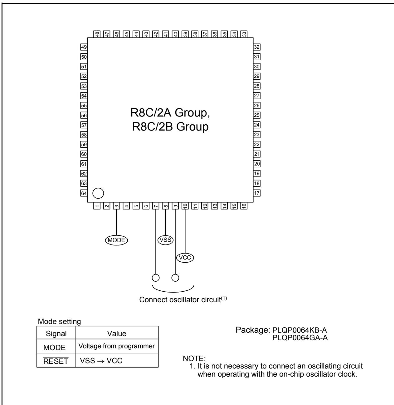
Figure 20.17 Pin Connections for Standard Serial I/O Mode 3
