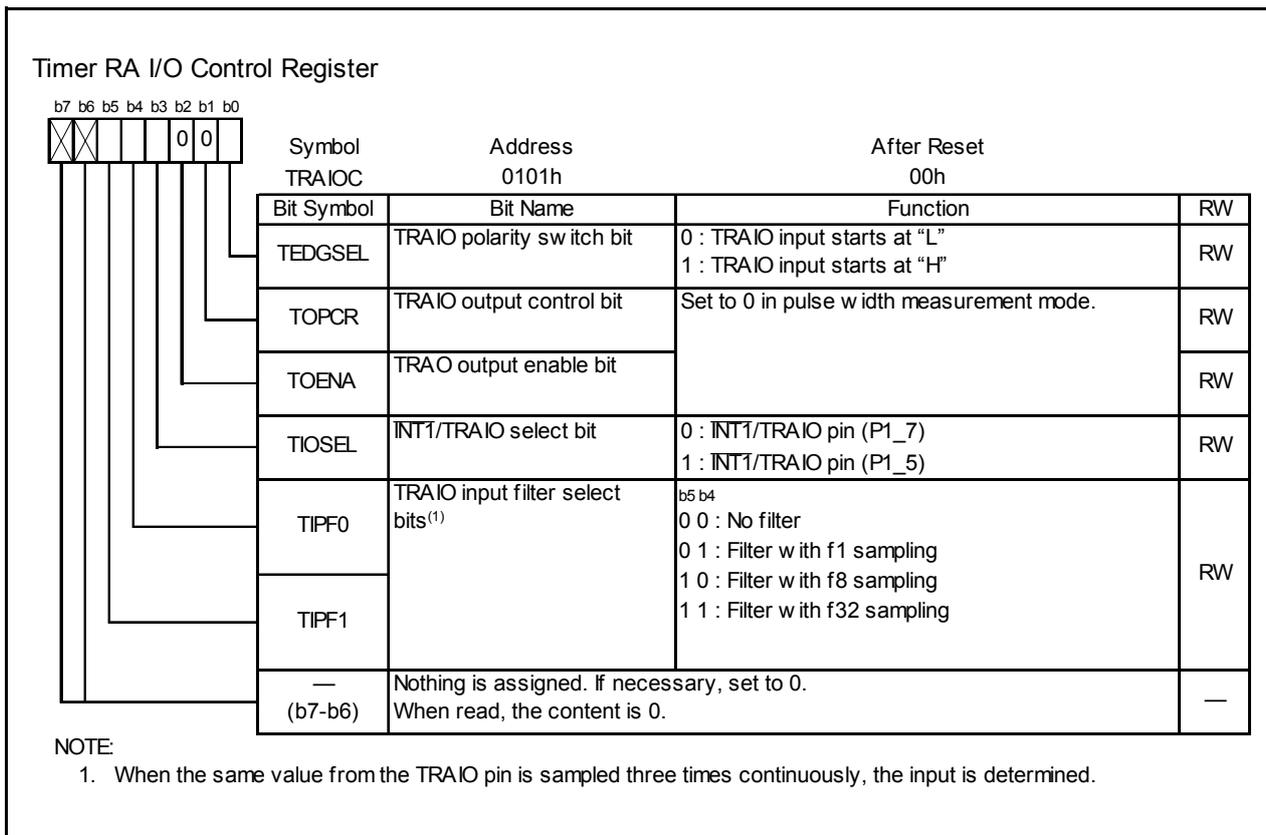
Figure 14.8 TRATIO Register in Pulse Width Measurement Mode
