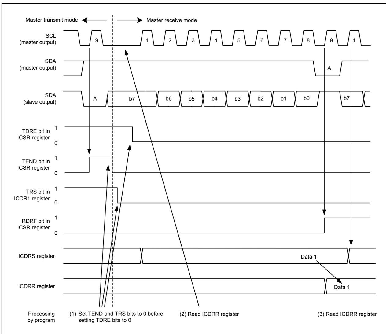
Figure 16.37 Operating Timing in Master Receive Mode (I<sup>2</sup>C bus Interface Mode) (1)
