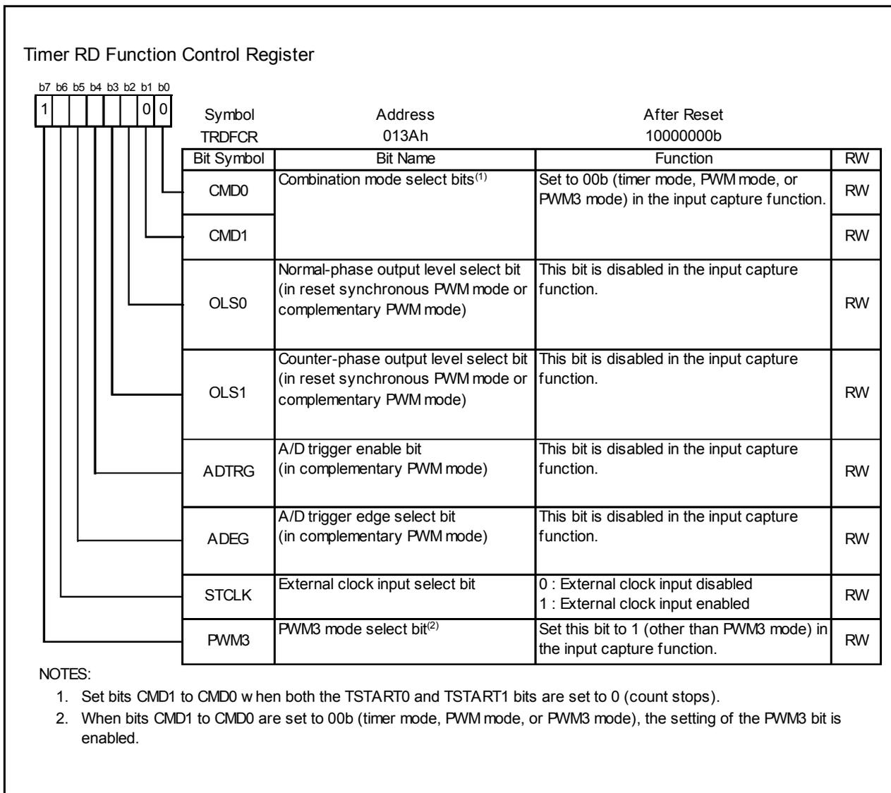
Figure 14.72 TRDFCR Register in Input Capture Function
