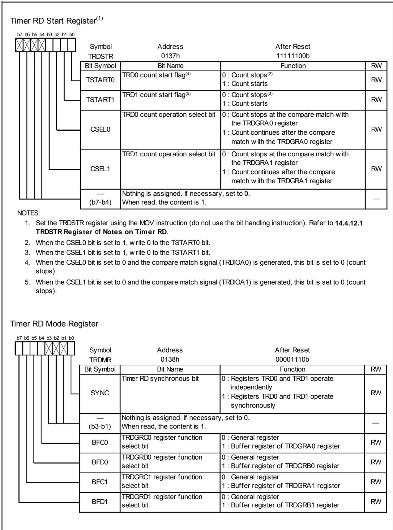
Figure 14.102 Registers TRDSTR and TRDMR in PWM Mode
