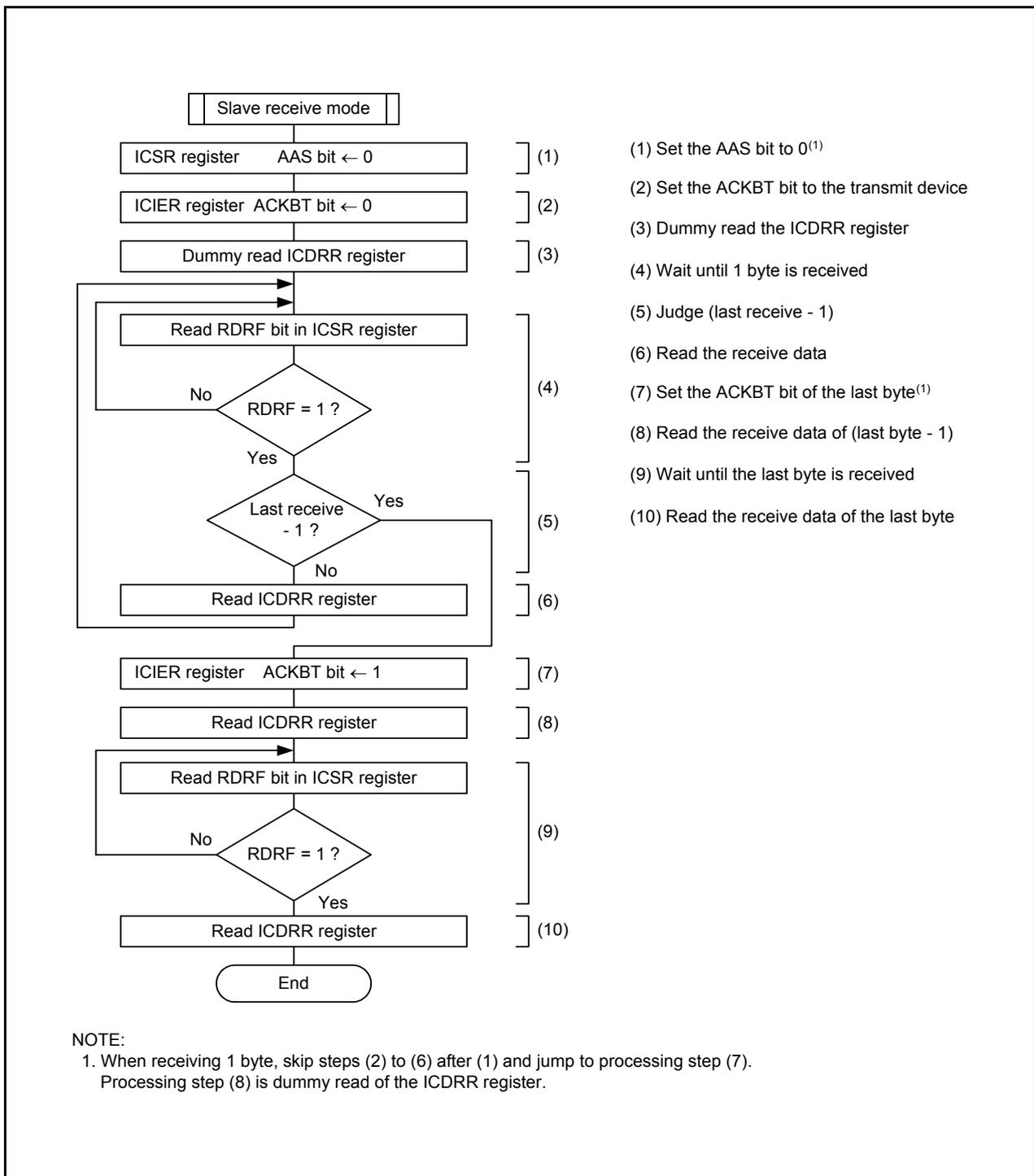
Figure 16.49 Example of Register Setting in Slave Receive Mode (I<sup>2</sup>C bus Interface Mode)
