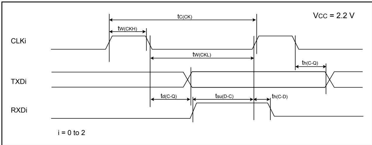
**Figure 21.21 Serial Interface Timing Diagram when  $V_{cc} = 2.2 V$**
