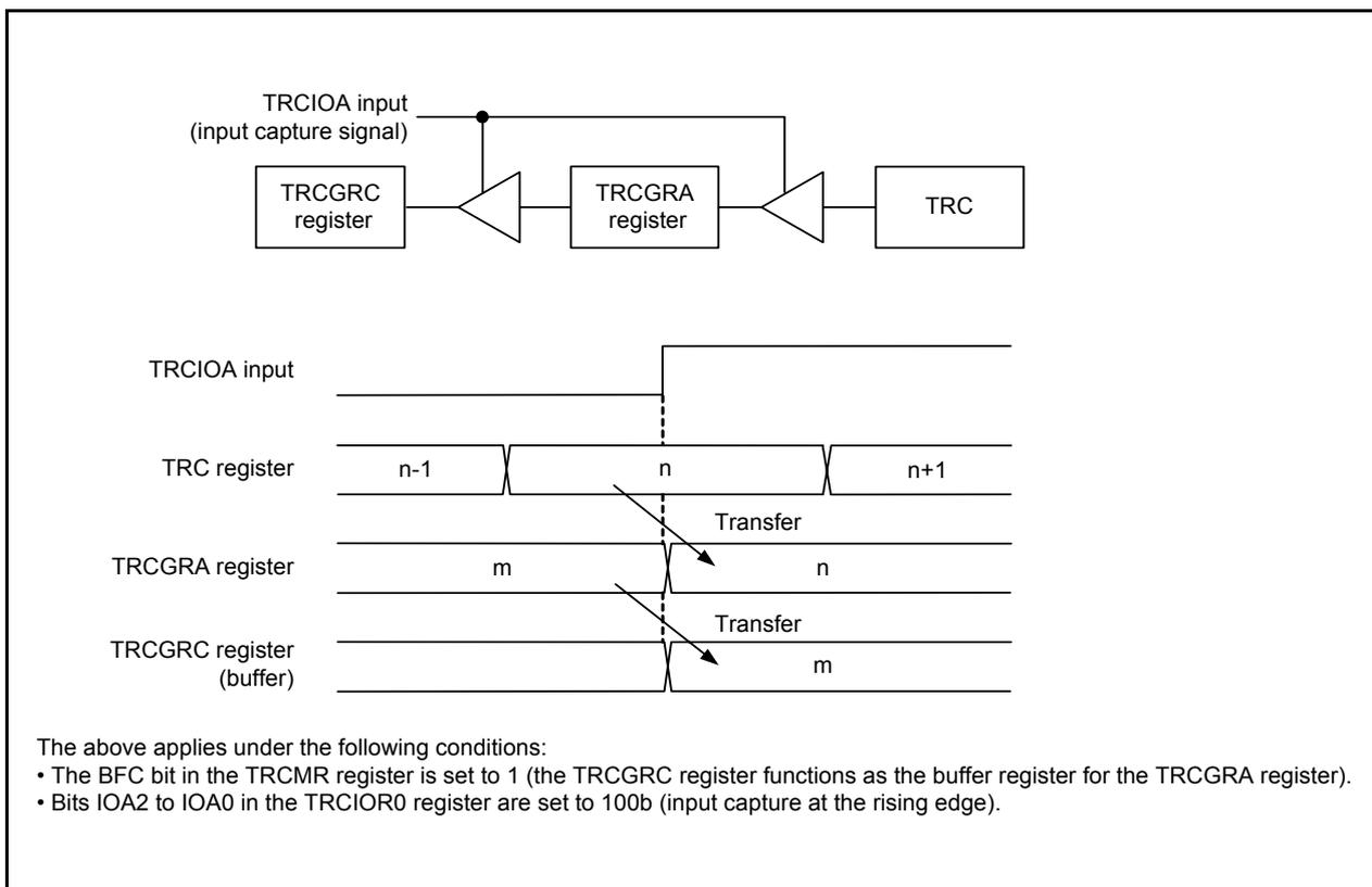
**Figure 14.39 Buffer Operation for Input Capture Function**
