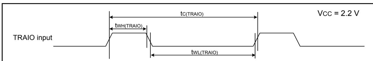
**Figure 21.19 TRAIO Input and  $\overline{\text{INT1}}$  Input Timing Diagram when  $V_{CC} = 2.2\text{ V}$** **Table 21.34 TRFI Input**
