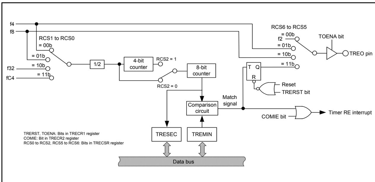
Figure 14.166 Block Diagram of Output Compare Mode
