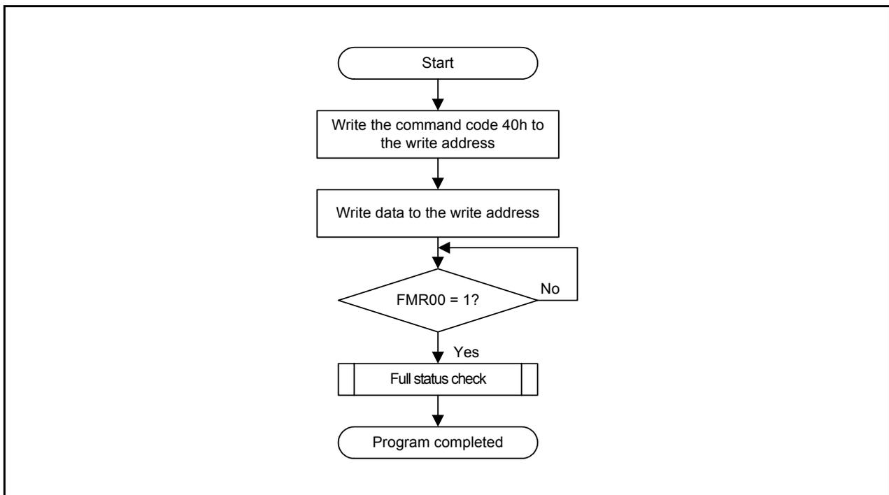
Figure 20.12 Program Command (When Suspend Function Disabled)
