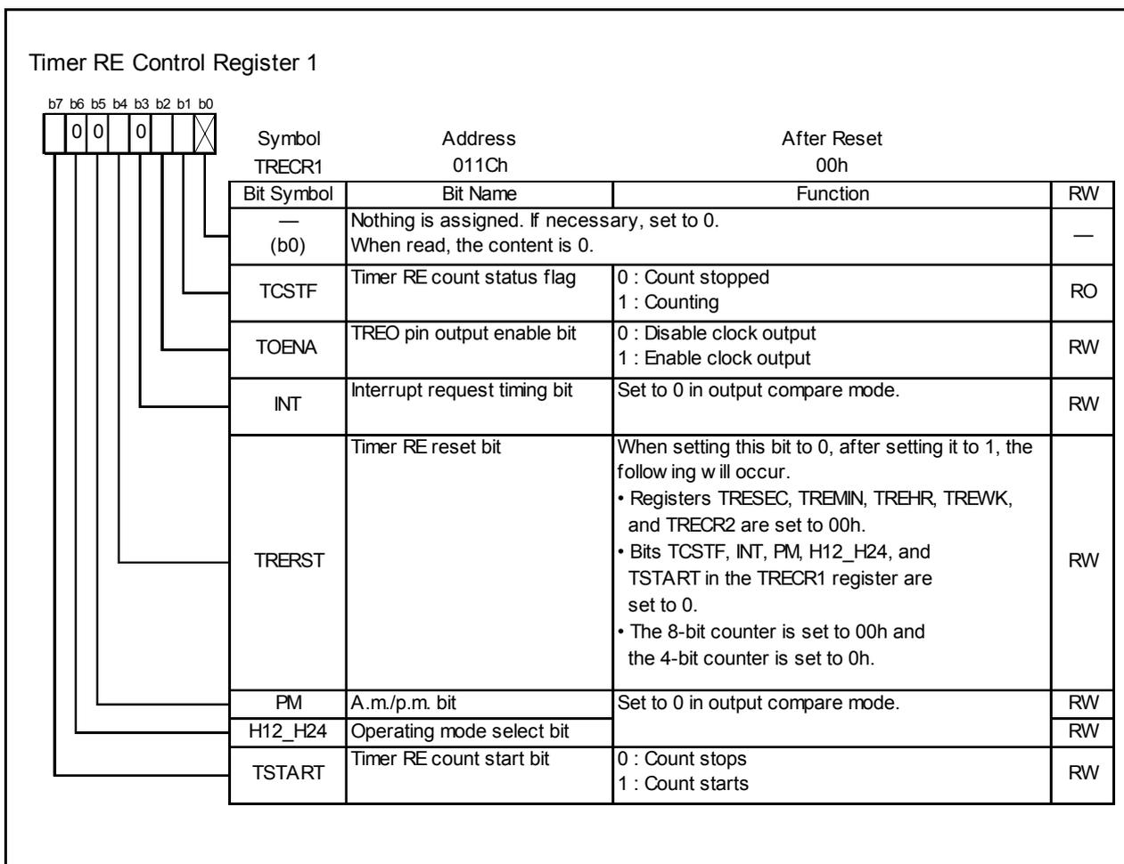
Figure 14.169 TREC1 Register in Output Compare Mode
