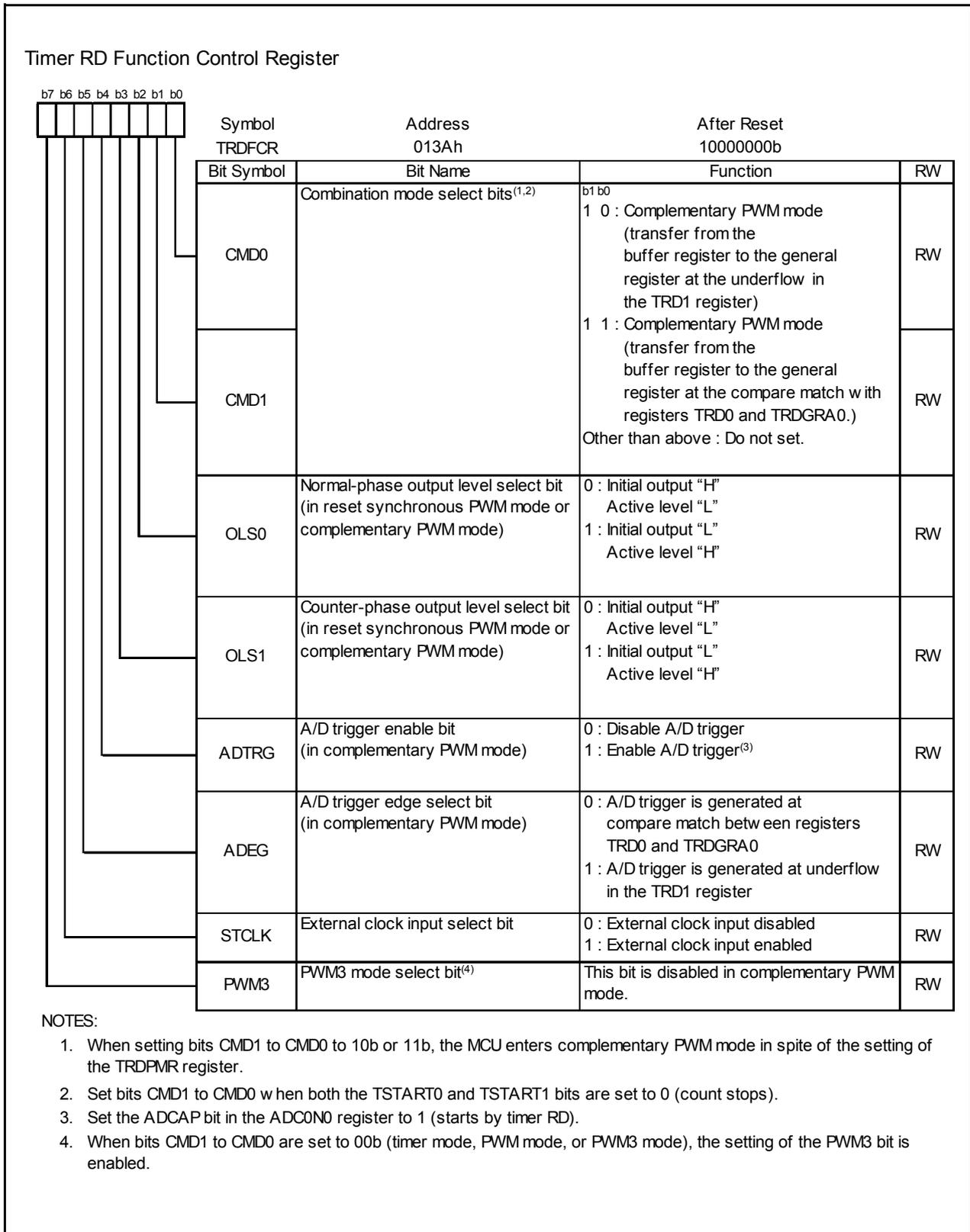
Figure 14.129 TRDFCR Register in Complementary PWM Mode
