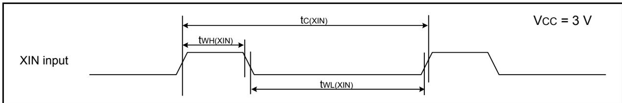
**Figure 21.13 XIN Input and XCIN Input Timing Diagram when  $V_{CC} = 3\text{ V}$** **Table 21.26 TRAIO Input,  $\overline{\text{INT1}}$  Input**
