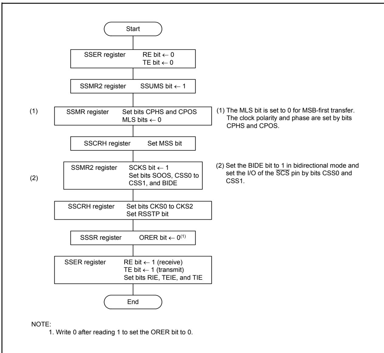
Figure 16.19 Initialization in 4-Wire Bus Communication Mode
