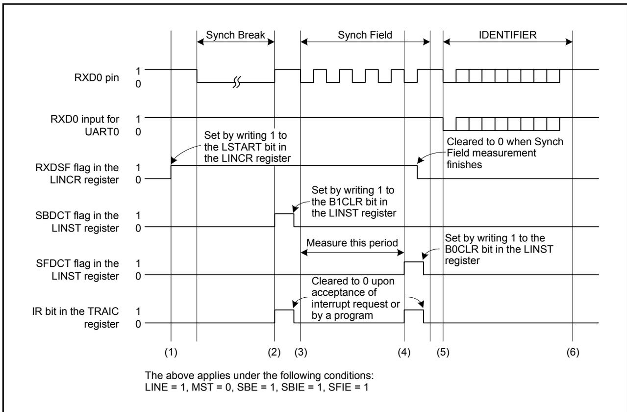
**Figure 17.7 Typical Operation when Receiving a Header Field**
