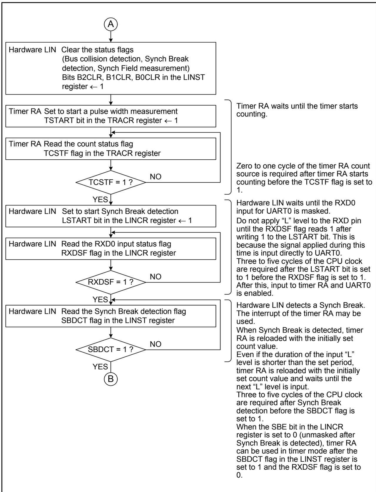
Figure 17.9 Example of Header Field Reception Flowchart (2)
