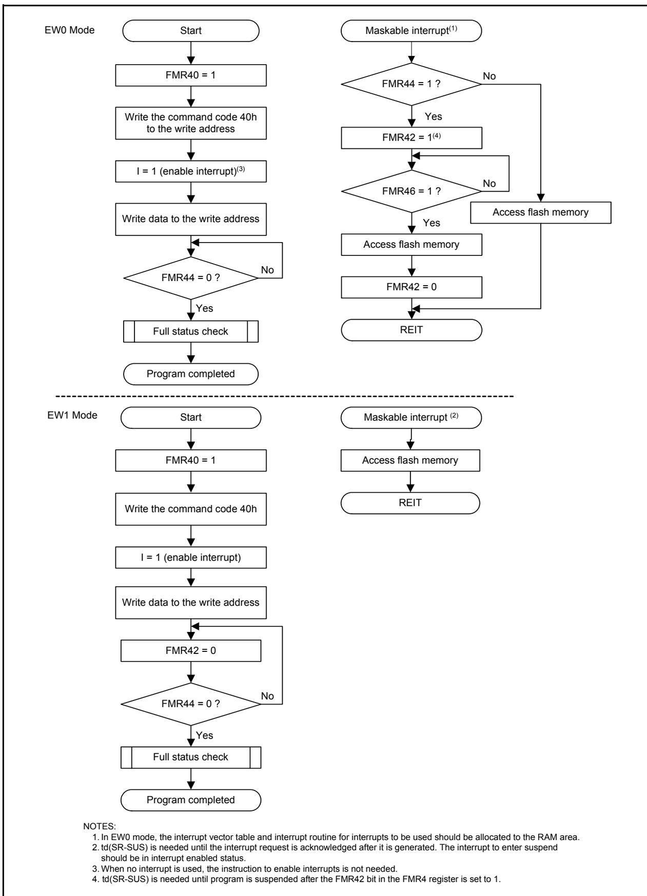
Figure 20.13 Program Command (When Suspend Function Enabled)
