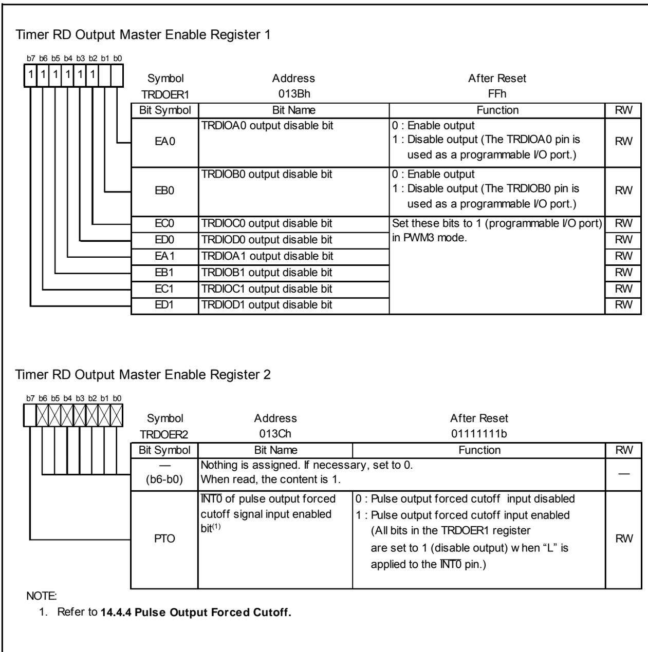
Figure 14.143 Registers TRDOER1 to TRDOER2 in PWM3 Mode
