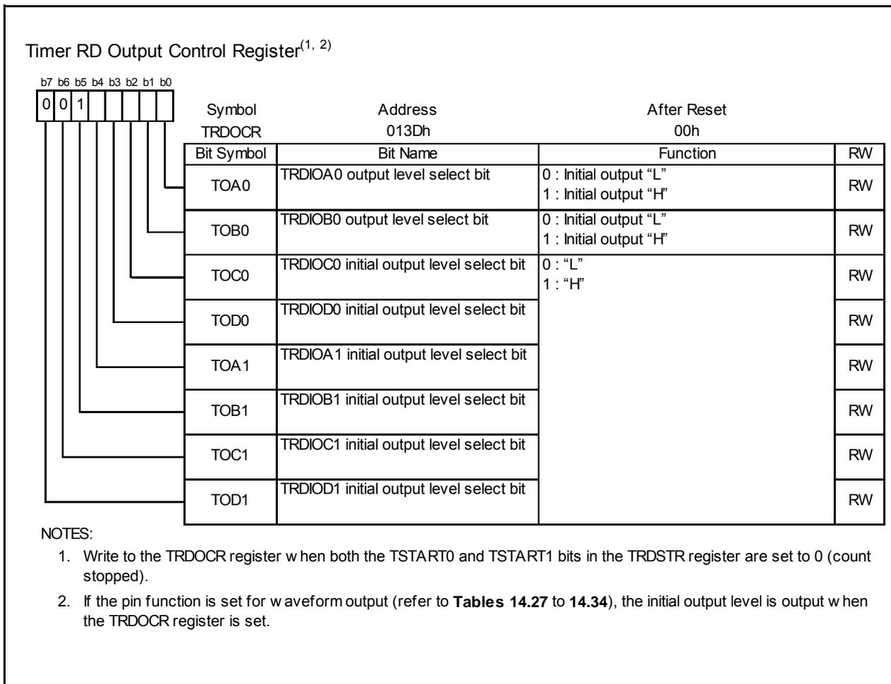
Figure 14.89 TRDOCR Register in Output Compare Function
