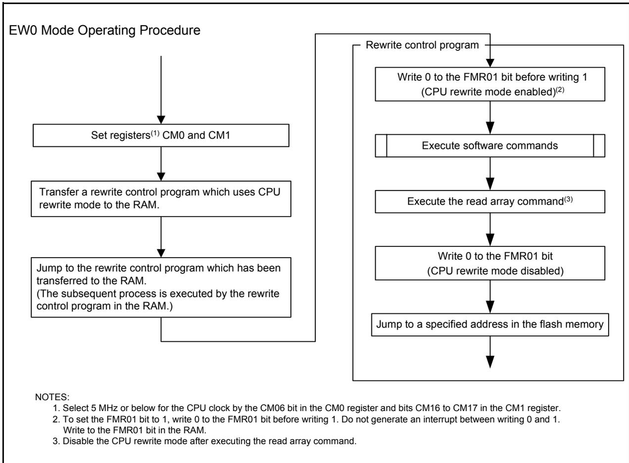
**Figure 20.9 How to Set and Exit EW0 Mode**
