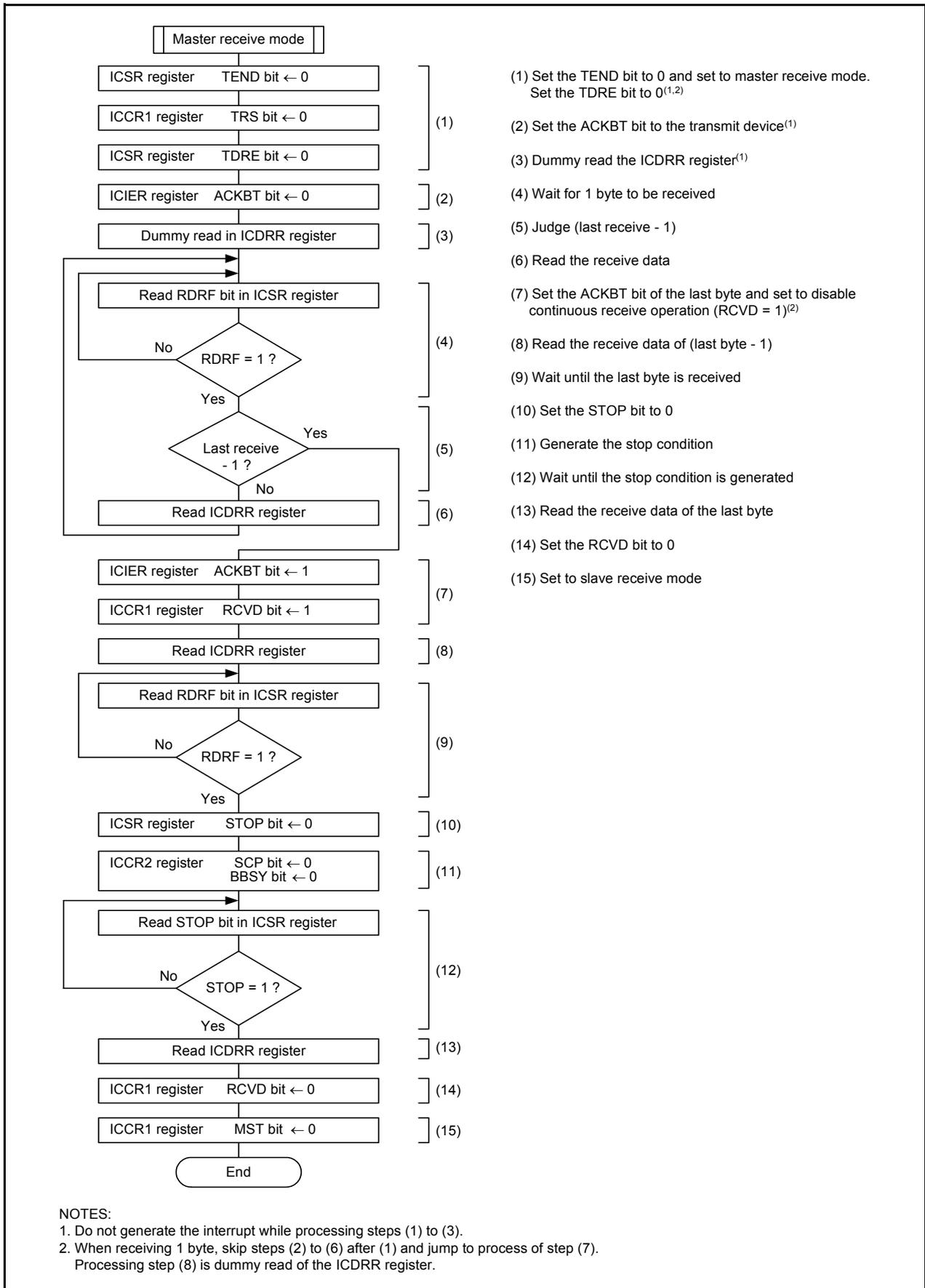
Figure 16.47 Example of Register Setting in Master Receive Mode (I<sup>2</sup>C bus Interface Mode)
