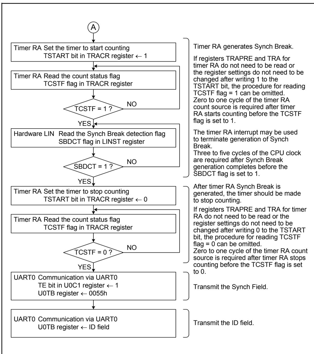
Figure 17.6 Example of Header Field Transmission Flowchart (2)
