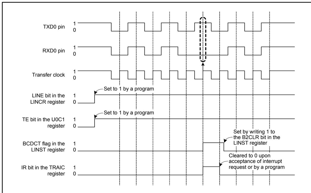
Figure 17.11 Typical Operation when a Bus Collision is Detected
