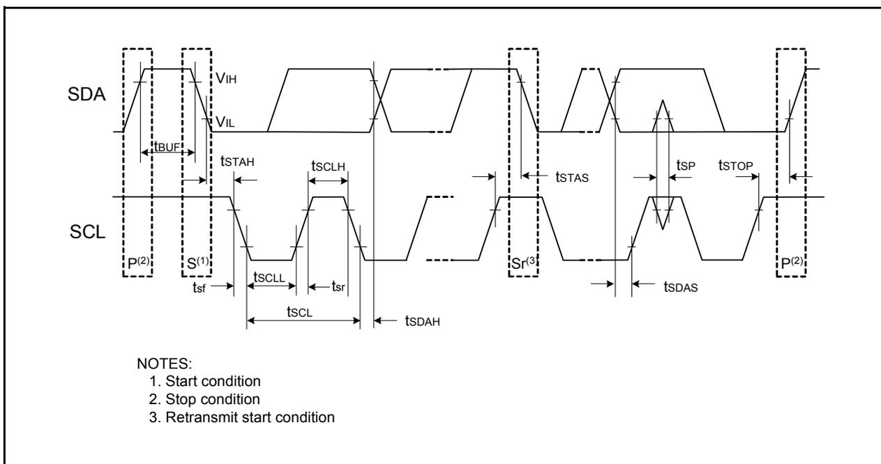
**Figure 21.7 I/O Timing of I<sup>2</sup>C bus Interface**
