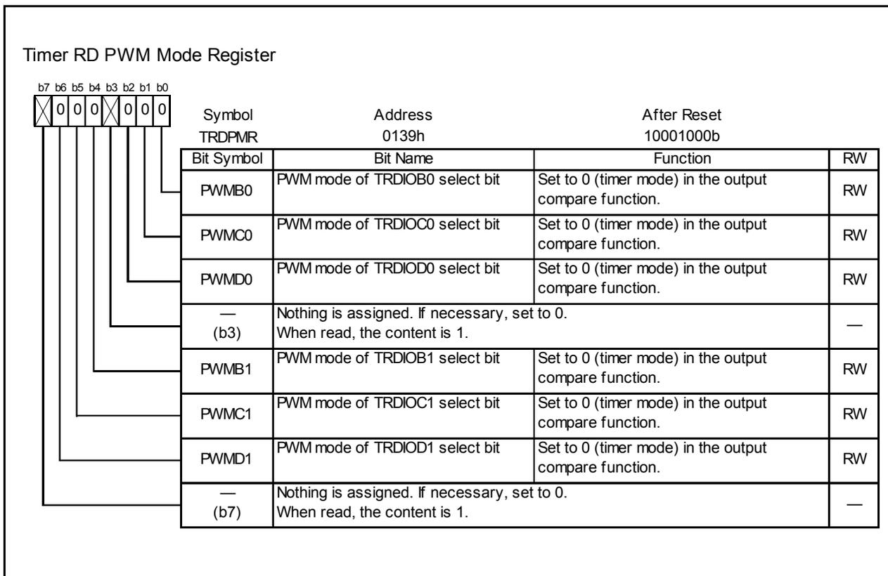
Figure 14.86 TRDPMR Register in Output Compare Function
