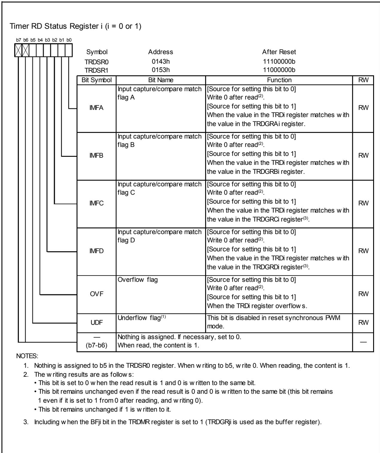
Figure 14.120 Registers TRDSR0 to TRDSR1 in Reset Synchronous PWM Mode
