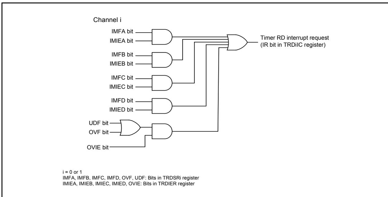
**Figure 14.151 Block Diagram of Timer RD Interrupt**
