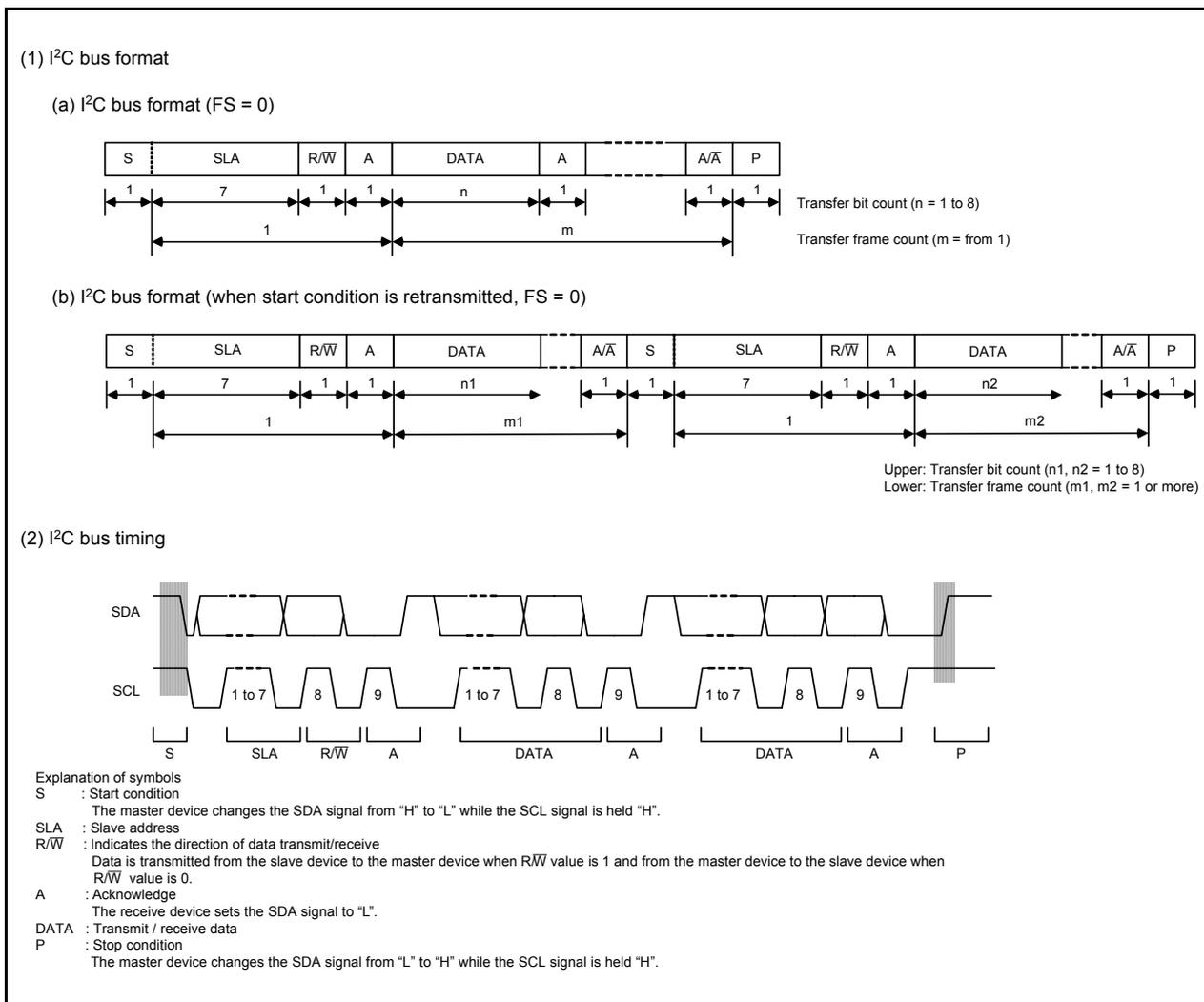
Figure 16.34 I<sup>2</sup>C bus Format and Bus Timing
