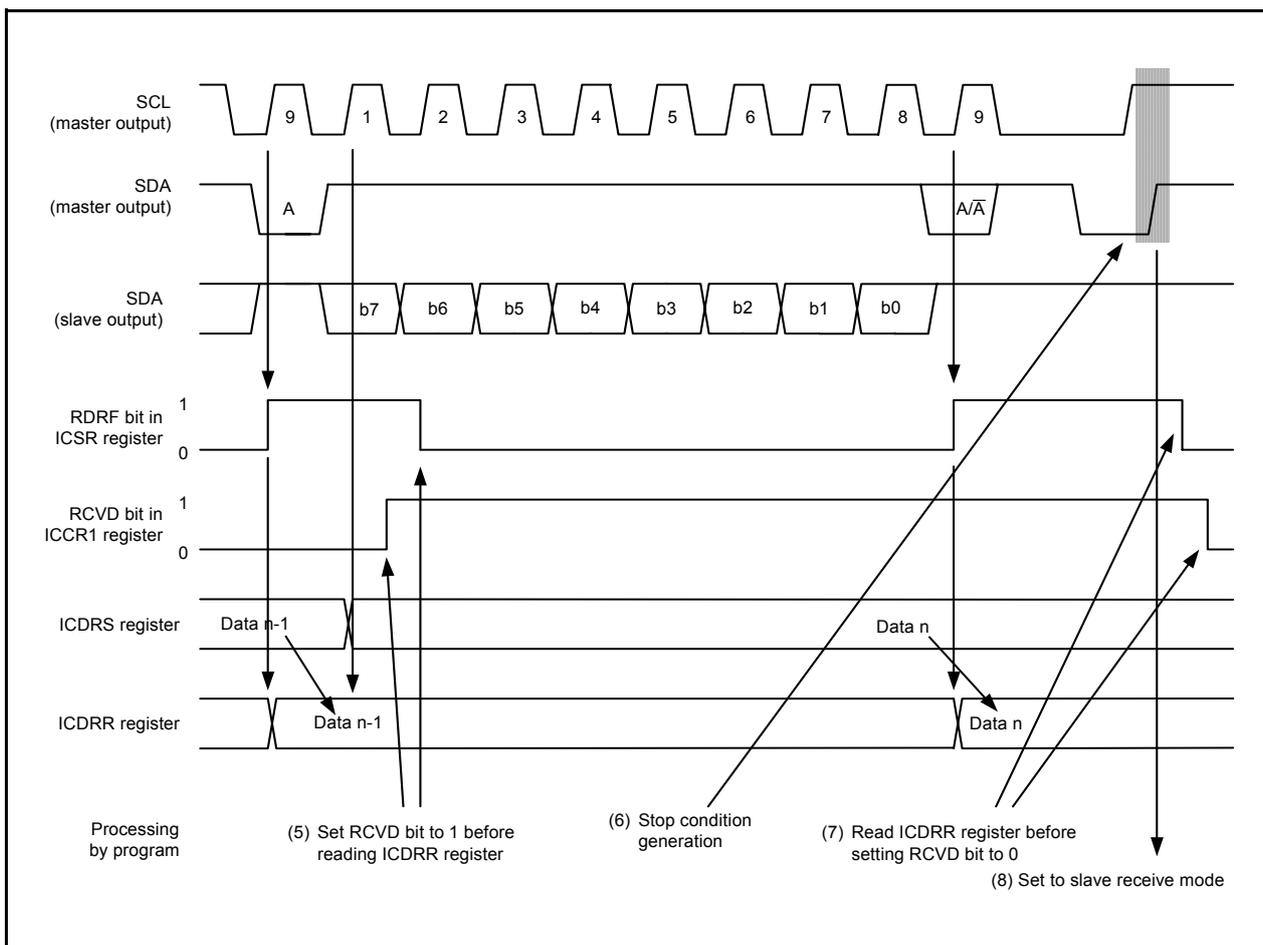
Figure 16.38 Operating Timing in Master Receive Mode (I<sup>2</sup>C bus Interface Mode) (2)
