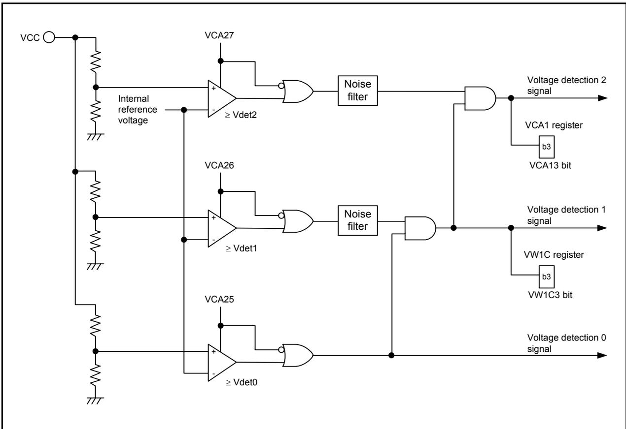
Figure 6.1 Block Diagram of Voltage Detection Circuit
