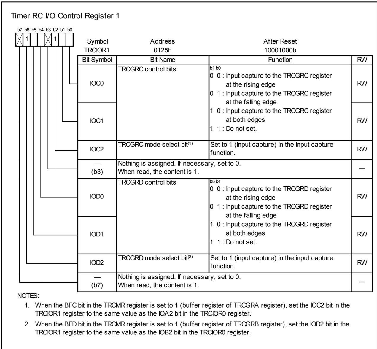
Figure 14.45 TRCIOR1 Register for Input Capture Function
