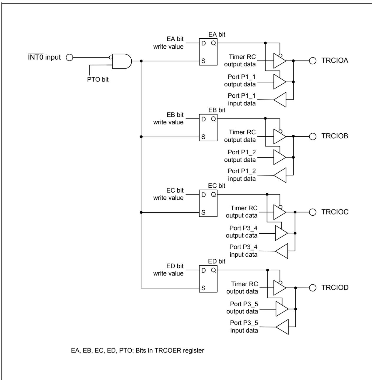
Figure 14.42 Forced Cutoff of Pulse Output
