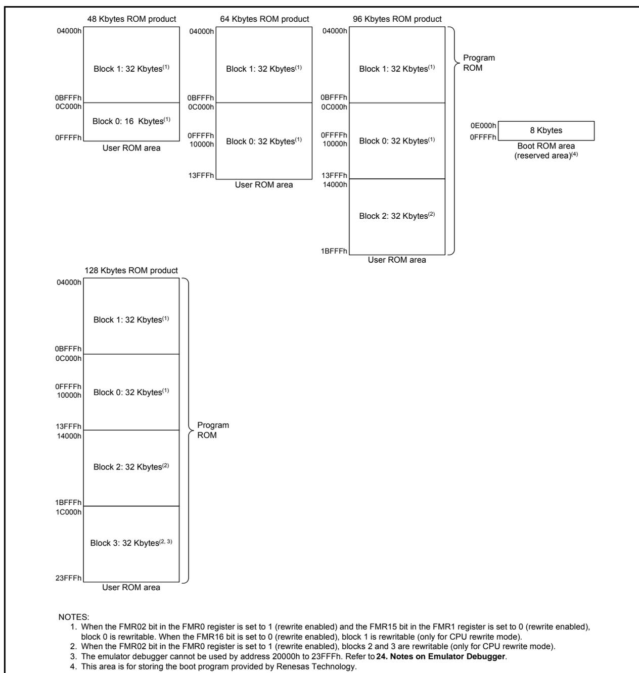
Figure 20.1 Flash Memory Block Diagram for R8C/2A Group
