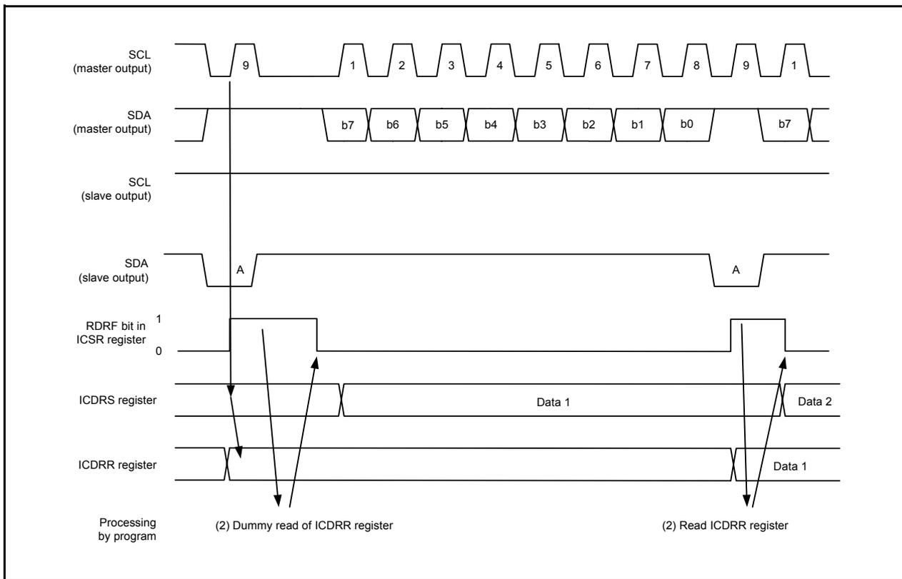
Figure 16.41 Operating Timing in Slave Receive Mode (I<sup>2</sup>C bus Interface Mode) (1)
