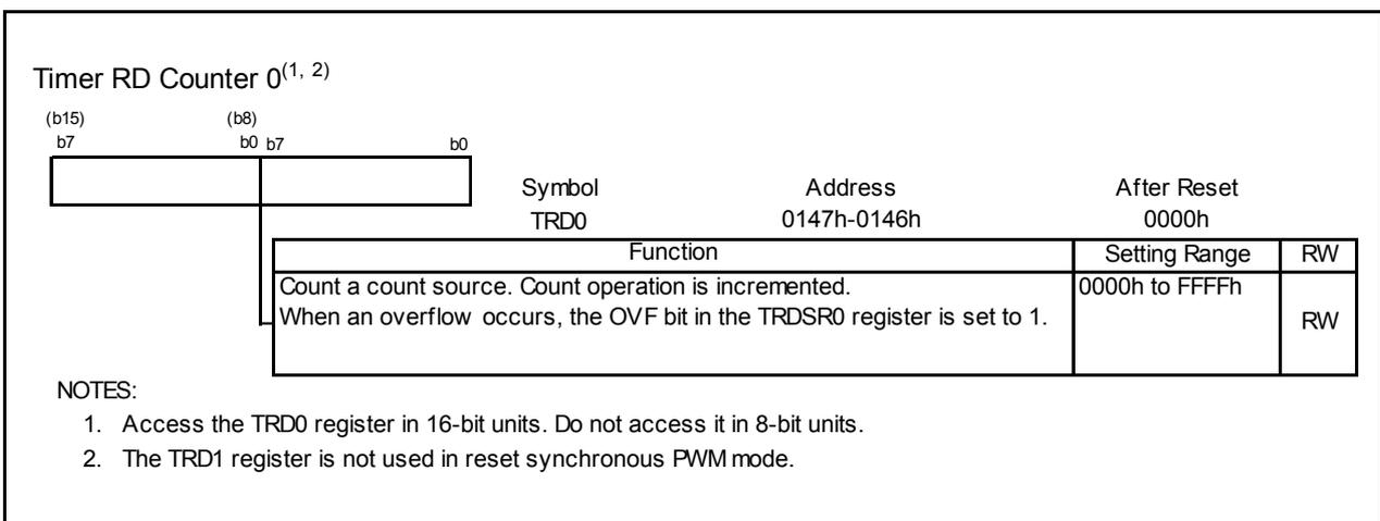
Figure 14.122 TRD0 Registrar in Reset Synchronous PWM Mode
