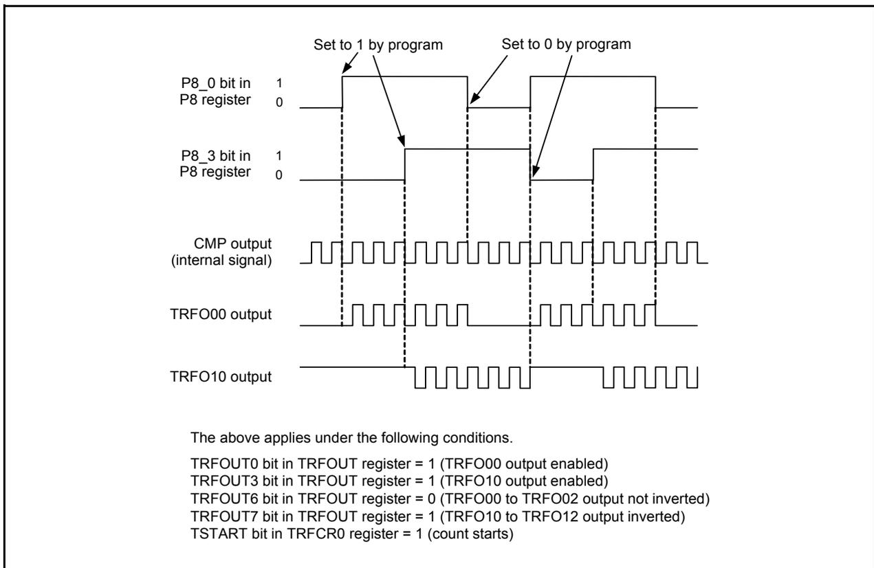
**Figure 14.184 Operating Example in Output Compare Mode (“L” and “H” Held Output in Count Stops)**
