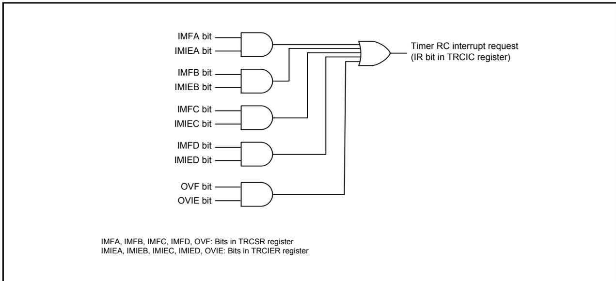
**Figure 14.61 Timer RC Interrupt Block Diagram**
