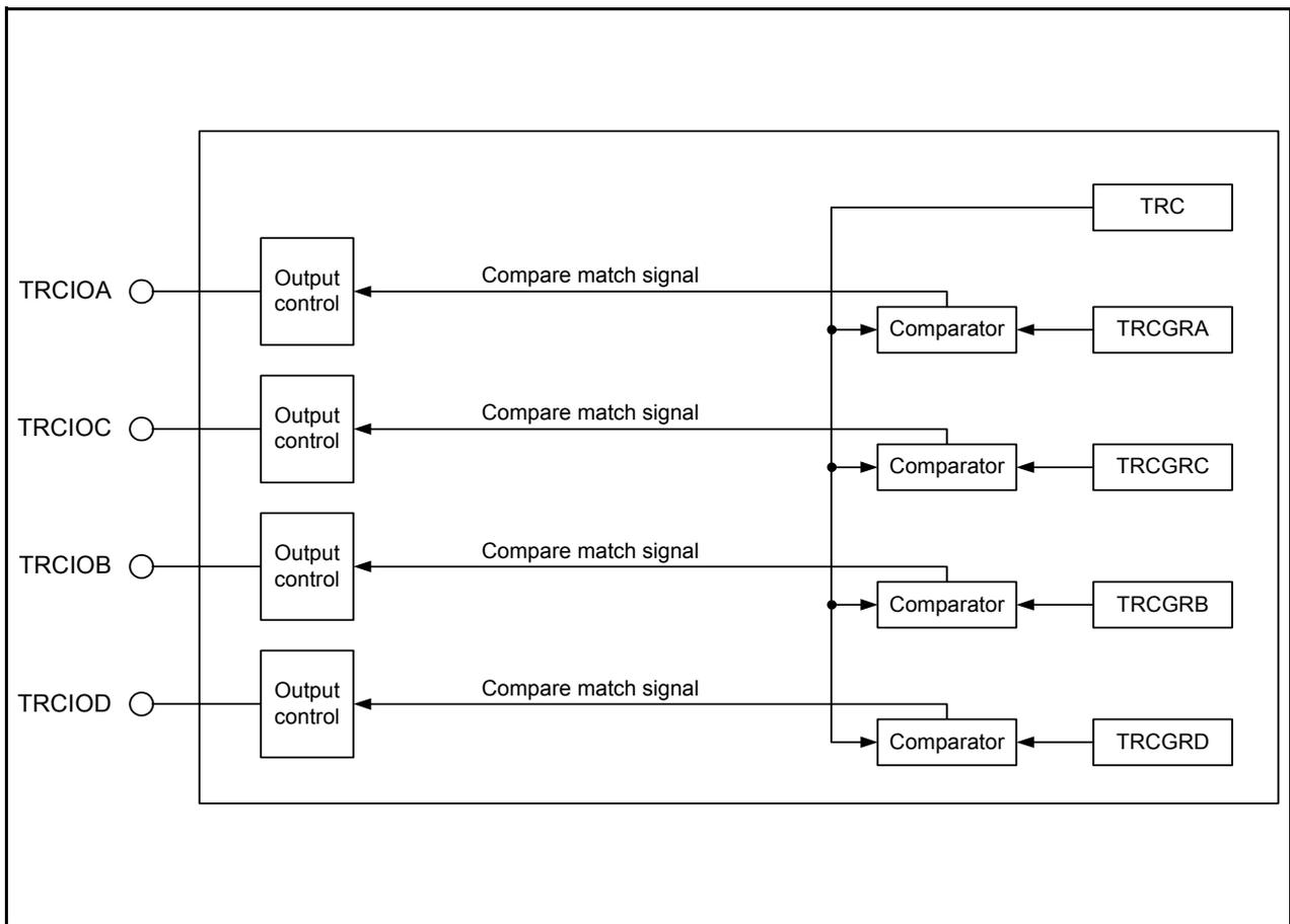
Figure 14.47 Block Diagram of Output Compare Function
