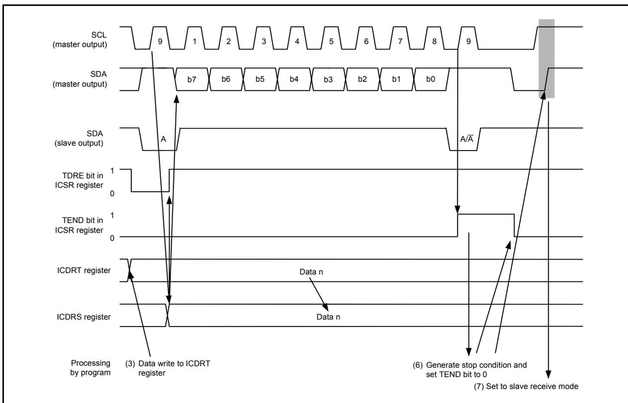
Figure 16.36 Operating Timing in Master Transmit Mode (I<sup>2</sup>C bus Interface Mode) (2)
