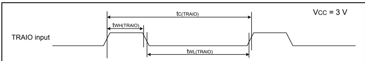
**Figure 21.14 TRAIO Input and  $\overline{\text{INT1}}$  Input Timing Diagram when  $V_{CC} = 3\text{ V}$** **Table 21.27 TRFI Input**
