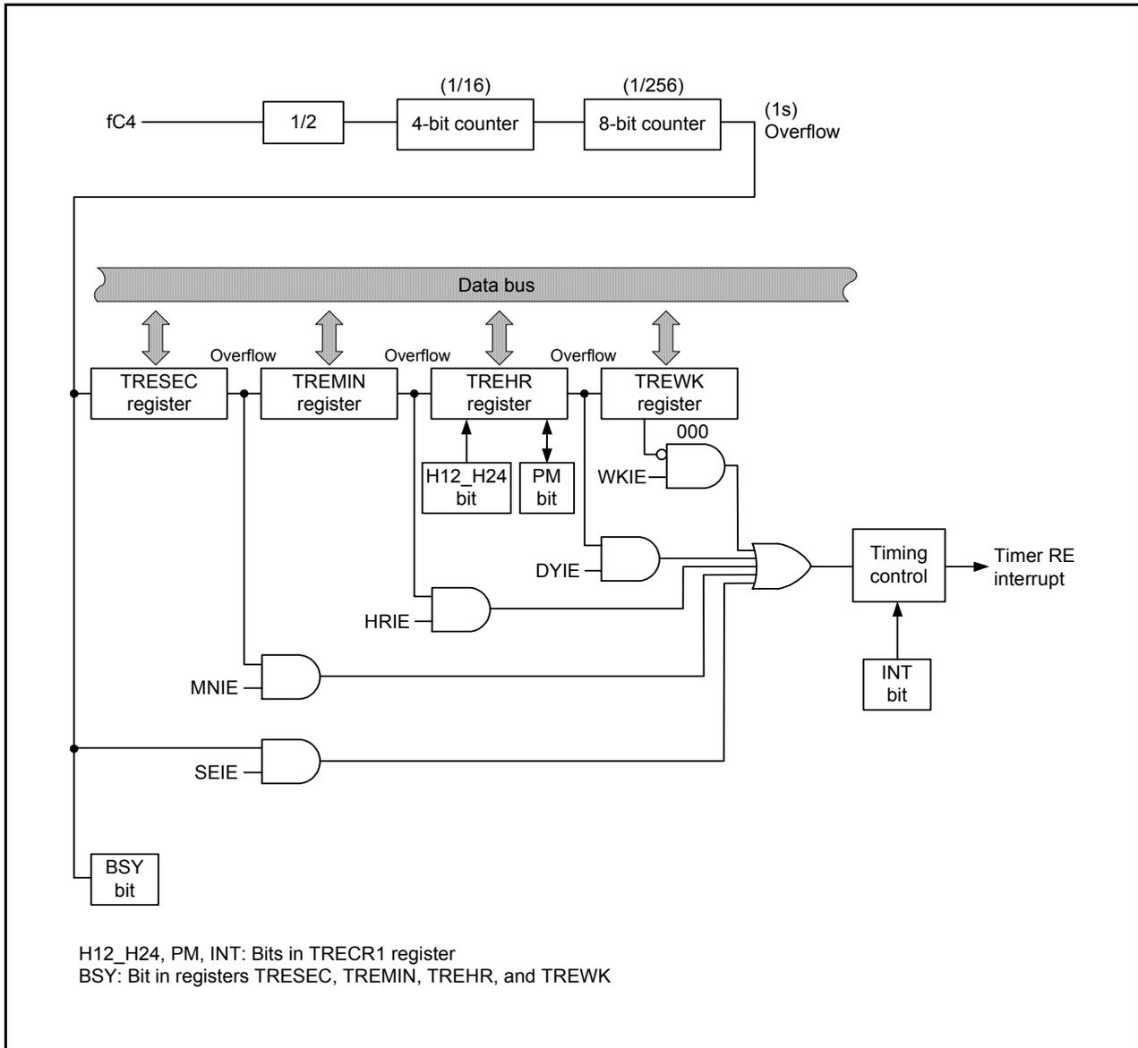
Figure 14.156 Block Diagram of Real-Time Clock Mode
