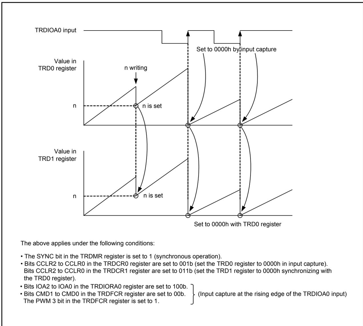
Figure 14.66 Synchronous Operation
