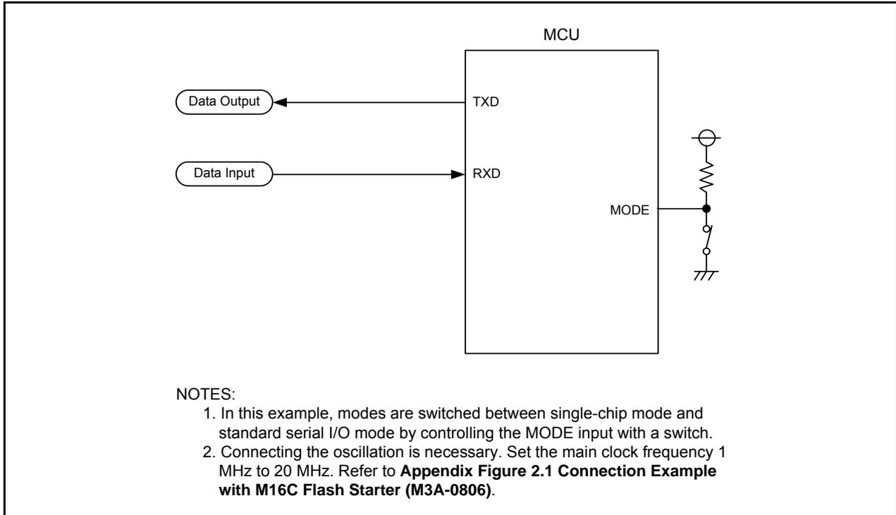
**Figure 20.18 Pin Processing in Standard Serial I/O Mode 2**
