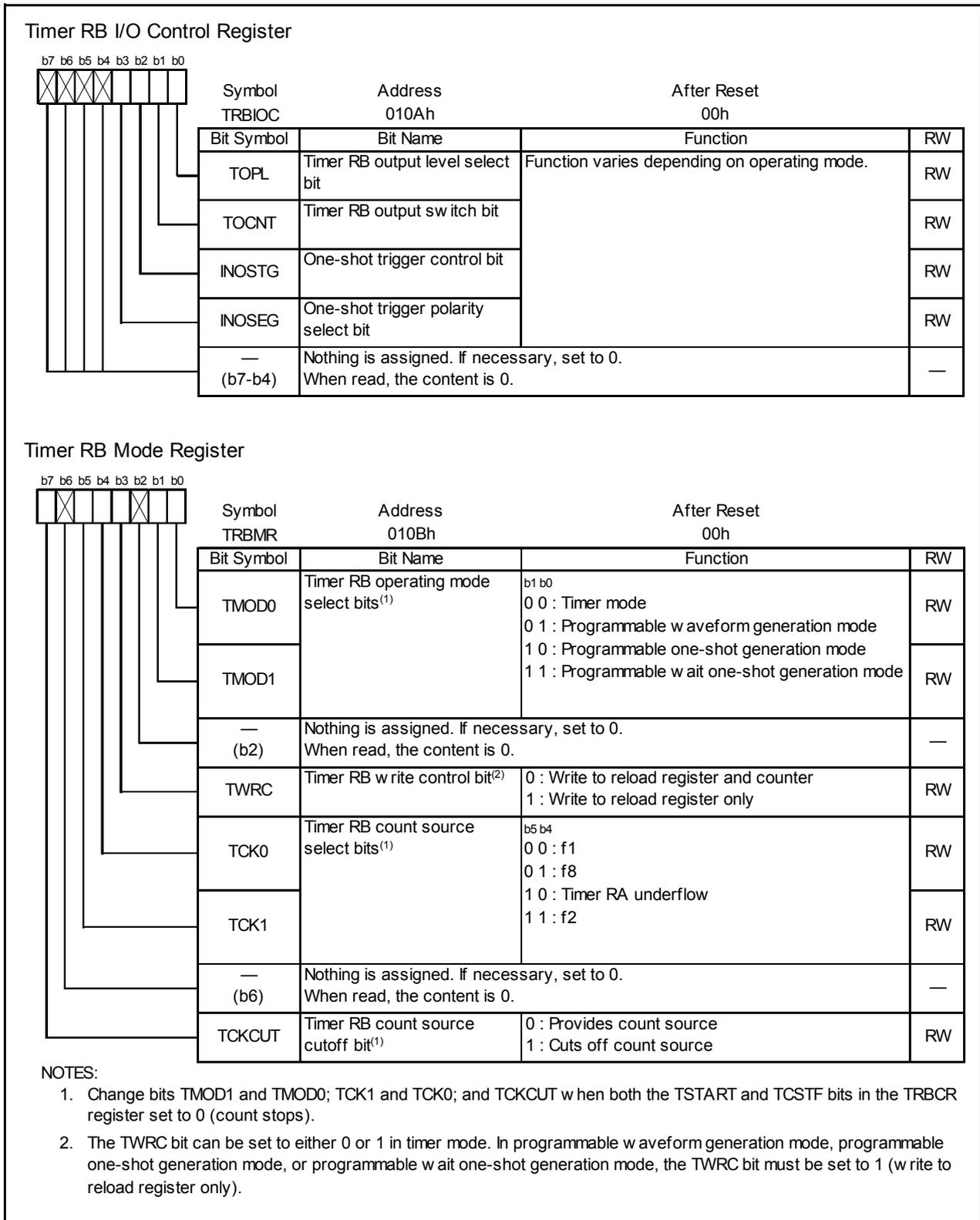
Figure 14.14 Registers TRBIOC and TRBMR
