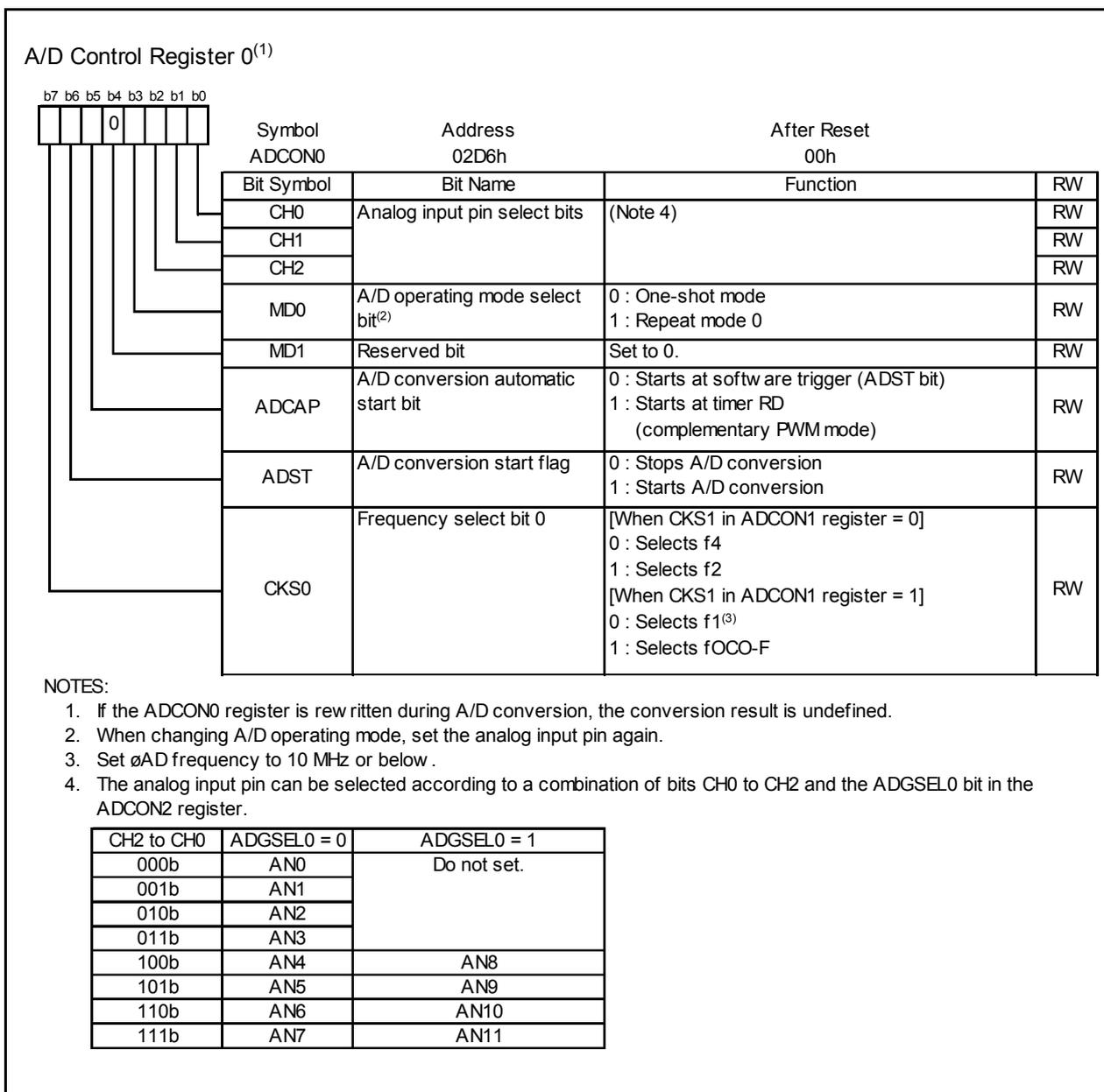
Figure 18.3 ADCON0 Register
