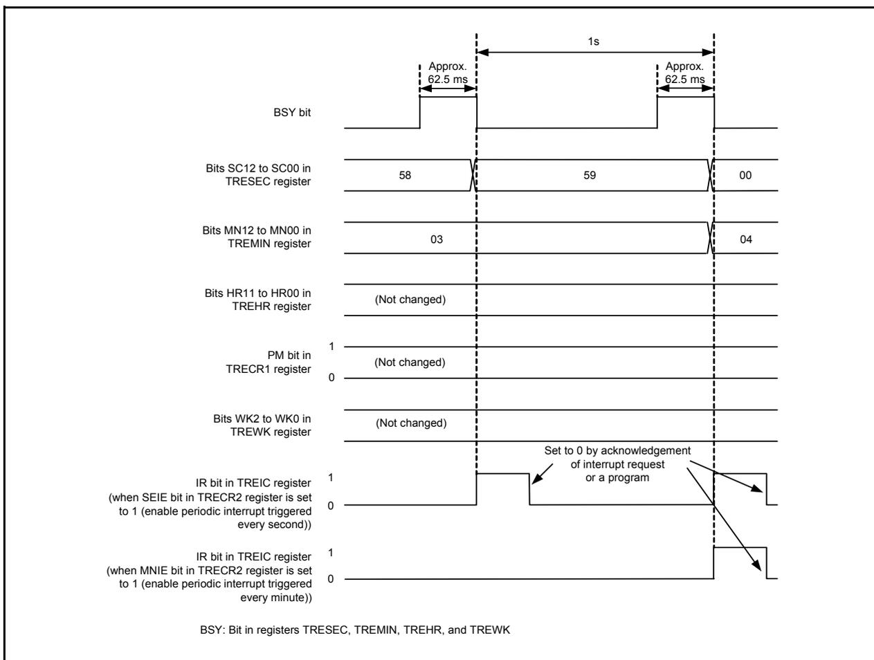
Figure 14.165 Operating Example in Real-Time Clock Mode
