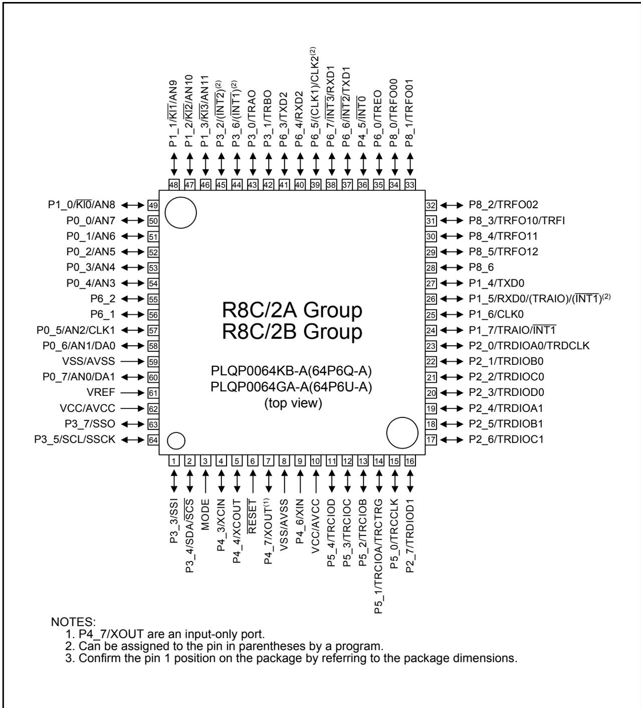
Figure 1.4 64-pin LQFP Package Pin Assignment (Top View)
