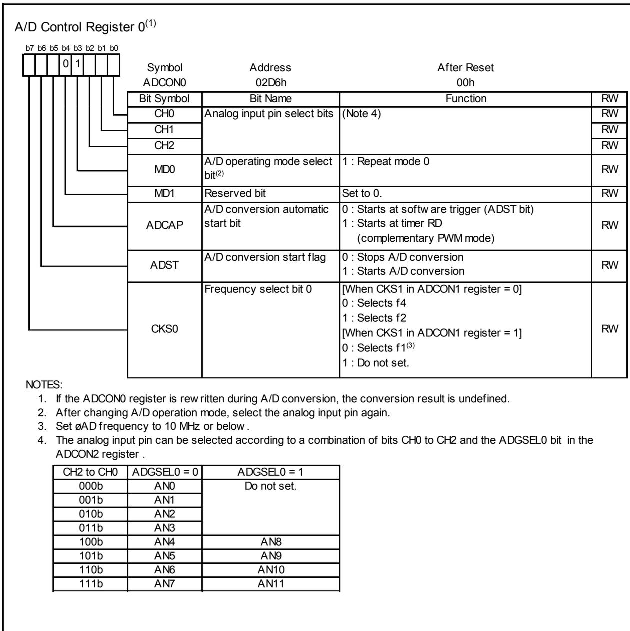
**Figure 18.7 ADCON0 Register in Repeat Mode 0**
