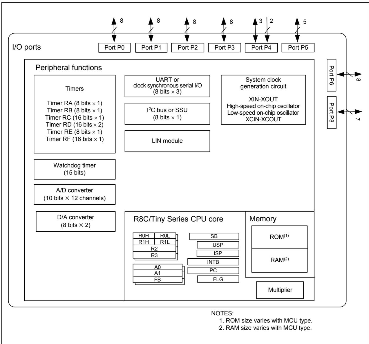
Figure 1.3 Block Diagram
