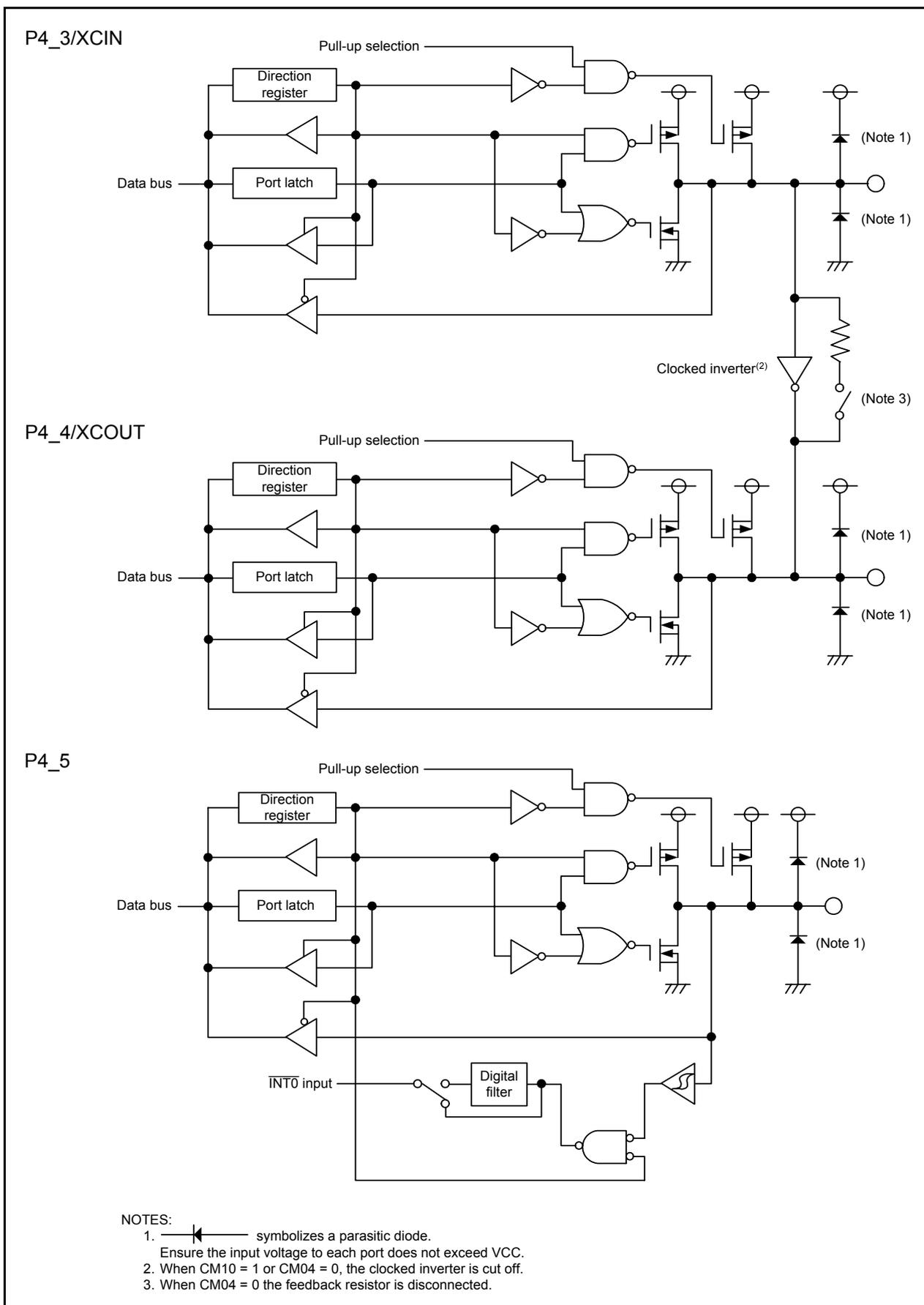
Figure 7.5 Configuration of Programmable I/O Ports (5)
