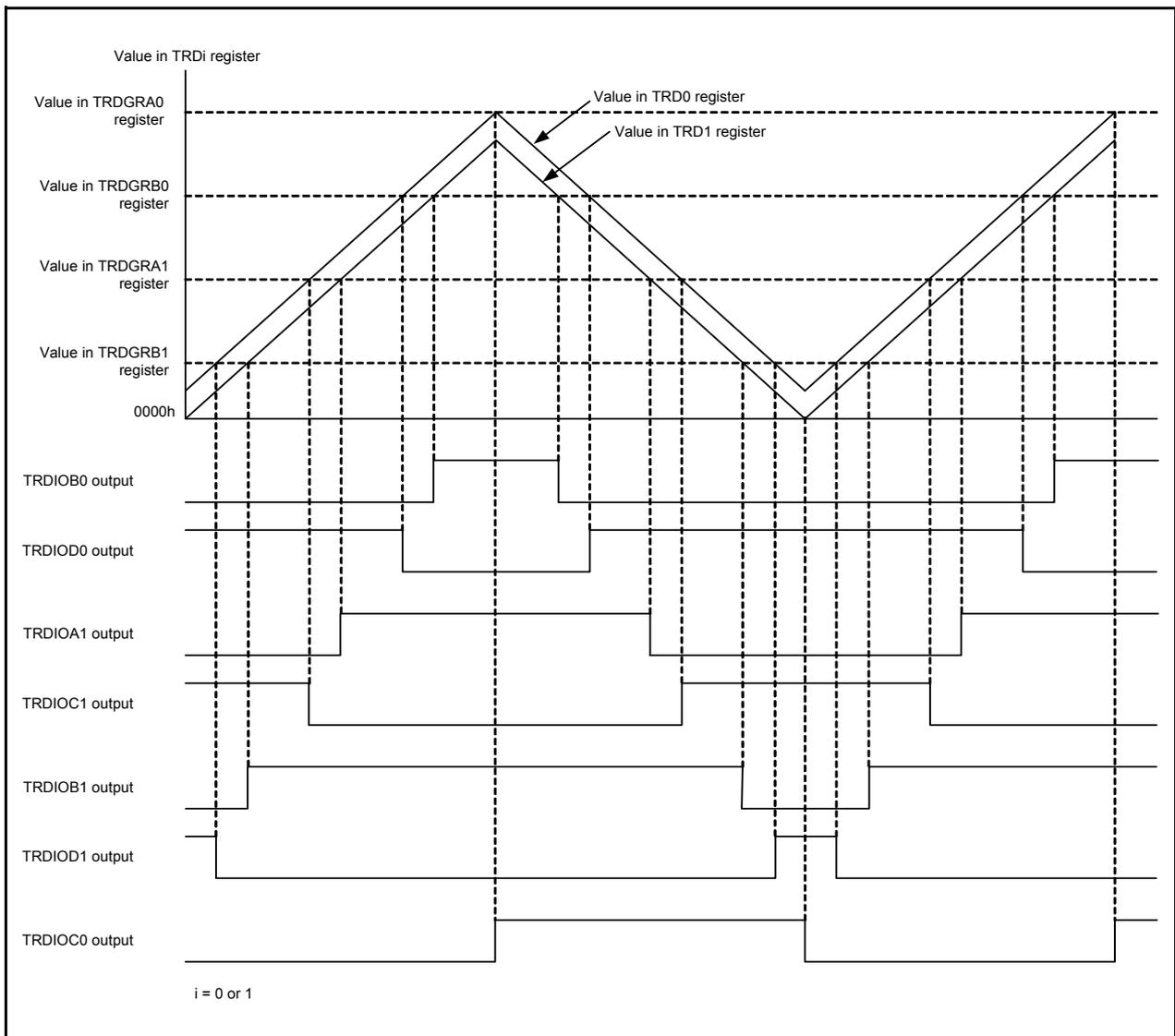
Figure 14.136 Output Model of Complementary PWM Mode
