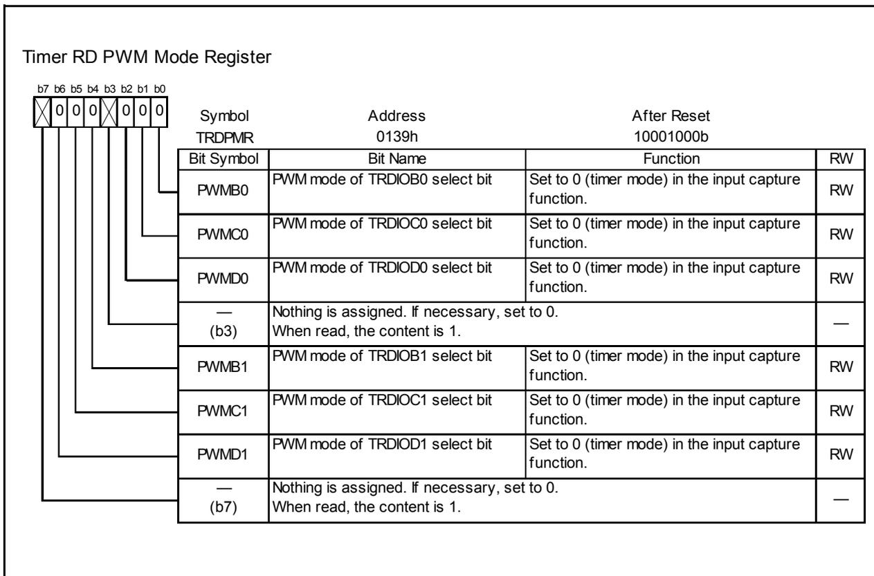
Figure 14.71 TRDPMR Register in Input Capture Function
