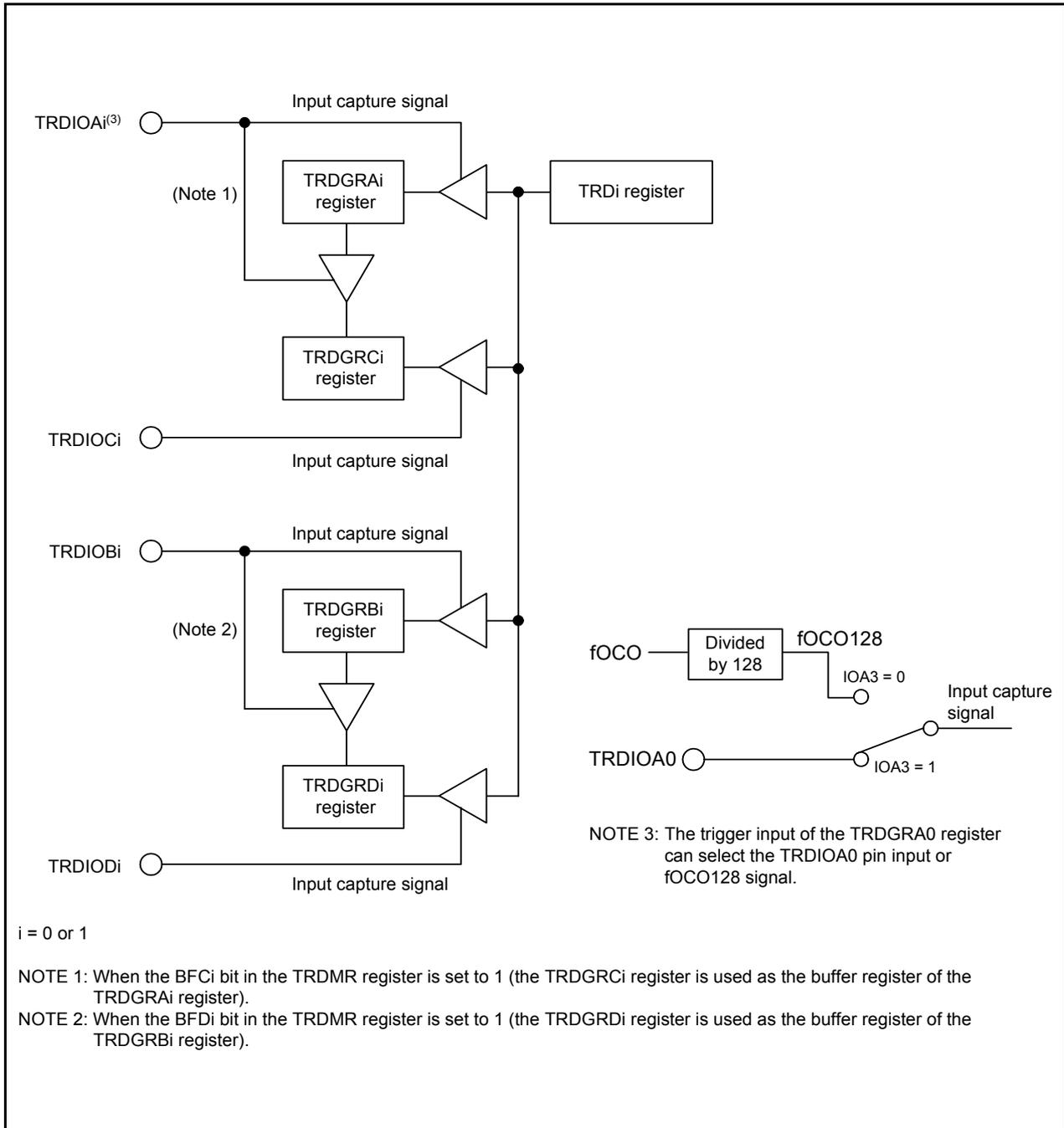
Figure 14.68 Block Diagram of Input Capture Function
