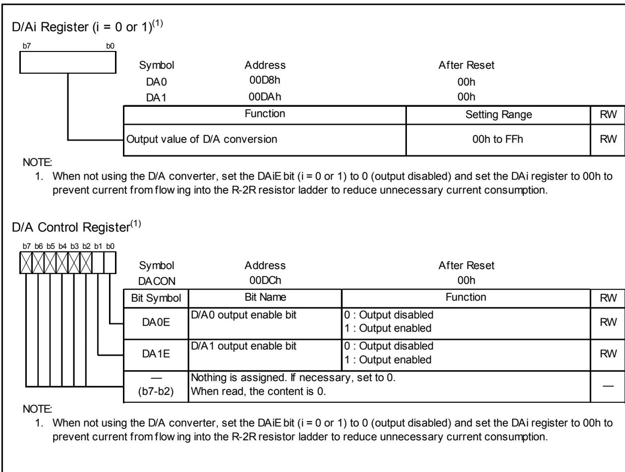
Figure 19.2 Registers DA0 to DA1 and DACON
