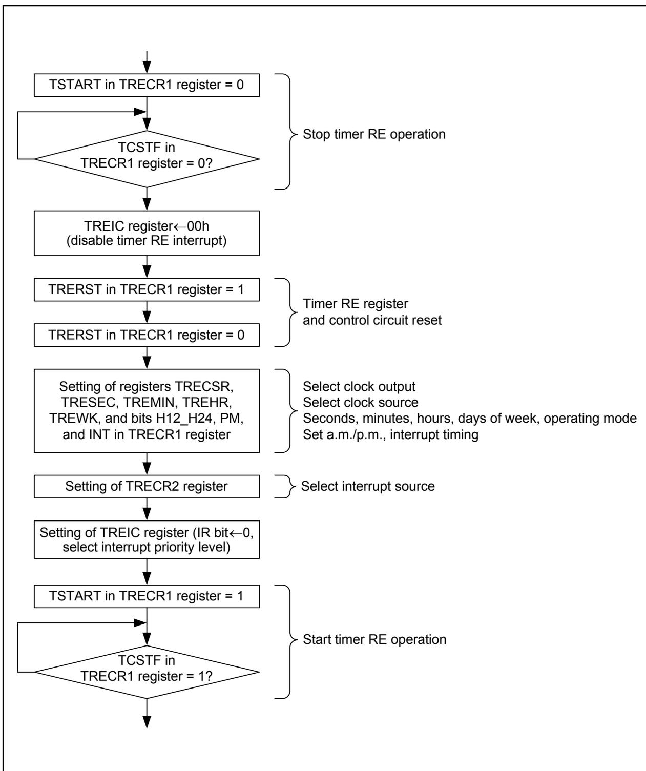
Figure 22.8 Setting Example in Real-Time Clock Mode
