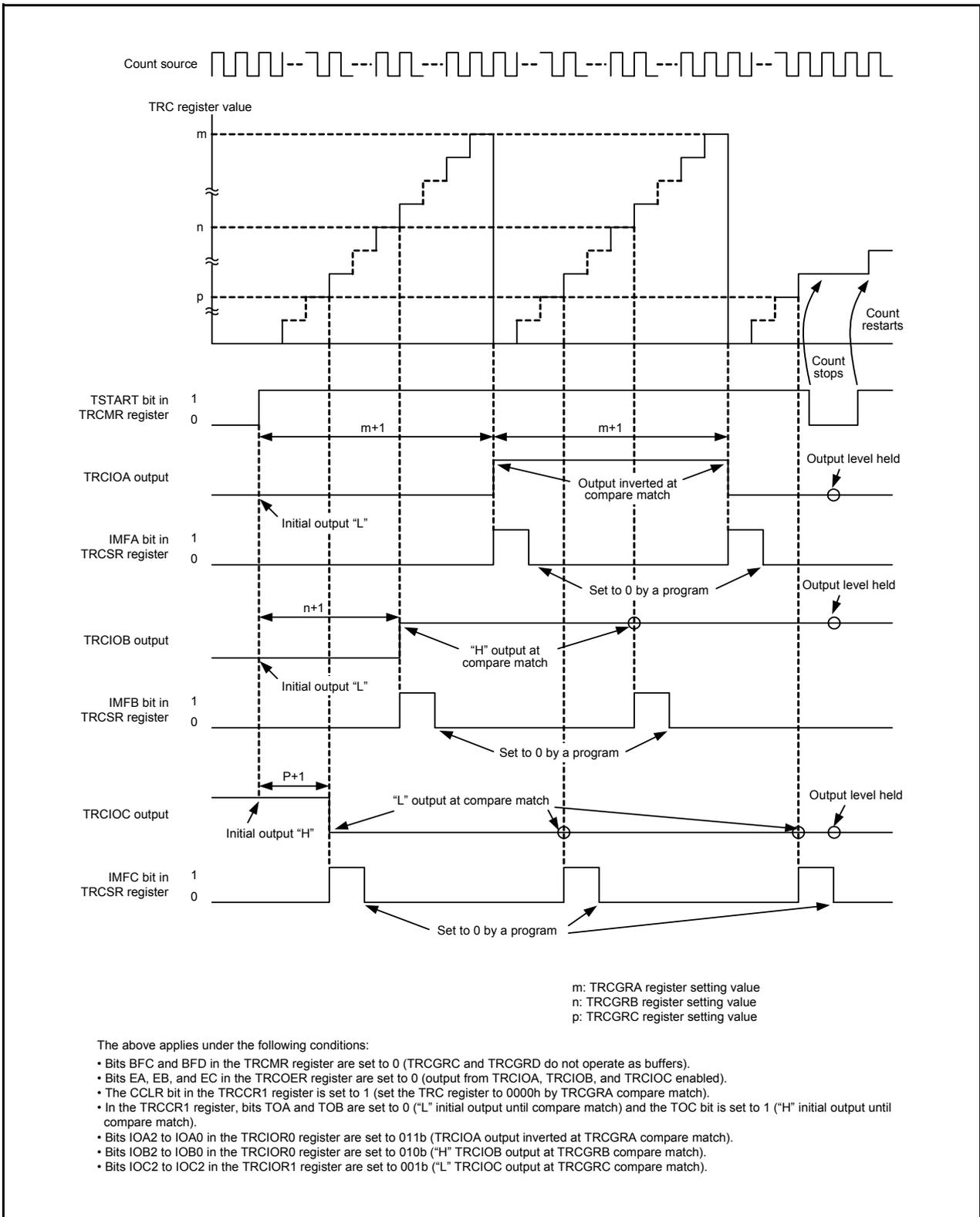
Figure 14.51 Operating Example of Output Compare Function
