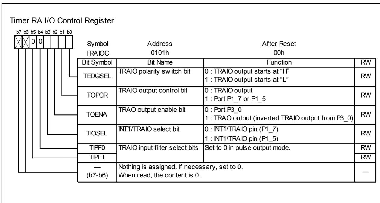
Figure 14.6 TRATIO Register in Pulse Output Mode
