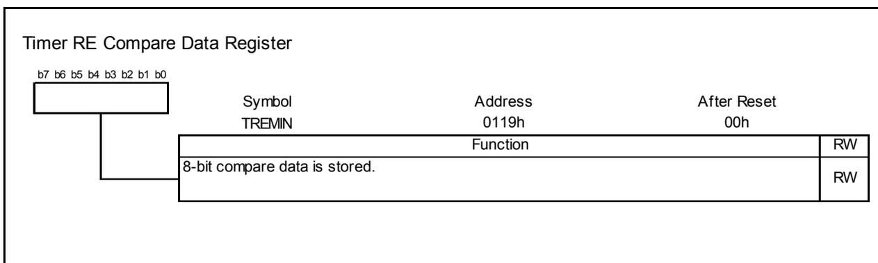
Figure 14.168 TREMIN Register in Output Compare Mode
