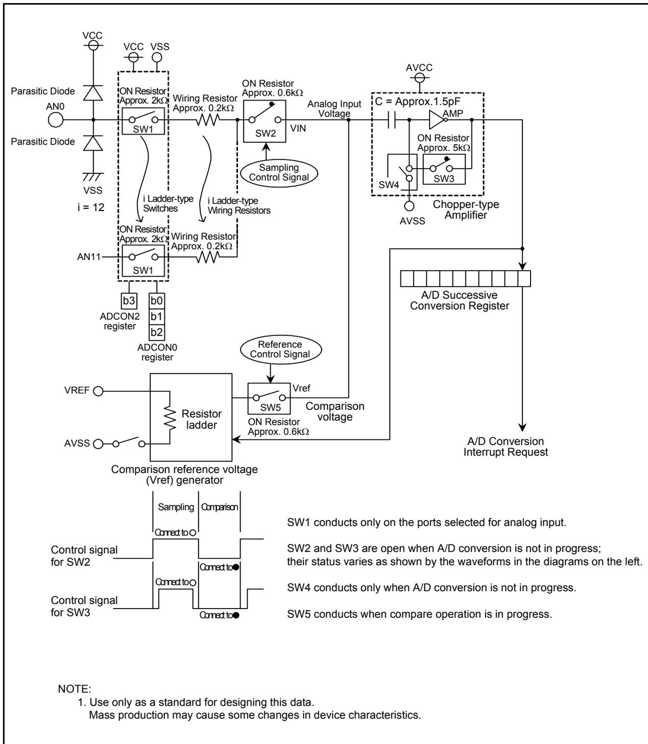
Figure 18.11 Internal Equivalent Circuit of Analog Input
