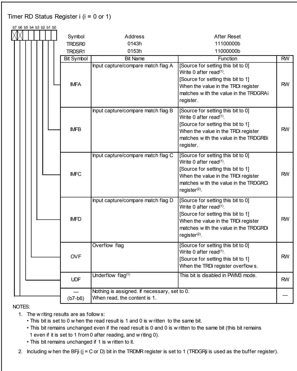
Figure 14.146 Registers TRDSR0 to TRDSR1 in PWM3 Mode
