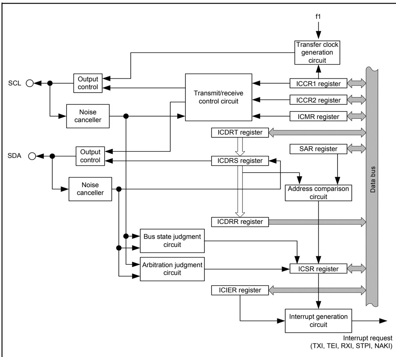
Figure 16.23 Block Diagram of I<sup>2</sup>C bus interface
