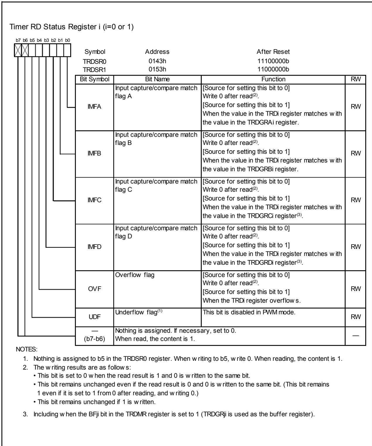
Figure 14.107 Registers TRDSR0 to TRDSR1 in PWM Mode
