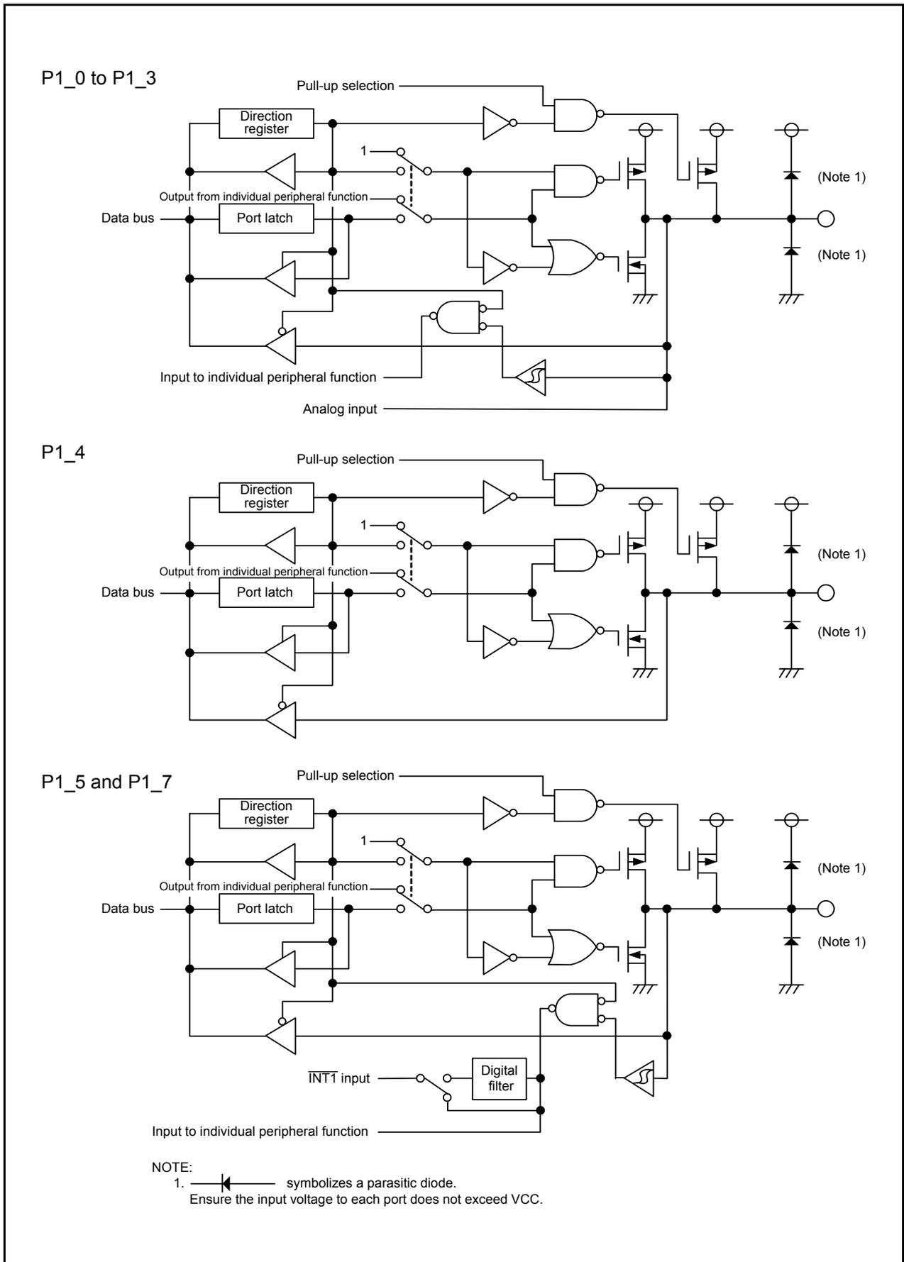
Figure 7.2 Configuration of Programmable I/O Ports (2)
