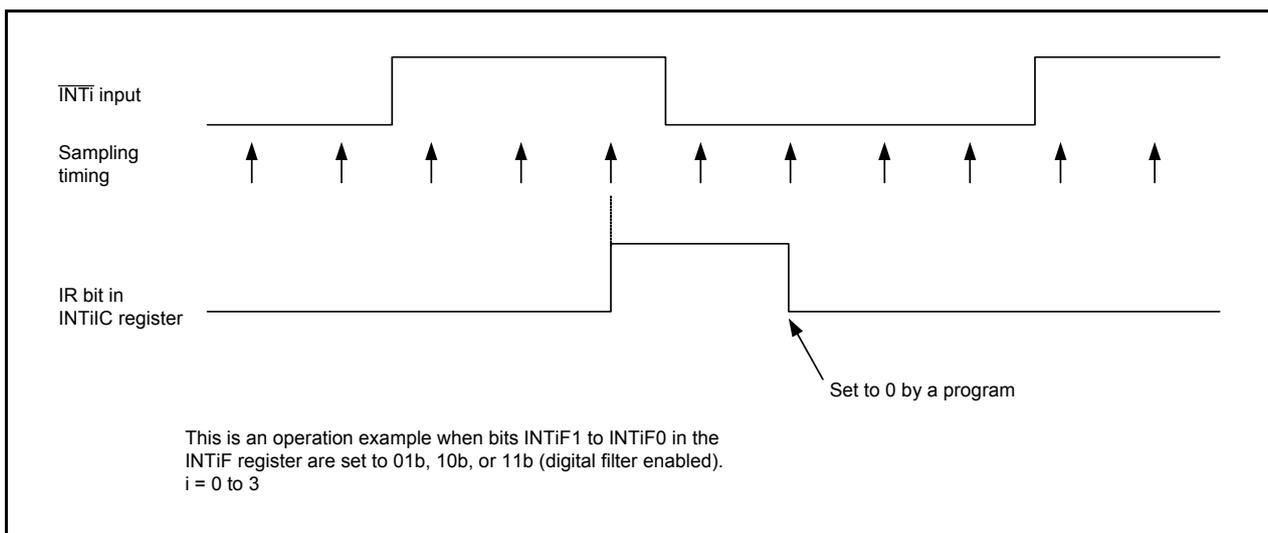
Figure 12.17 Operating Example of  $\overline{\text{INT}}_i$  Input Filter
