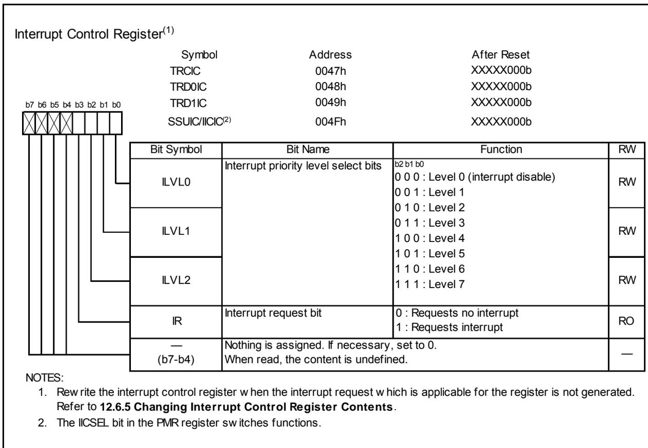
Figure 12.4 Registers TRCIC, TRD0IC, TRD1IC, SSUIC, and IICIC
