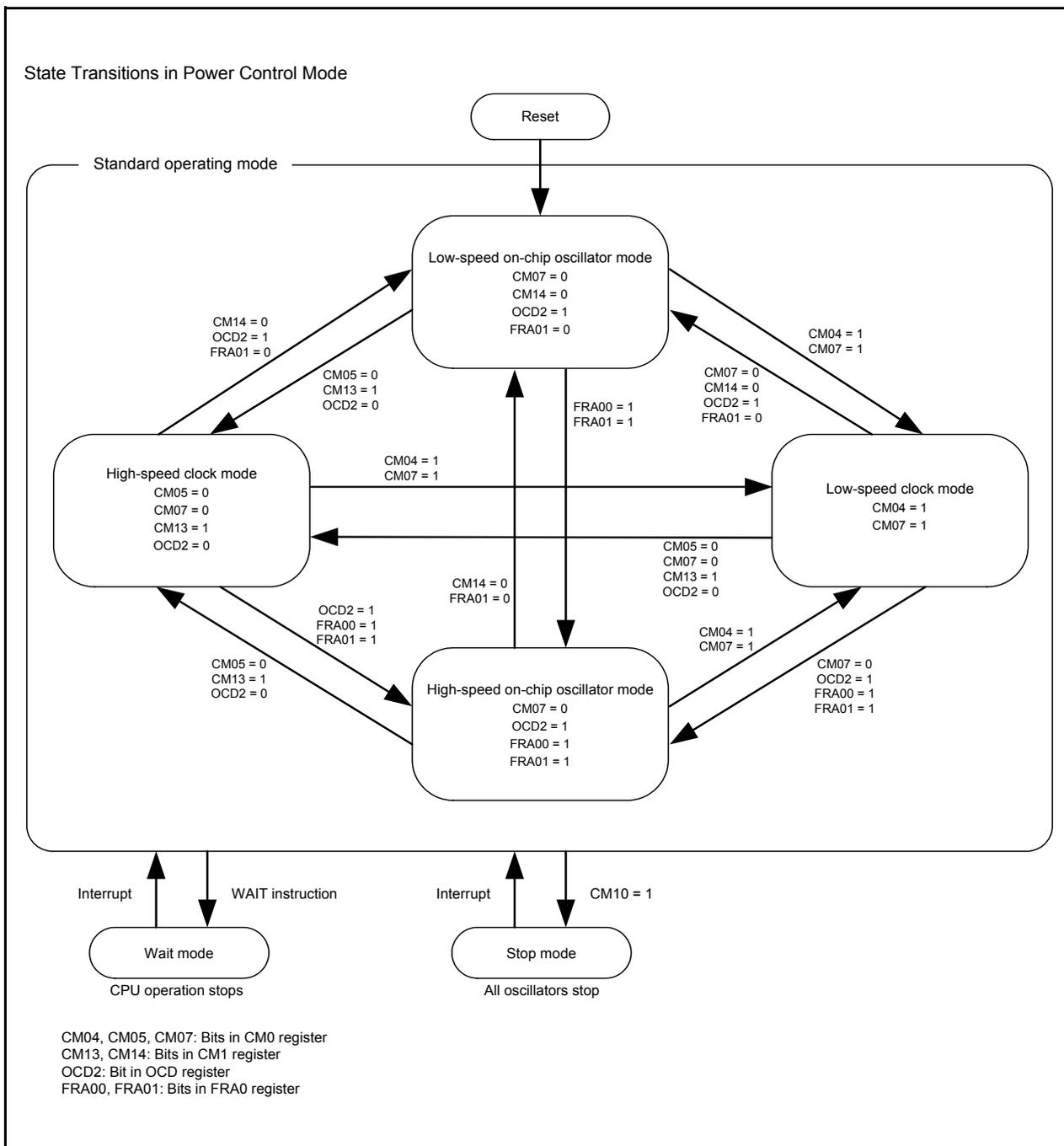
Figure 10.16 State Transitions in Power Control Mode
