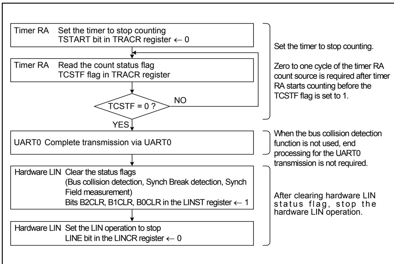
Figure 17.12 Example of Hardware LIN Communication Completion Flowchart
