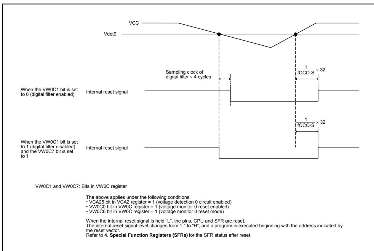
**Figure 6.9 Example of Voltage Monitor 0 Reset Operation**
