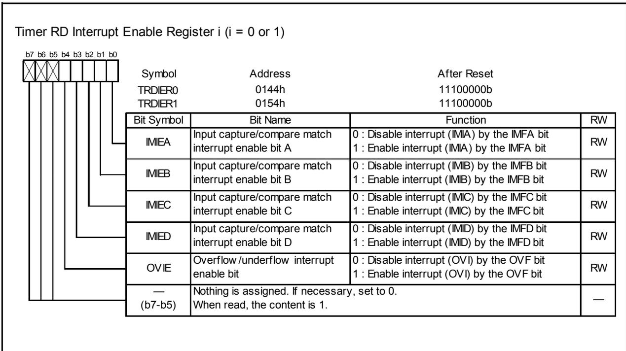
Figure 14.78 Registers TRDIER0 to TRDIER1 in Input Capture Function
