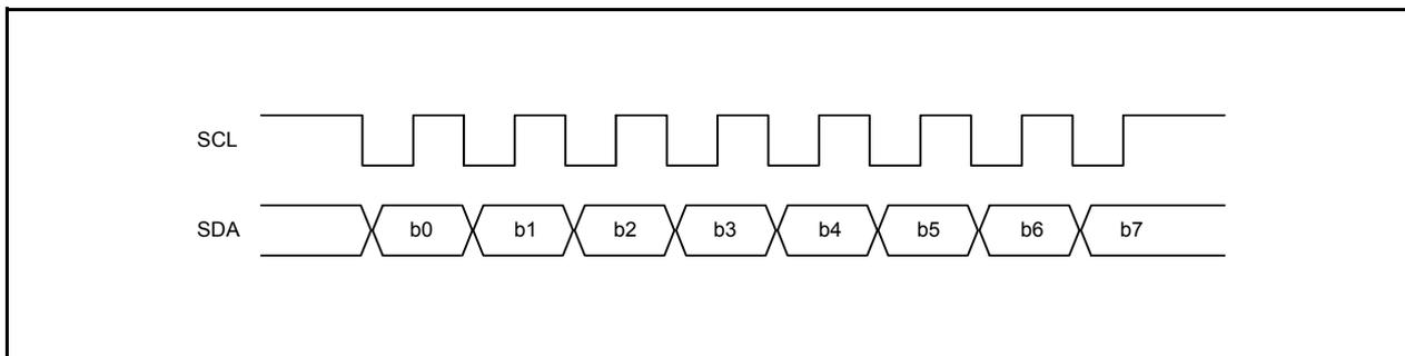
Figure 16.43 Transfer Format of Clock Synchronous Serial Format
