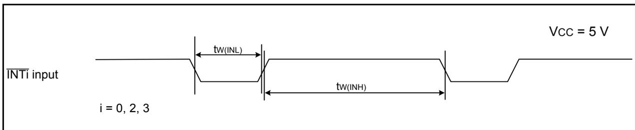
**Figure 21.12 External Interrupt  $\overline{INTi}$  Input Timing Diagram when Vcc = 5 V**
