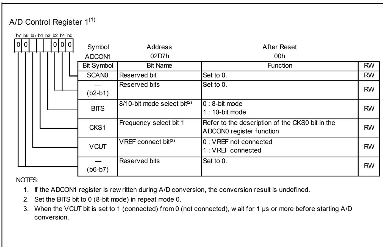
Figure 18.4 ADCON1 Register
