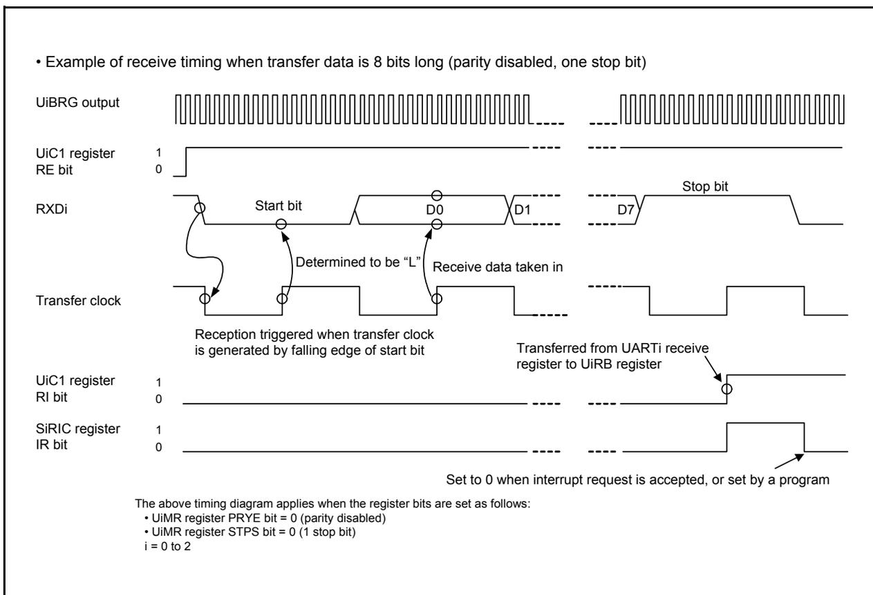
Figure 15.13 Receive Timing Example in UART Mode
