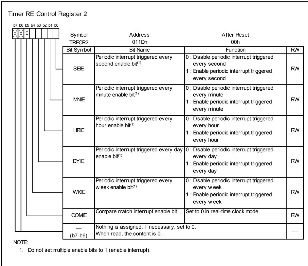
Figure 14.163 TREC2 Register in Real-Time Clock Mode
