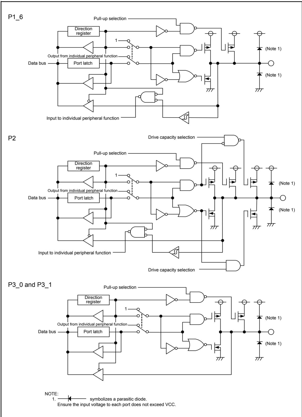
Figure 7.3 Configuration of Programmable I/O Ports (3)
