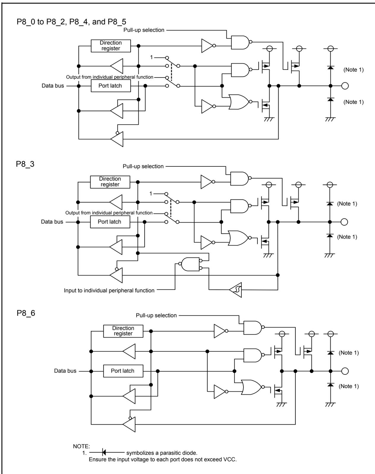
Figure 7.10 Configuration of Programmable I/O Ports (10)
