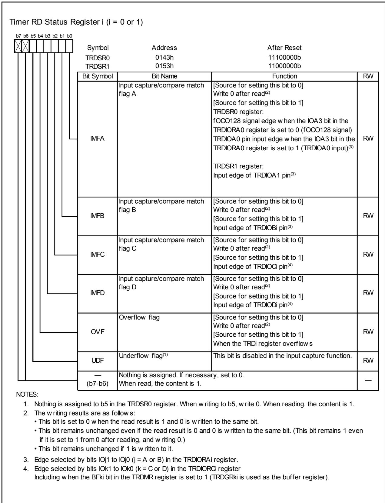
Figure 14.77 Registers TRDSR0 to TRDSR1 in Input Capture Function
