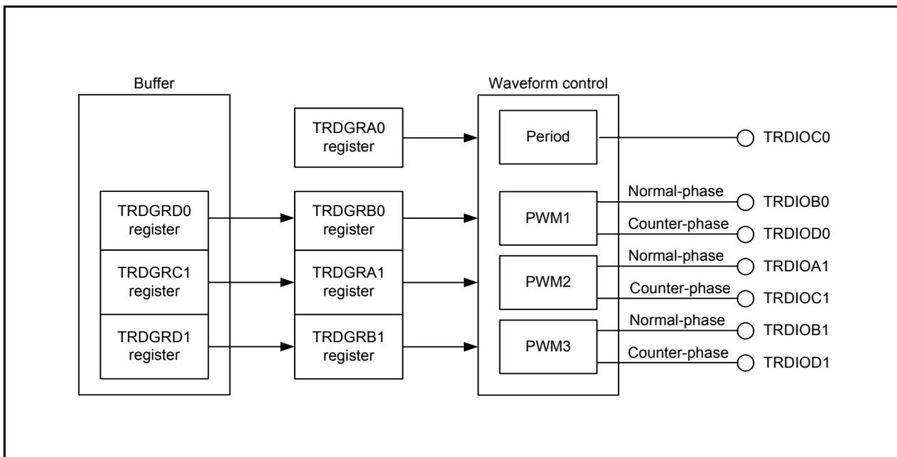
Figure 14.125 Block Diagram of Complementary PWM Mode
