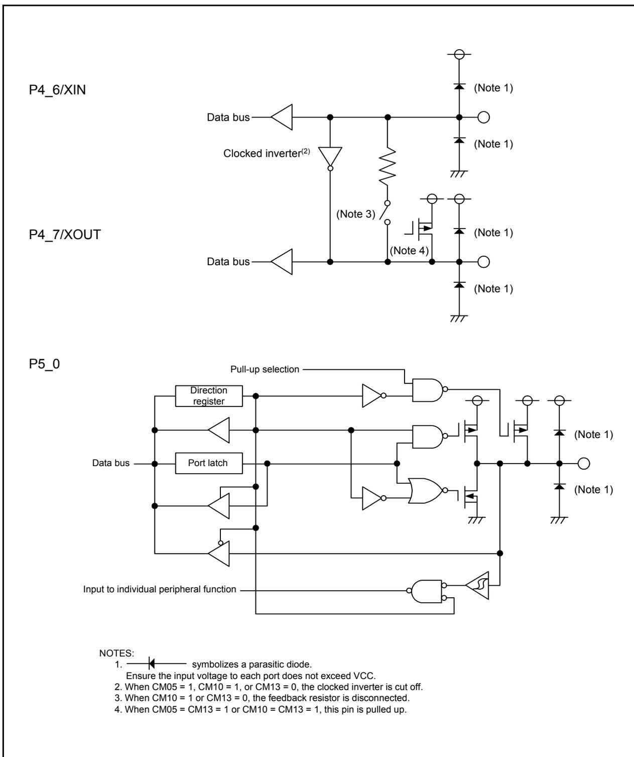
Figure 7.6 Configuration of Programmable I/O Ports (6)
