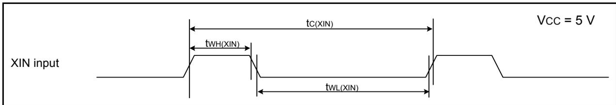
**Figure 21.8 XIN Input and XCIN Input Timing Diagram when  $V_{CC} = 5\text{ V}$** **Table 21.19 TRAIO Input,  $\overline{\text{INT1}}$  Input**
