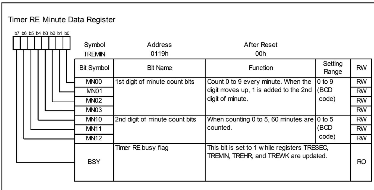
Figure 14.158 TREMIN Register in Real-Time Clock Mode
