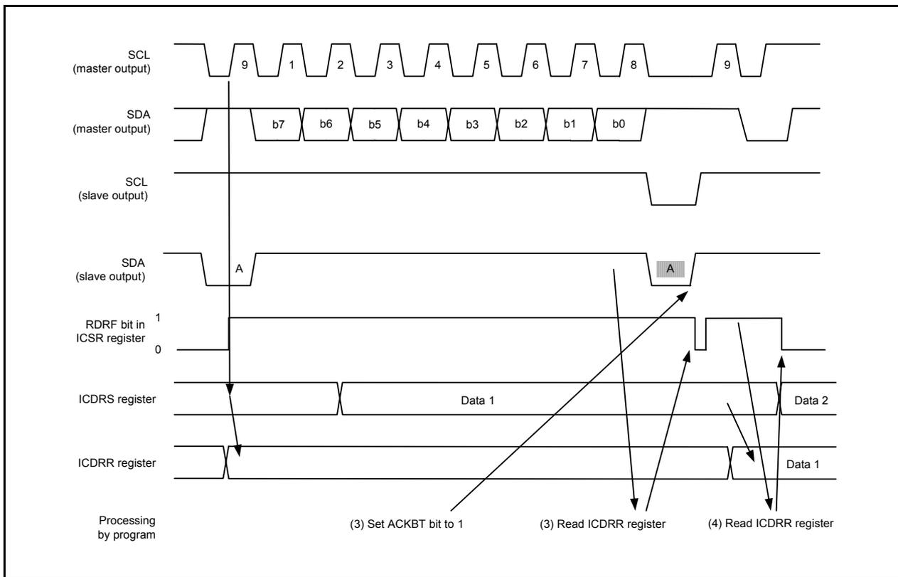
Figure 16.42 Operating Timing in Slave Receive Mode (I<sup>2</sup>C bus Interface Mode) (2)
