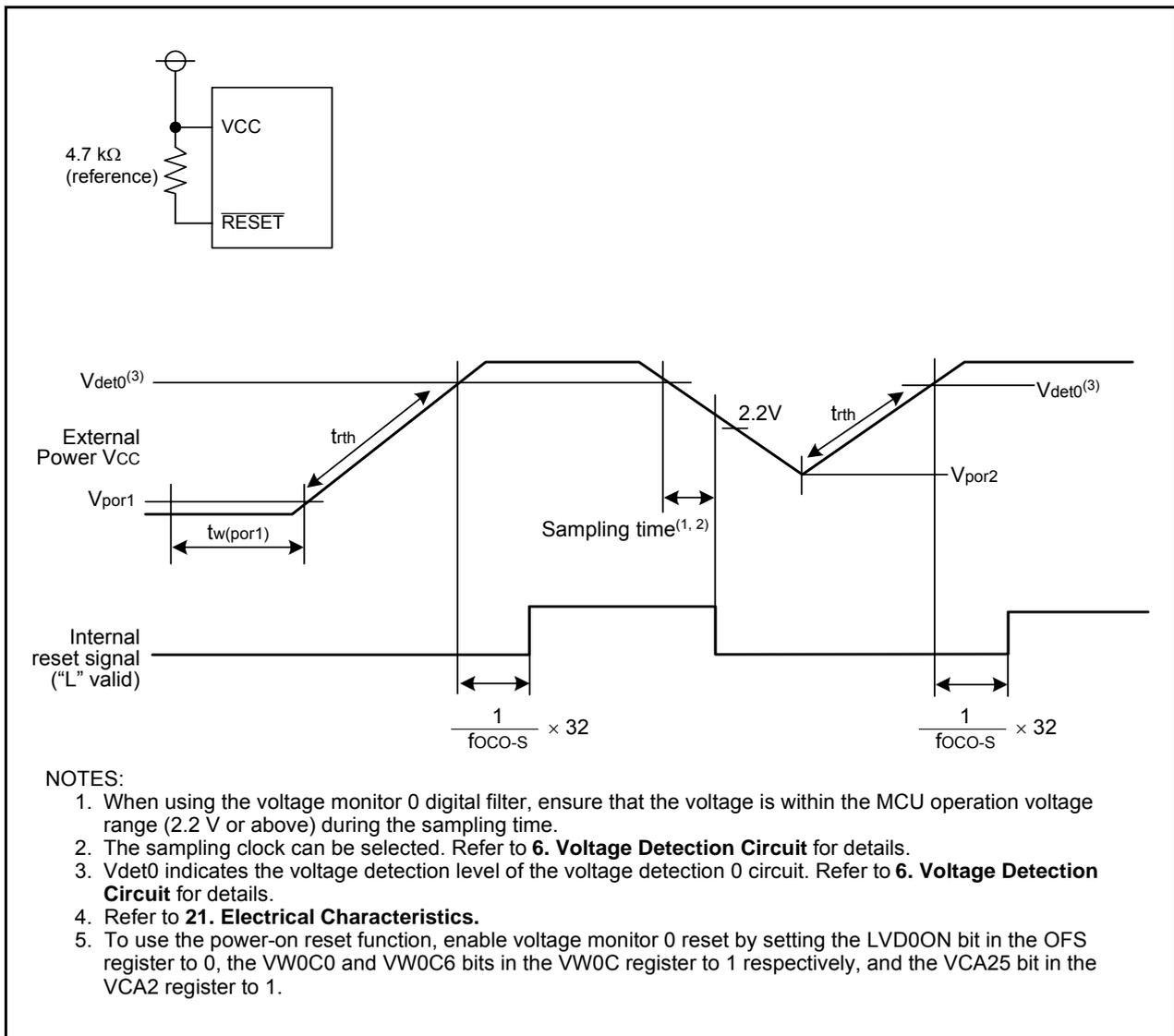
Figure 5.7 Example of Power-On Reset Circuit and Operation
