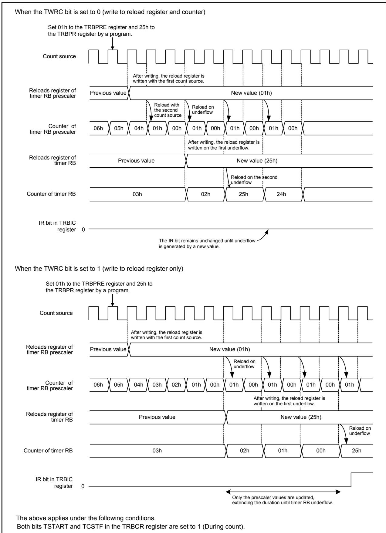
**Figure 14.17 Operating Example of Timer RB when Counter Value is Rewritten during Count Operation**
