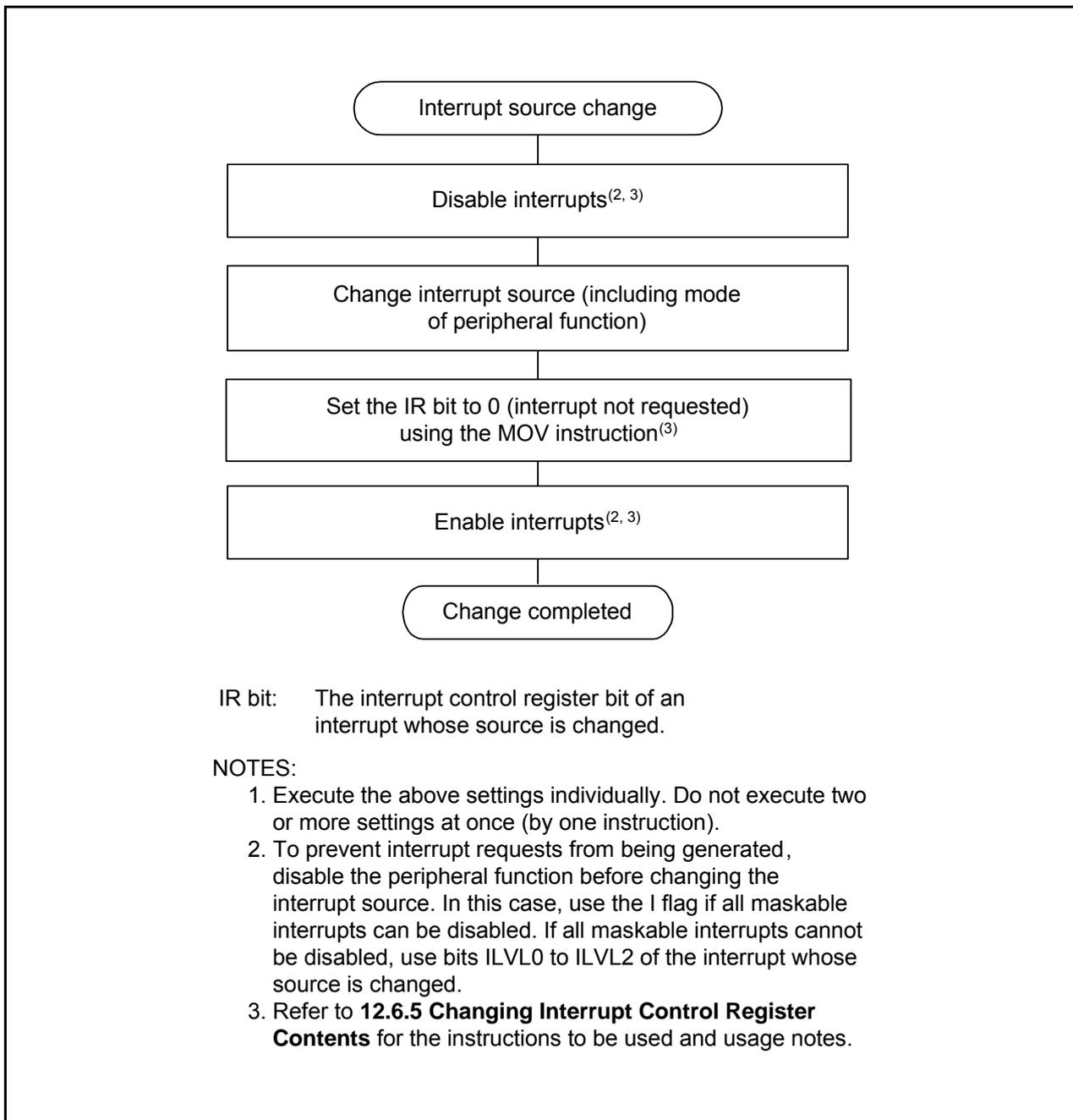
Figure 22.1 Example of Procedure for Changing Interrupt Sources
