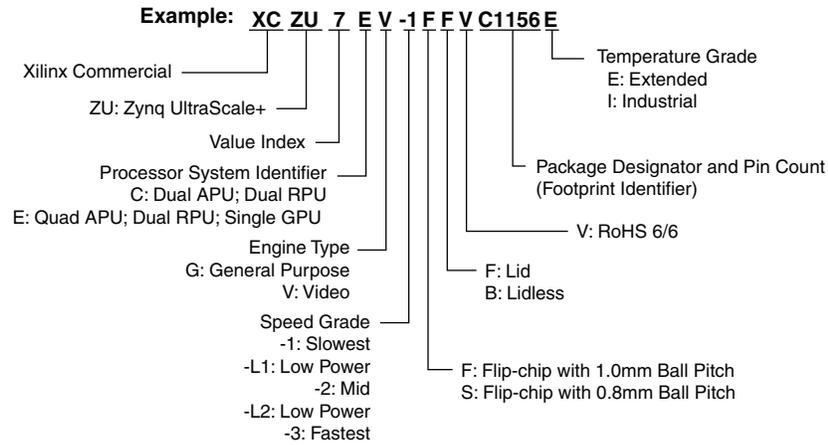
1) -L1 and -L2 are the ordering codes for the low power -1L and -2L speed grades, respectively.
