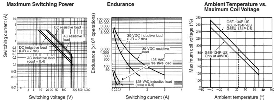
**Note:** The maximum coil voltage refers to the maximum value in a varying range of operating power voltage, not a continuous voltage.
