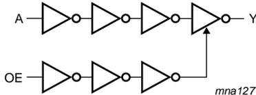
Fig 3. Logic diagram
