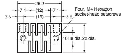
**Note:** The material is fiber-glass-reinforced polybutylene terephthalate resin (PBT).
