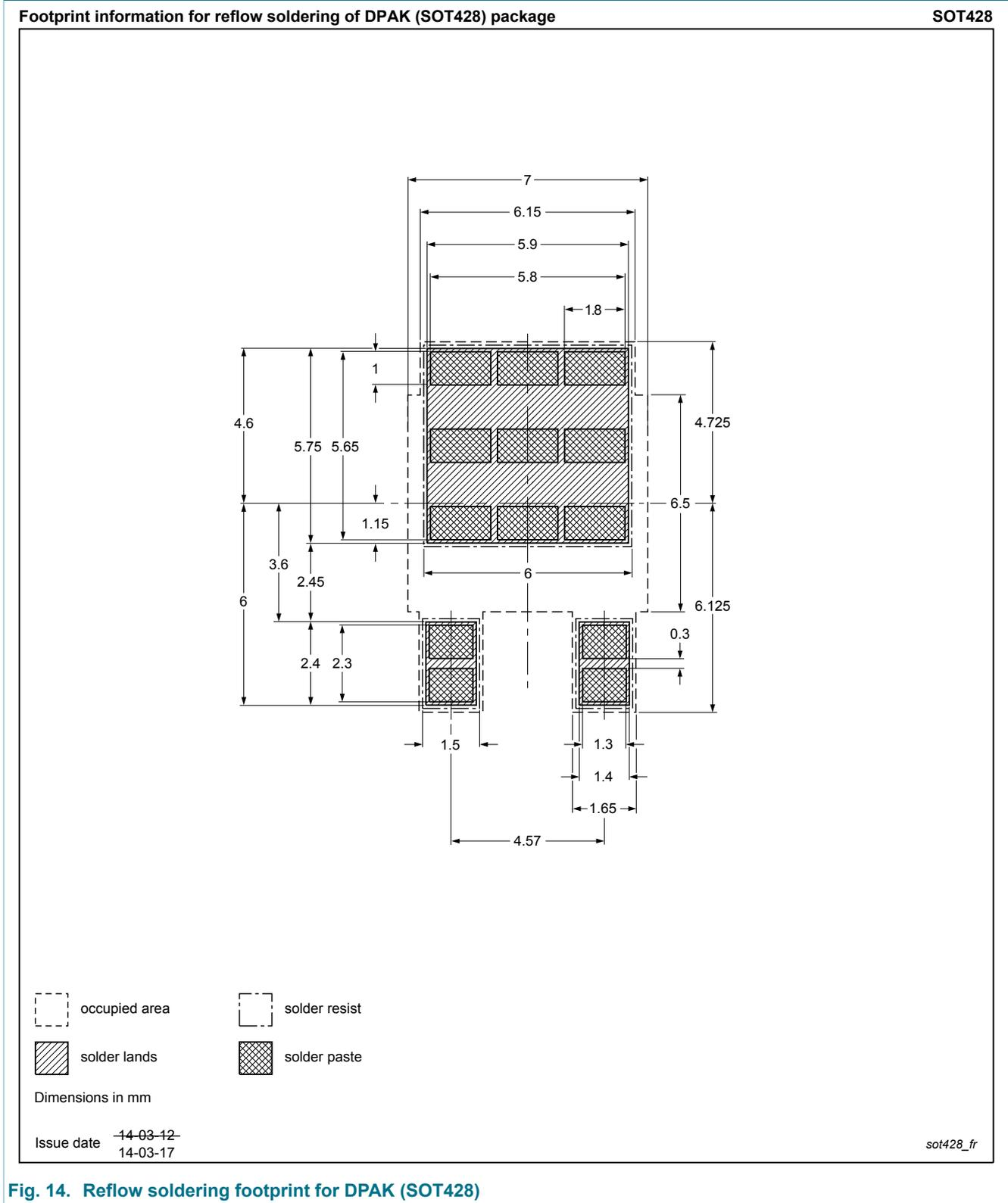
Fig. 14. Reflow soldering footprint for DPAK (SOT428)
