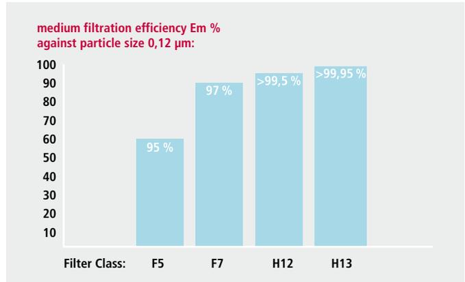
Filter Class F5, F7: Fine dust filter as per EN 779
