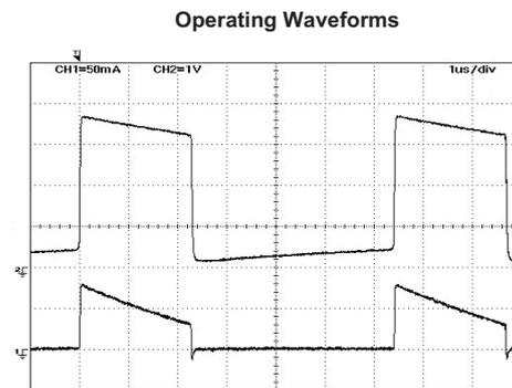
Channel 1 (lower): LED current  $I_{Led}$ . 50mA/div.
