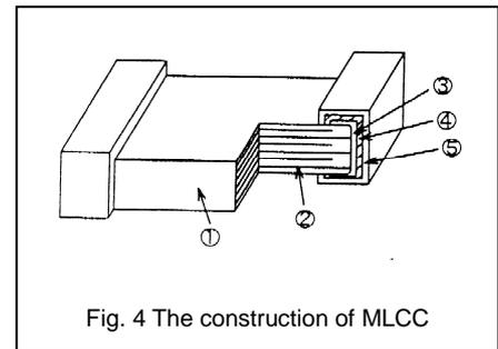
Fig. 4 The construction of MLCC
