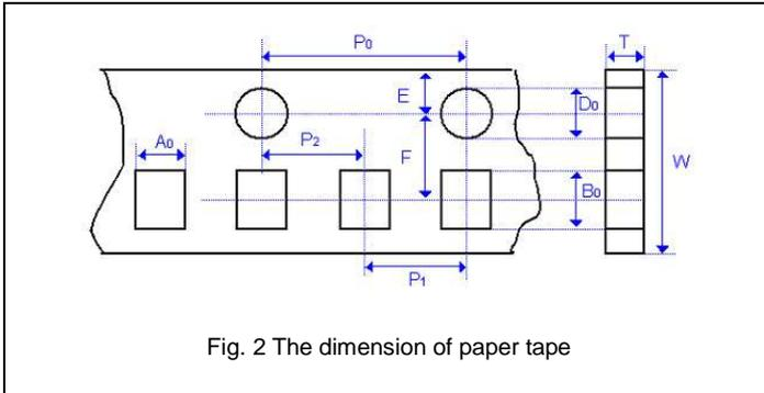
Fig. 2 The dimension of paper tape
