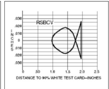
Powerful visible red beam with precise .06" diameter sensing spot. Useful in many high-contrast color registration applications.
