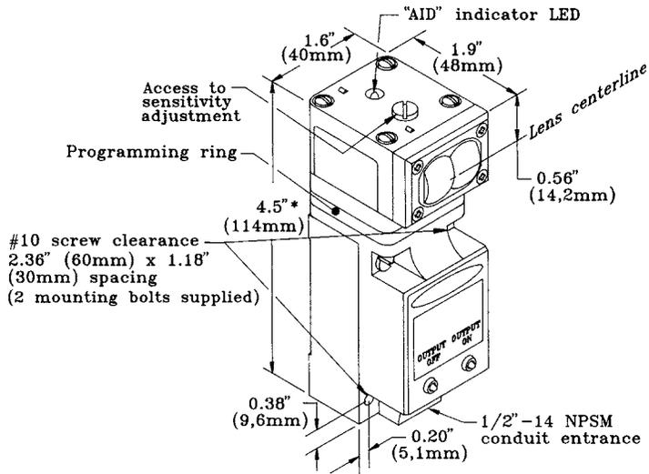
\* 5.0" (127mm) with logic module and second programming ring installed.
