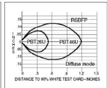
Model RSBFP is a visible-light sensor head designed for use with plastic fiber optics. It is compatible with all standard Banner plastic fiber optic assemblies (see Banner product catalog). In order to function properly, the RSBFP must be programmed for the "HS" response mode. The RSBFP is not for use with glass fiber optics (instead use model RSBF or RSBFV).
