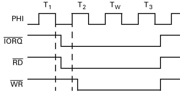
Figure 11. I/O Read and Write Cycles with  $\overline{\text{IO}}\text{C} = 1$
