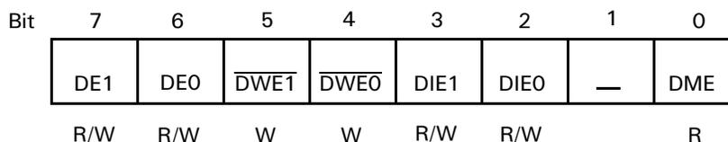
Figure 71. DMA Status Register (DSTAT: I/O Address = 30H)
