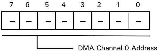
Figure 55. DMA Source Address Register 0 Low
