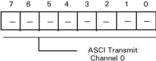
Figure 36. ASCII Register
