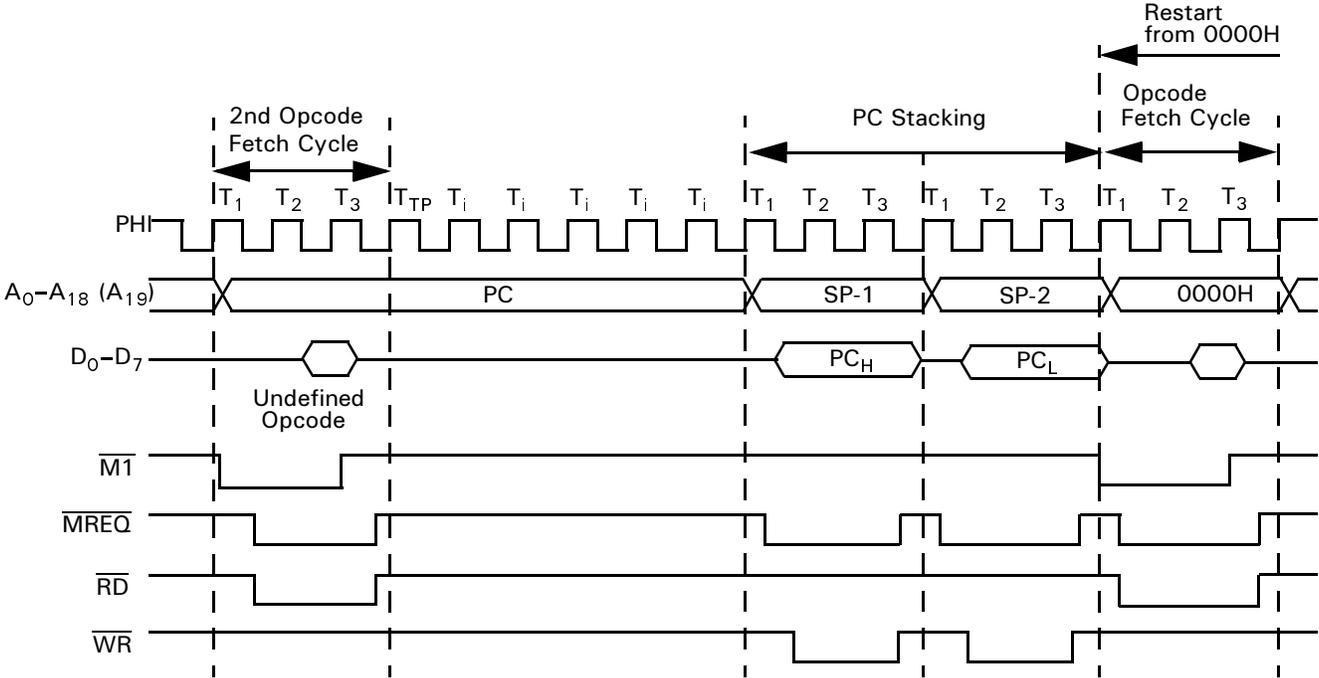
Figure 75. TRAP Timing—2<sup>nd</sup> Opcode Undefined
