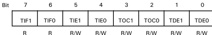
Figure 46. Timer Control Register (TCR: I/O Address = 10H)
