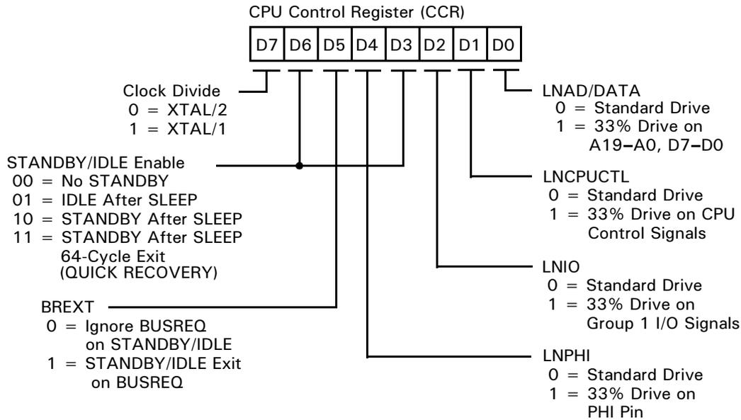
Figure 31. CPU Control Register (CCR) Address 1FH
