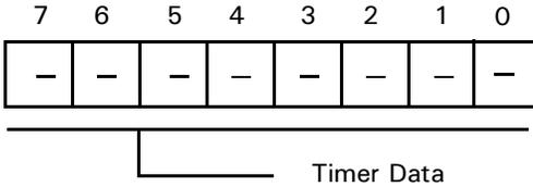
Figure 43. Timer Data Register Channel 0 High
