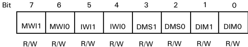
**Figure 73. DMA/WAIT Control Register (DCNTL: I/O Address = 32H)**
