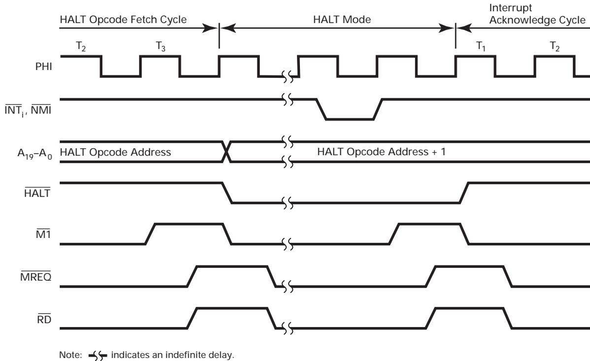
**Figure 13. HALT Timing**
