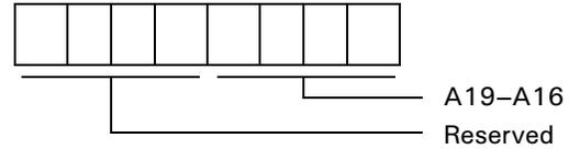
Figure 60. DMA Destination Address Register Channel 0B
