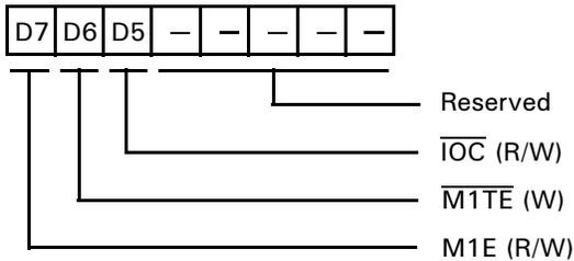
**Figure 81. Operating Control Register (OMCR: I/O Address = 3EH)**
