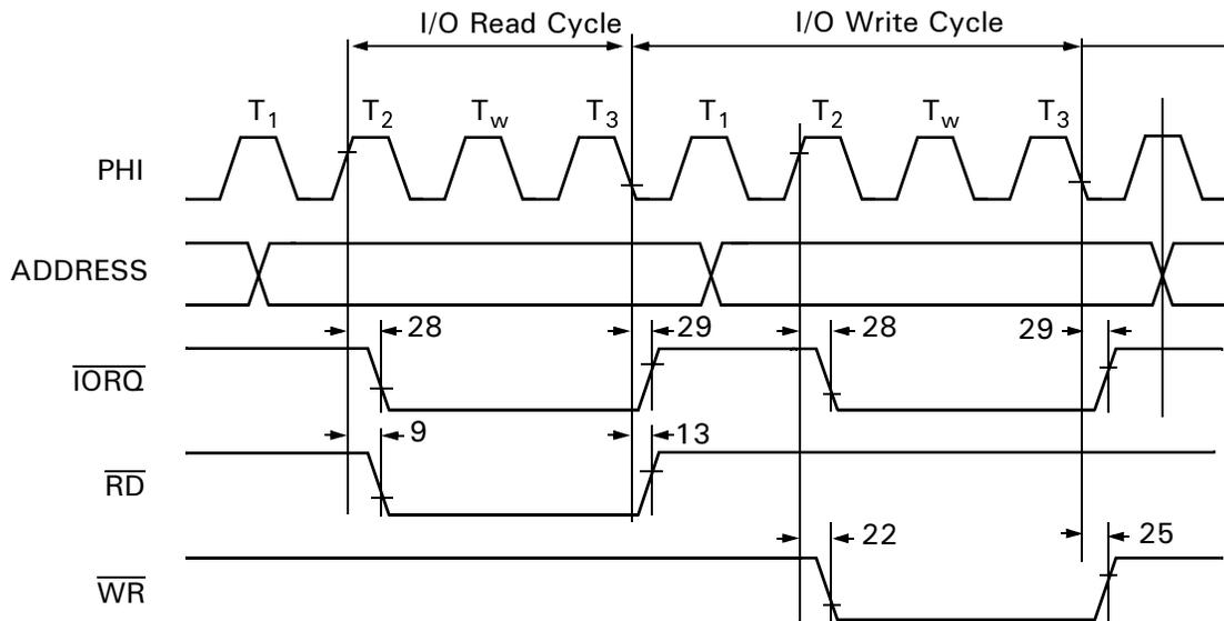
CPU Timing ( $\overline{\text{IOC}} = 0$ )
