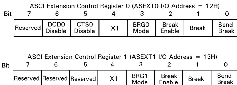
Figure 47. ASCII Extension Control Registers, Channels 0 and 1
