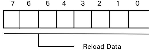
Figure 51. Timer Reload Register Channel 1 High
