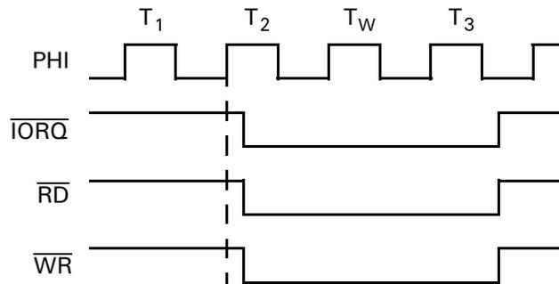
Figure 12. I/O Read and Write Cycles with  $\overline{\text{IO}}\text{C} = 0$
