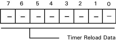
Figure 45. Timer Reload Register Channel 0 High
