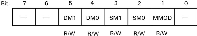
**Figure 72. DMA Mode Register (DMODE: I/O Address = 31H)**
