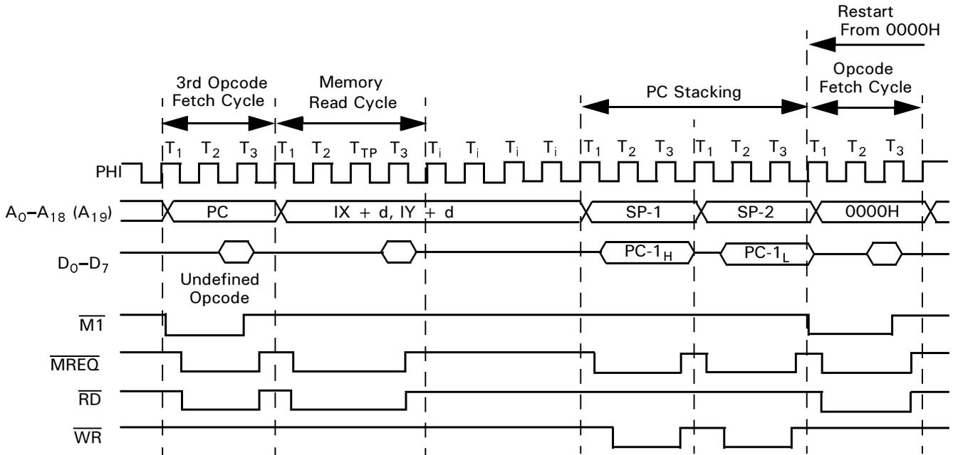
Figure 76. TRAP Timing—3<sup>rd</sup> Opcode Undefined
