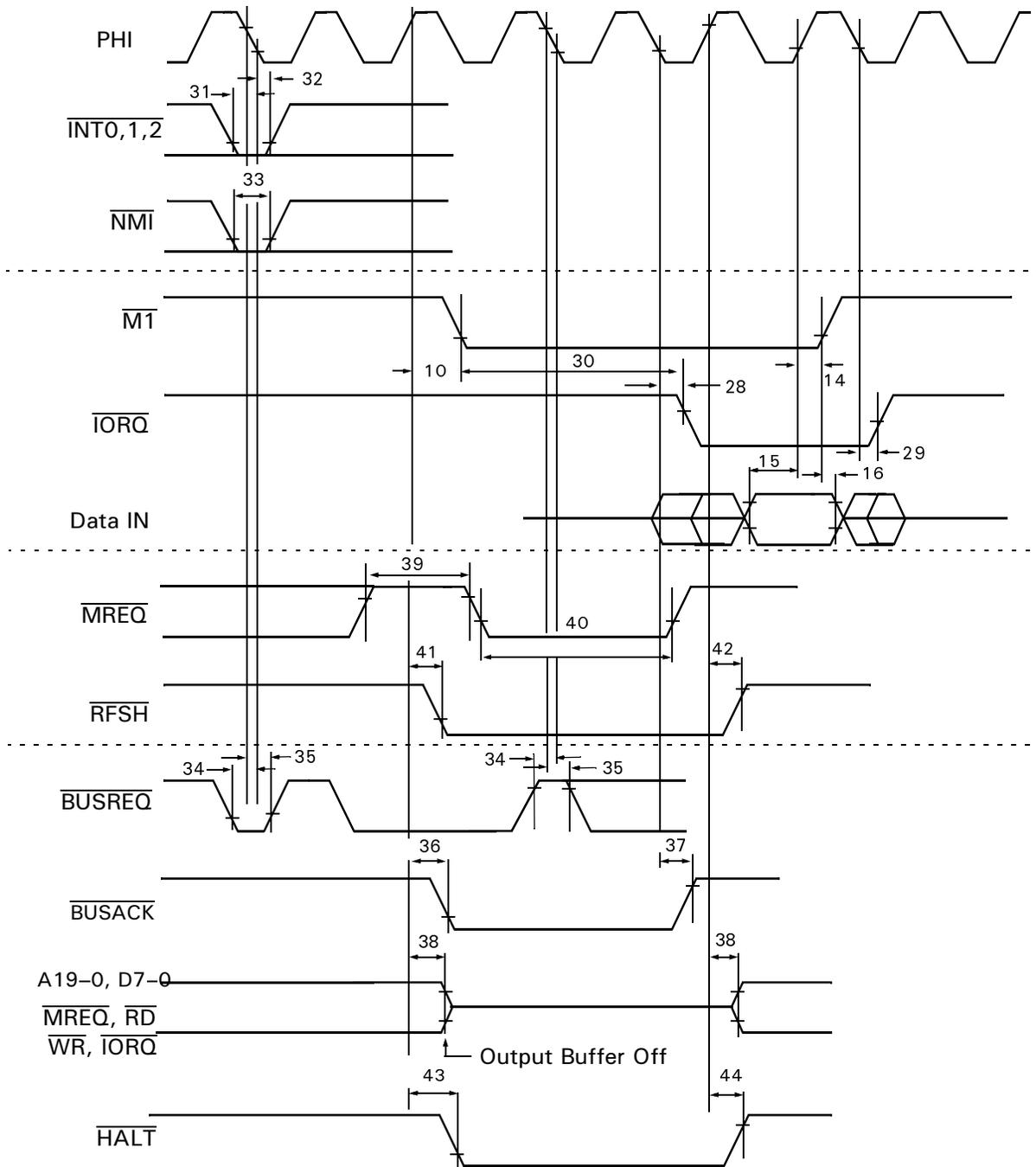
**Figure 21. CPU Timing**
