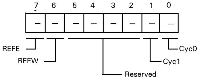
**Figure 77. Refresh Control Register (RCR: I/O Address = 36H)**
