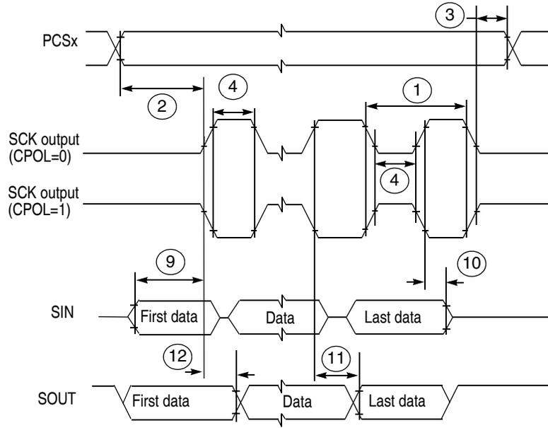
Figure 22. DSPI Modified Transfer Format Timing—Master, CPHA = 0
