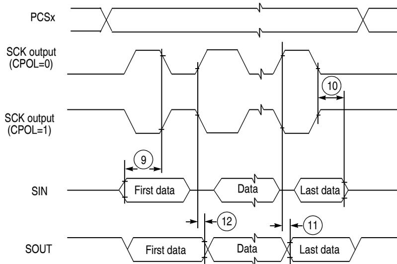
Figure 19. DSPI Classic SPI Timing—Master, CPHA = 1
