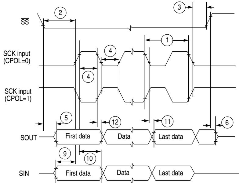
Figure 20. DSPI Classic SPI Timing—Slave, CPHA = 0
