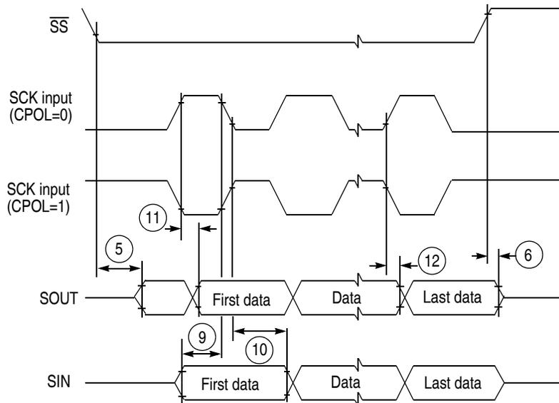
Figure 21. DSPI Classic SPI Timing—Slave, CPHA = 1
