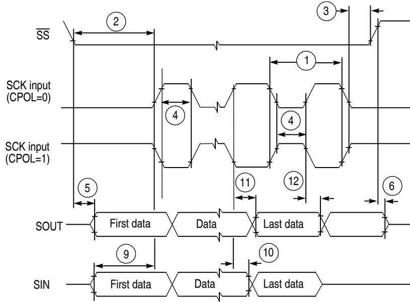
Figure 24. DSPI Modified Transfer Format Timing—Slave, CPHA = 0
