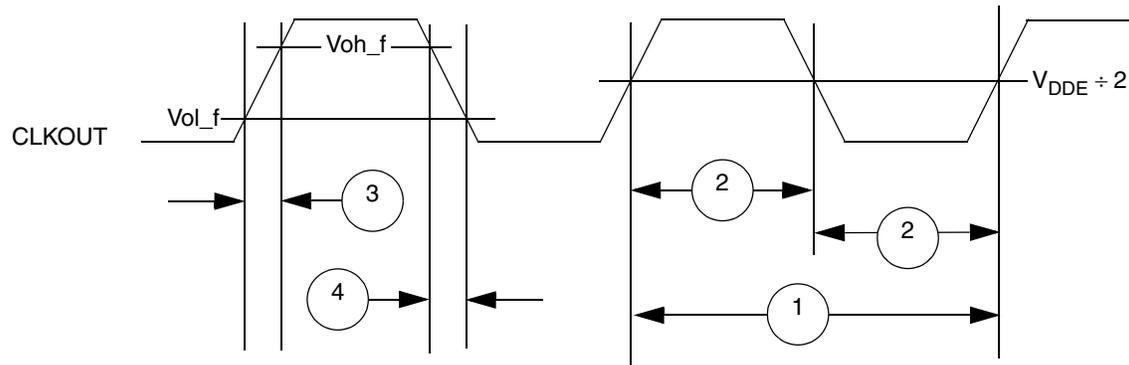
Figure 12. CLKOUT Timing
