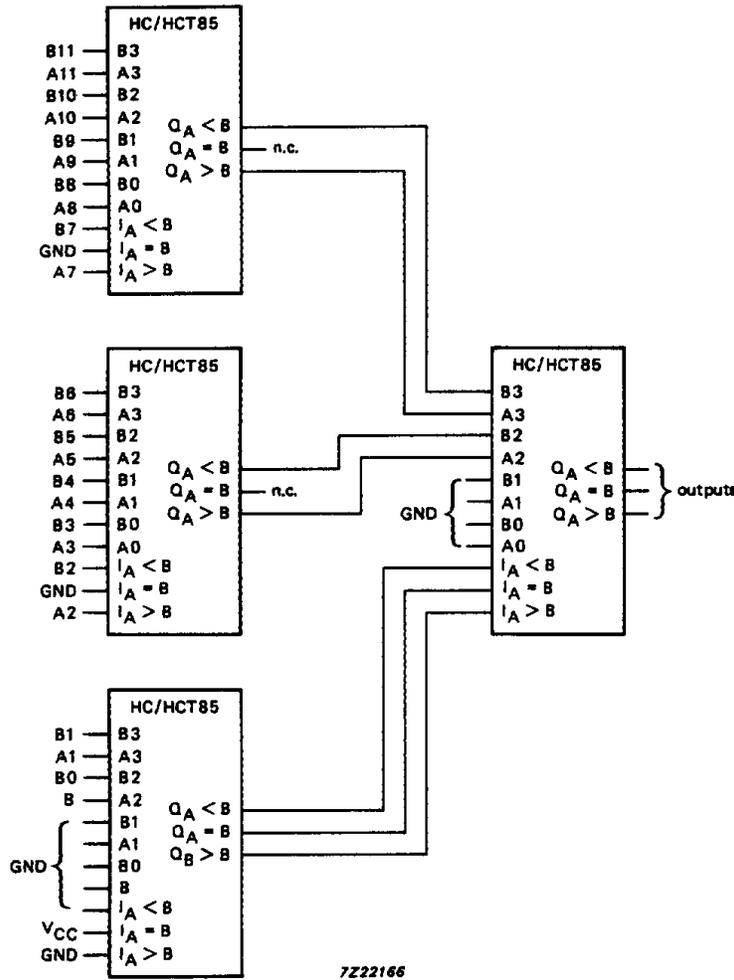
Fig.8 Parallel cascading; comparing 12-bit words.
