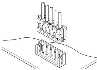
This, the thinnest, 2.5mm pitch connector, is 8.1mm in height after mounting and 3.8mm in width. It is designed to meet the demand for the high-density connection of internal wires to printed circuit boards. It is compact, highly reliable and low in cost.
