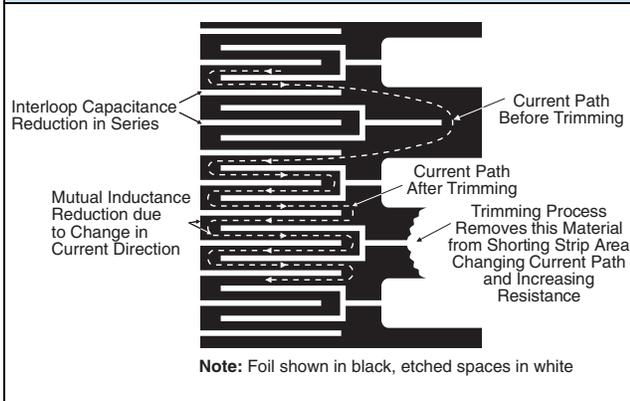
\* To acquire a precision resistance value, the Bulk Metal® Foil chip is trimmed by selectively removing built-in “shorting bars.” To increase the resistance in known increments, marked areas are cut, producing progressively smaller increases in resistance. This method eliminates “hot spot” and improves the long term stability of the resistor.
