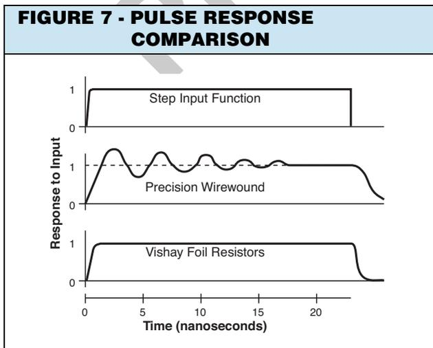
Figure 7 shows the current response to a voltage pulse comparing a fast Bulk Metal® Foil resistor to a slower wirewound resistor. Here a pulse width of one nanosecond would have been completely missed by the wirewound resistor while the Vishay Foil resistor achieves full replication in the time allotted.
