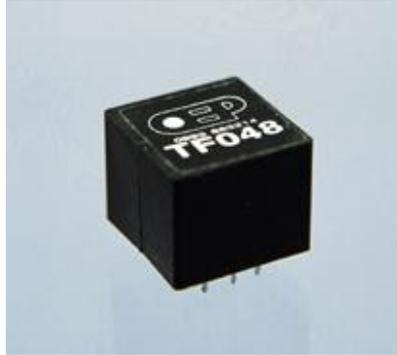
PCB mounting encapsulated 600:600  $\Omega$  line transformer offering improved performance over the OEP1200 and similar devices. A three part concentrically wound bobbin is utilised to provide improved primary to secondary coupling together with improved frequency response and return loss characteristics.
