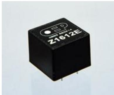
This 600:600  $\Omega$  Line Isolation/Matching Transformer is a very low distortion version of the industry standard OEP1200 device for use in V.34 applications. In common with that product this transformer is designed for use where the telephone line current is diverted from the winding by a choke or solid state device. Its use will enable users to comply with the requirements of BS6305.
