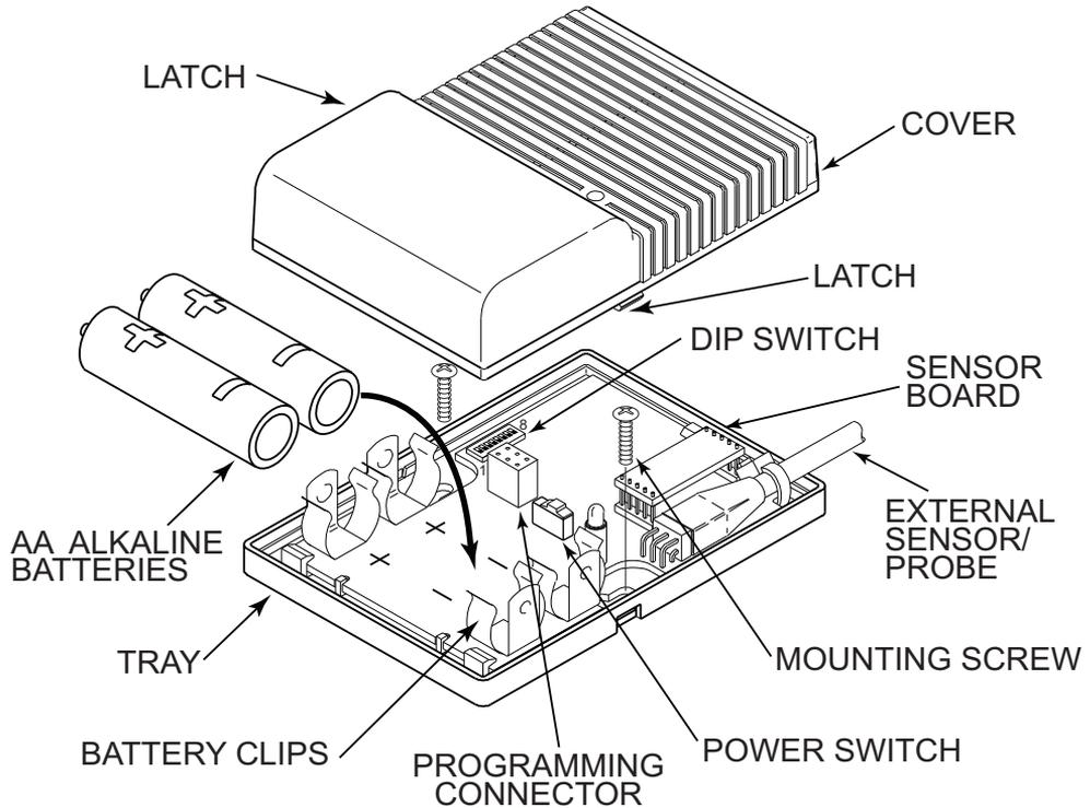
**Figure 2.4f Disassembly of the End Device (zED)**
