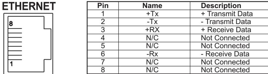
Figure 2.10 RJ45 Pinout
