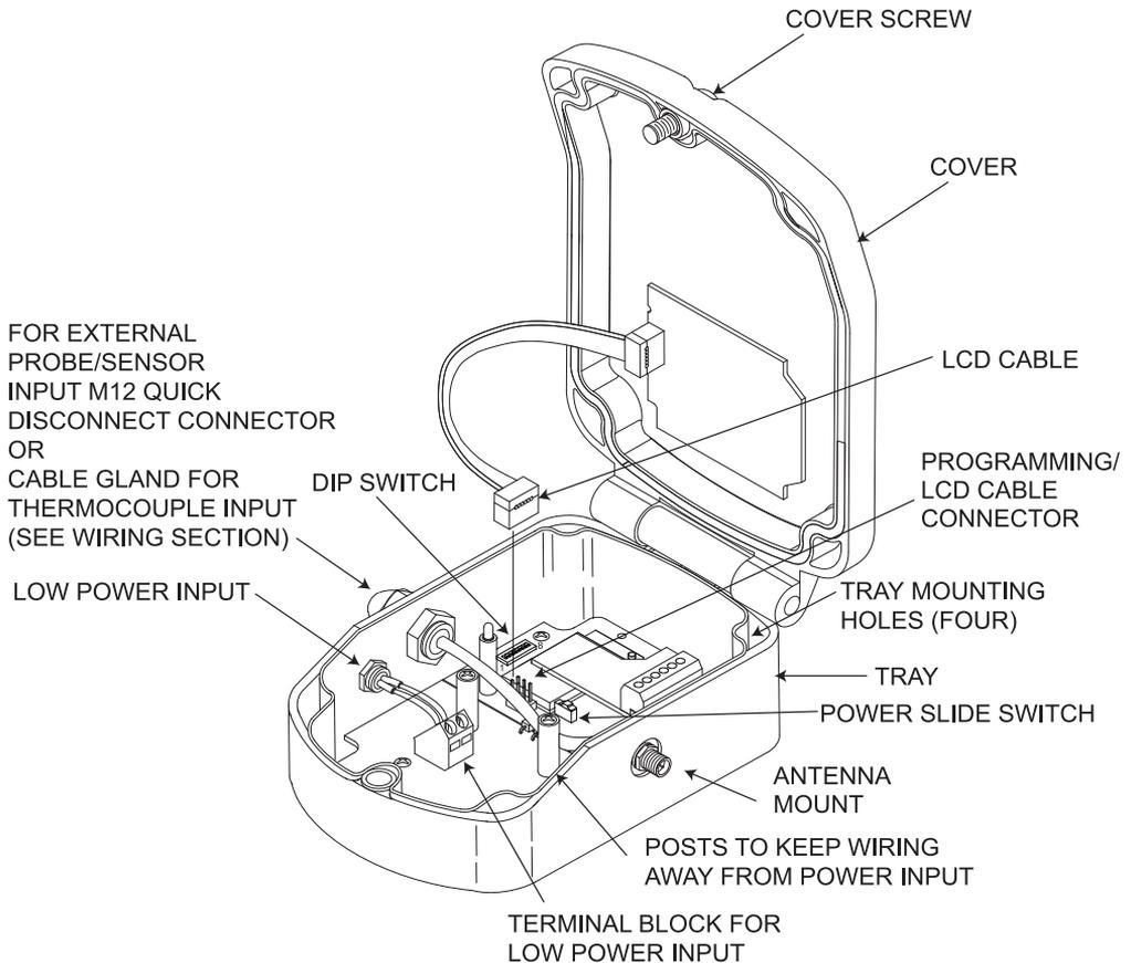
**Figure 2.3d Disassembly of the End Device (zED-DC-H2)**
