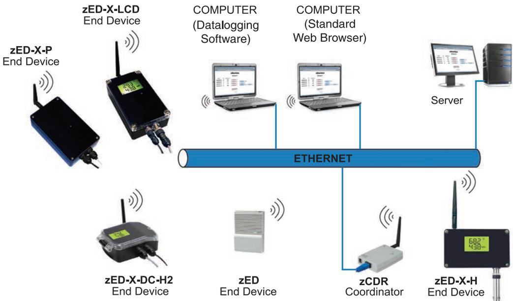
Figure 1.1 zSeries Wireless System on the Ethernet Network
