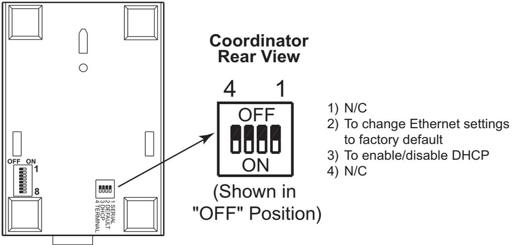
**Figure 2.9 Ethernet - 4 Position DIP Switch Setup**
