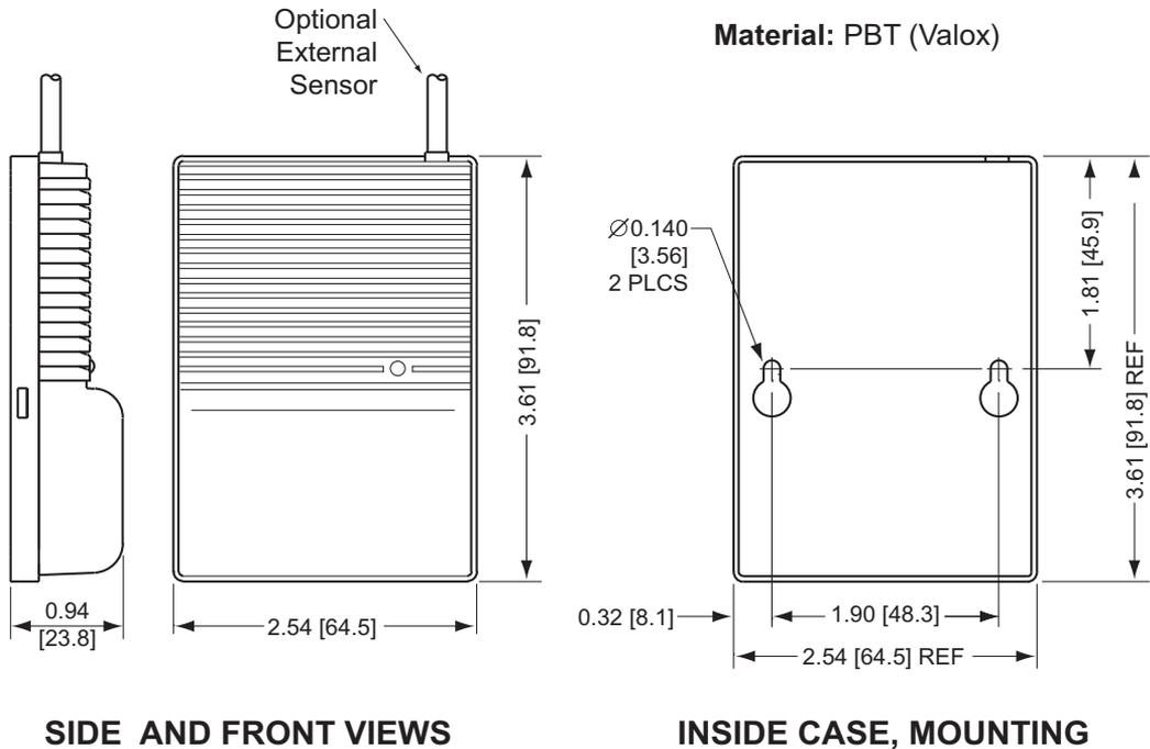
Figure 2.2c Mounting the End Device (zED)
