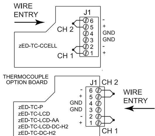
Figure 2.12 Thermocouple Wiring and TC Wire Color Chart
