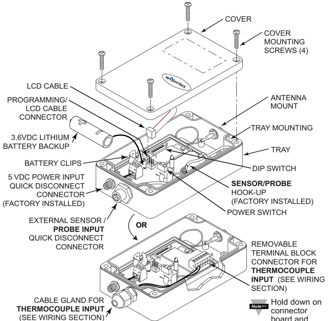
**Figure 2.4a Disassembly of the End Device
