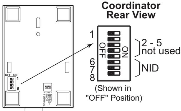
**Figure 2.8 Network ID (NID) - 8 Position DIP Switch Setup**
