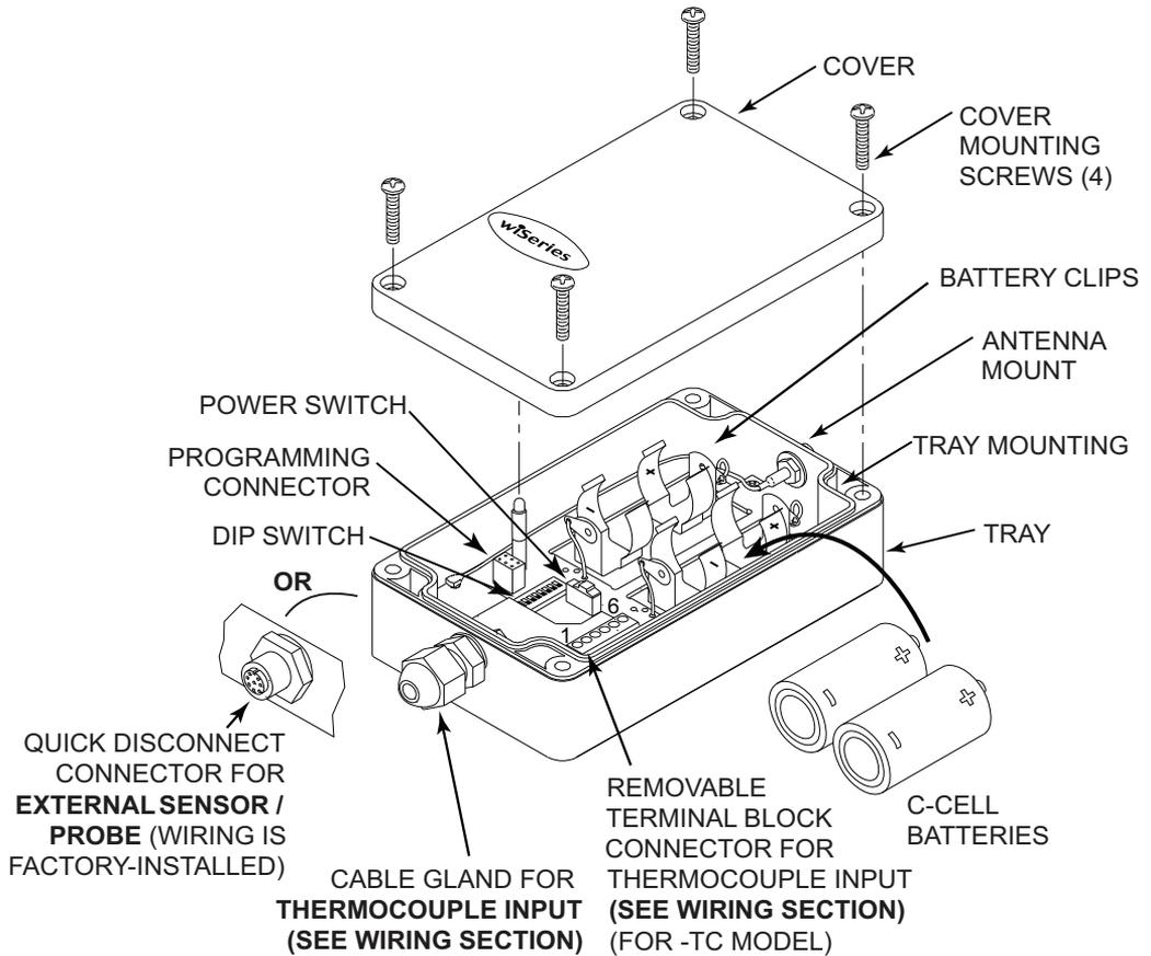
**Figure 2.4c Disassembly of the End Device (zED-x-CCELL or zED-TC-CCELL)**
