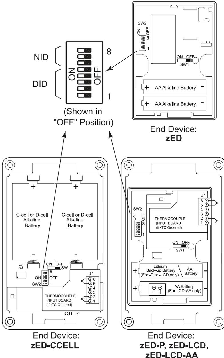
Figure 2.7a Device ID (DID) - 8 Position DIP Switch Setup
