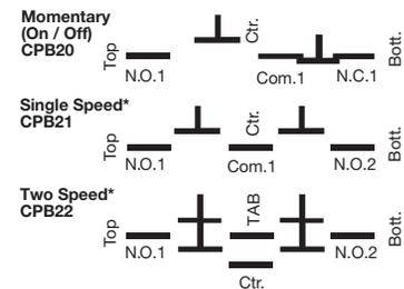
\*Mechanical "floating ball" interlock prevents activating both Pushbuttons simultaneously.
