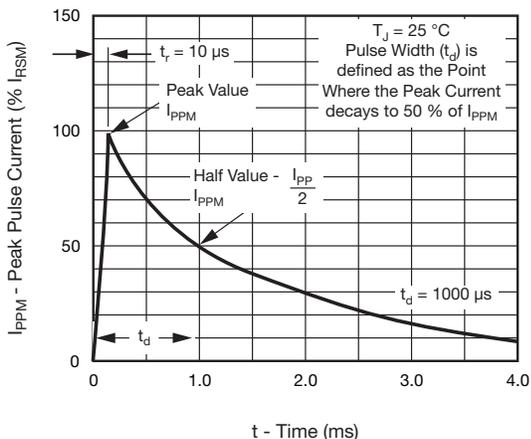
Fig. 3 - Pulse Waveform
