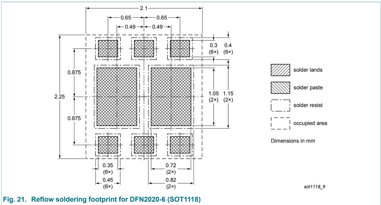
Fig. 21. Reflow soldering footprint for DFN2020-6 (SOT1118)
