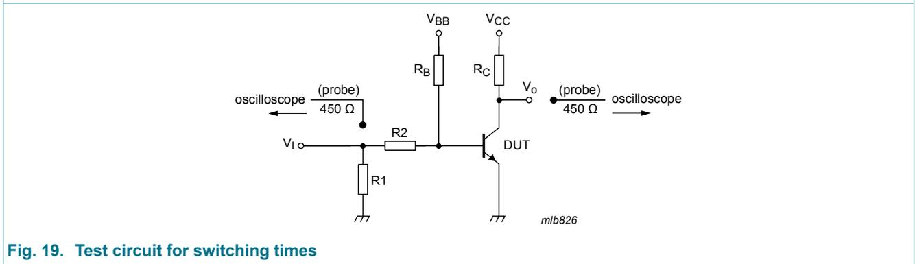
Fig. 19. Test circuit for switching times
