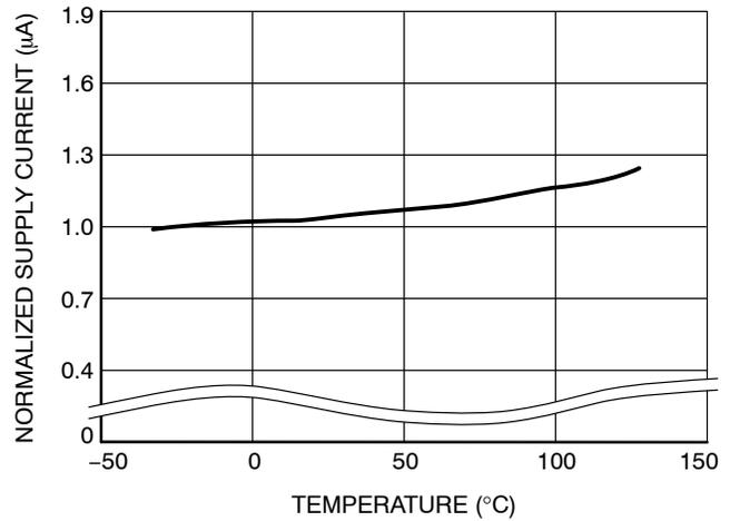
**Figure 3. Supply Current vs. Temperature (No Load, CAX8xxR/S/T/Z)**
