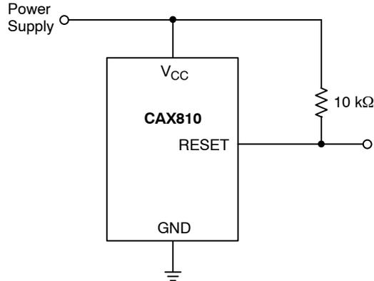
Figure 9. RESET Valid with  $V_{CC}$  Under 1.1 V
