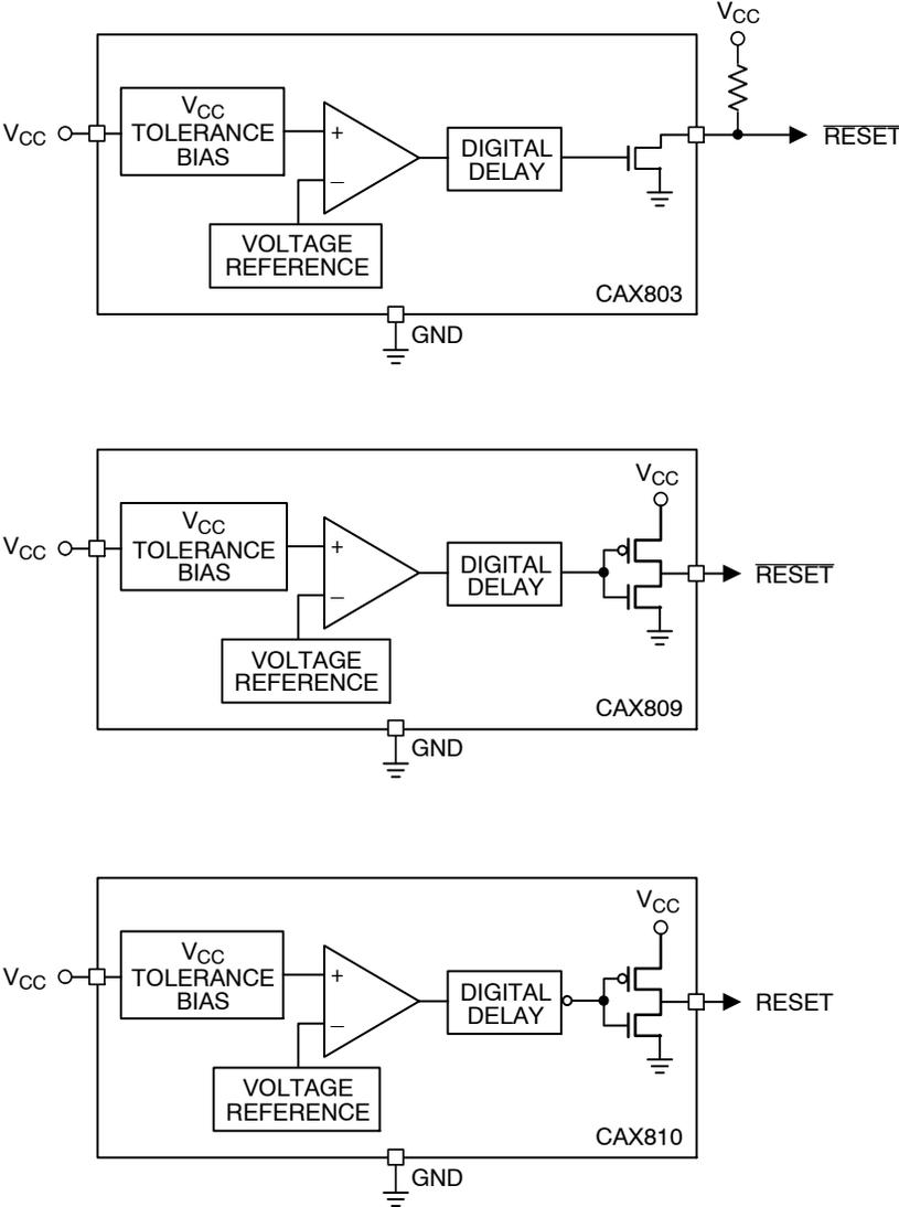
**Figure 1. Block Diagrams**
