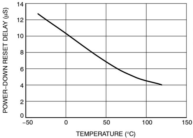
**Figure 4. Power-down Reset Delay vs. Temperature (CAX8xxR/S/T/Z)**
