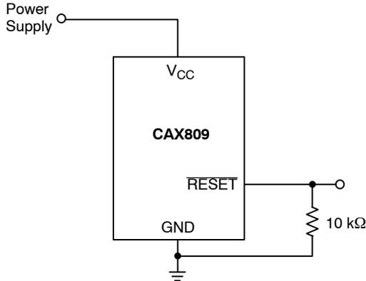
Figure 8. RESET Valid with  $V_{CC}$  Under 1.0 V
