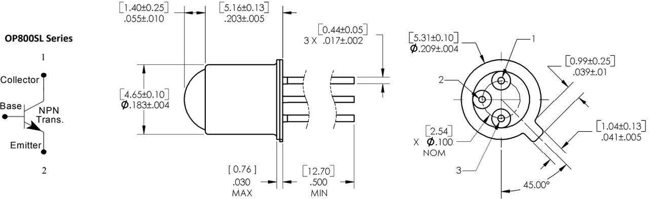
DIMENSIONS ARE IN: [MILLIMETERS]
