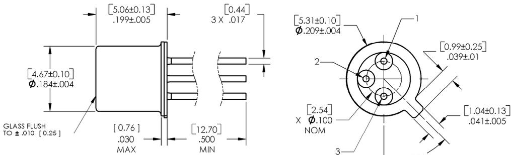
DIMENSIONS ARE IN: [MILLIMETERS]
