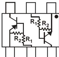
R<sub>1</sub>, R<sub>2</sub> Device Schematic
