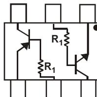
R<sub>1</sub> Only Device Schematic
