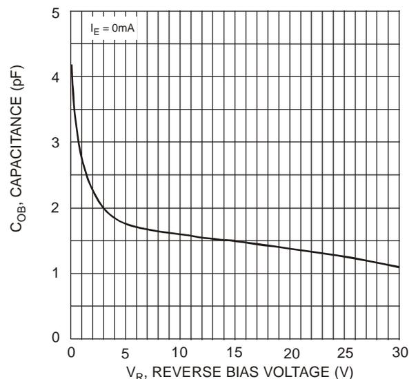
Fig. 4 Output Capacitance
