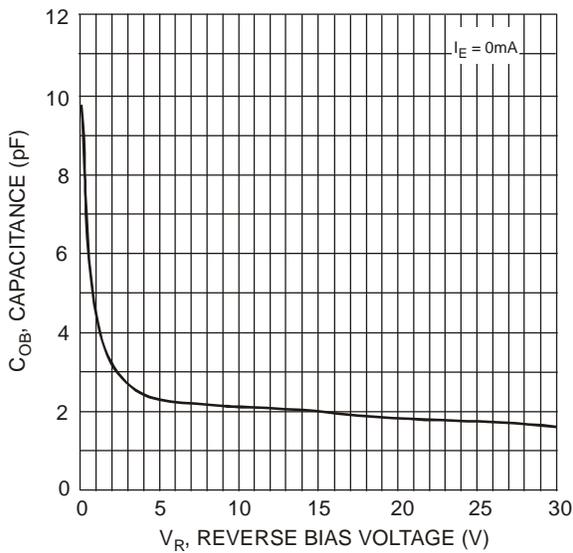
Fig. 9 Output Capacitance
