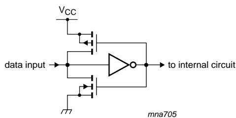
Fig 3. Bus hold circuit
