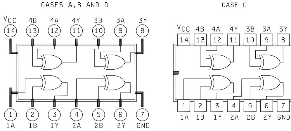
Figure 1. Terminal connections (top view).
