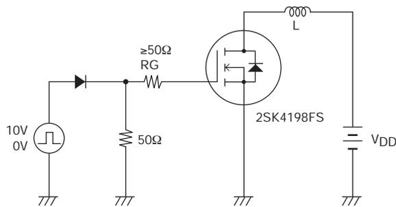
Fig.2 Switching Time Test Circuit
