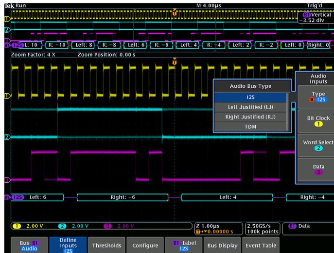
I<sup>2</sup>S bus setup, showing input configuration options for I<sup>2</sup>S bus.
