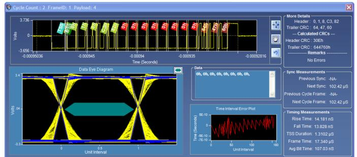
PC-based, eye-diagram analysis software builds an eye-diagram from the entire acquisition and plots it against TP1 mask called out by the FlexRay standard, available with MSO/DPO4000B and MDO4000B instruments.
