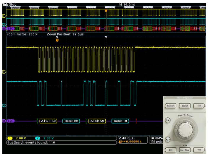
Search – I<sup>2</sup>C decode showing results from a Wave Inspector® search for Address value 50. Wave Inspector® controls provide unprecedented efficiency in viewing and navigating waveform data.
