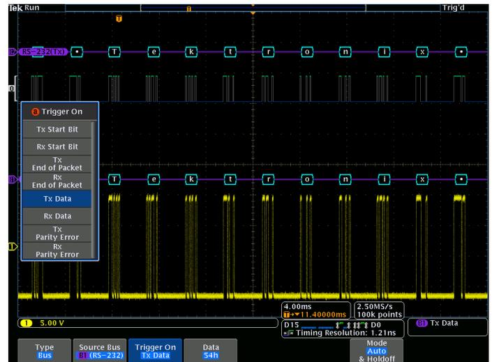
Triggering on a specific transmit data packet going across an RS-232 bus. A complete set of triggers, including triggers for specific serial packet content, ensures you quickly capture your event of interest.
