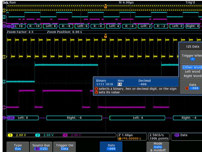
Triggering on a specific data value on the I<sup>2</sup>S bus.
