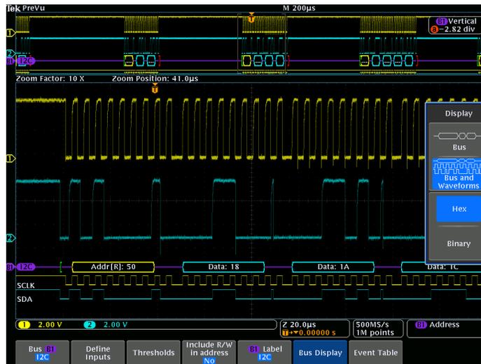
I<sup>2</sup>C bus setup, showing selection of bus display modes.
