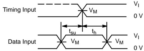
**Figure 11. Voltage Waveforms Setup and Hold Times**
