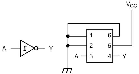
Figure 7. Inverter (When B = C = "L")
