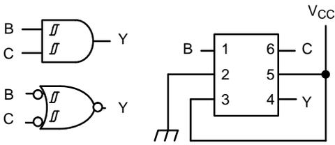
Figure 2. 2-Input AND (When A = "H")
