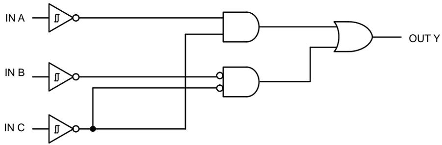
Figure 1. Function Diagram
