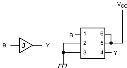
Figure 8. Buffer (When A = "L" and C = "H")
