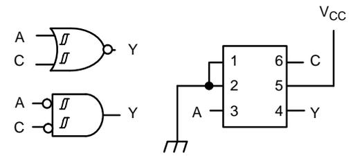
Figure 5. 2-Input NOR (When B = "L")
