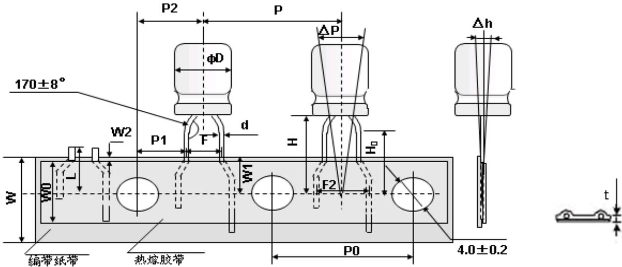
Fig-2 for  $\Phi 5$  F=2.0(TT) ;  $\Phi 6.3$  F=2.5(TU);  $\Phi 8 \times 5$  F=2.5(TU);  $\Phi 8 \times 7 \sim 20$  F=3.5mm(TV)
