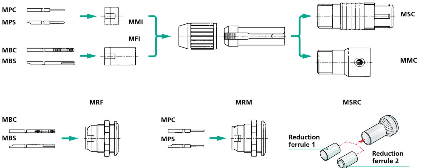
Housing and insert pre-assembled, contacts must be ordered separately.
