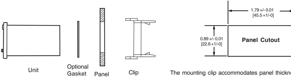
The mounting clip accommodates panel thicknesses up to 1/4" [6.4mm].
