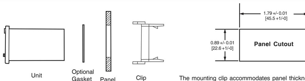
The mounting clip accommodates panel thicknesses up to 1/4" [6.4mm].
