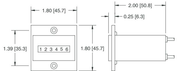
Mounting holes: For #5 flat head screw
