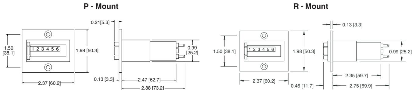
Mounting holes: For #8 flat head screw
