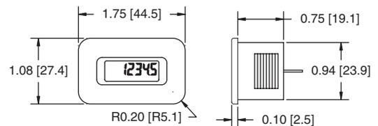
Compact Bezel Design, Spring clip retainer, Fast installation, Panel cutout 1.46 x 0.95 [37.1 x 24.1] opening.
