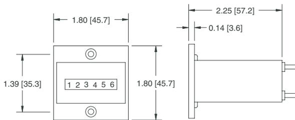
Mounting holes: For #5 flat head screw
