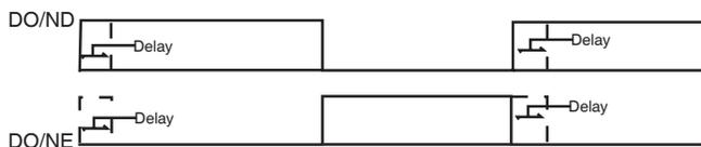
Output activates as input signal drops below setpoint (Low Alarm)
