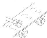
Generating pulses from idler roll with RPG
