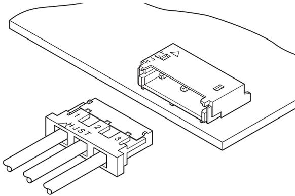
**Low profile connectors with high withstanding voltage, designed for connecting liquid crystal display back light lamps to their starters.**
