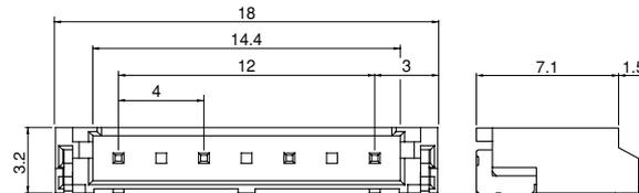
(4 circuits 4mm pitch with post removed)
