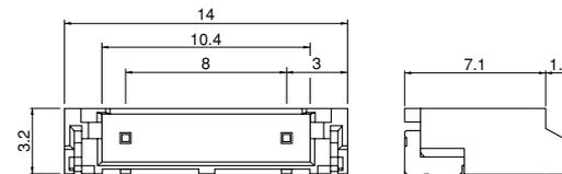
(2 circuits 8mm pitch with ribs against prying)
