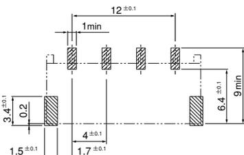
(4 circuits 4mm pitch with post removed)
