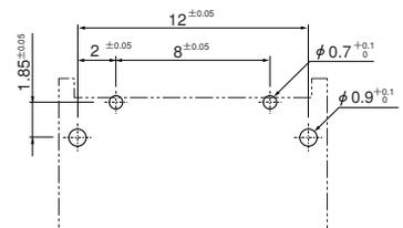
Note: 1. Tolerances are for pattern non-cumulative:  $\pm 0.05\text{mm}$  for all centers. Tolerance for hole size is  $\pm 0.1$ .
