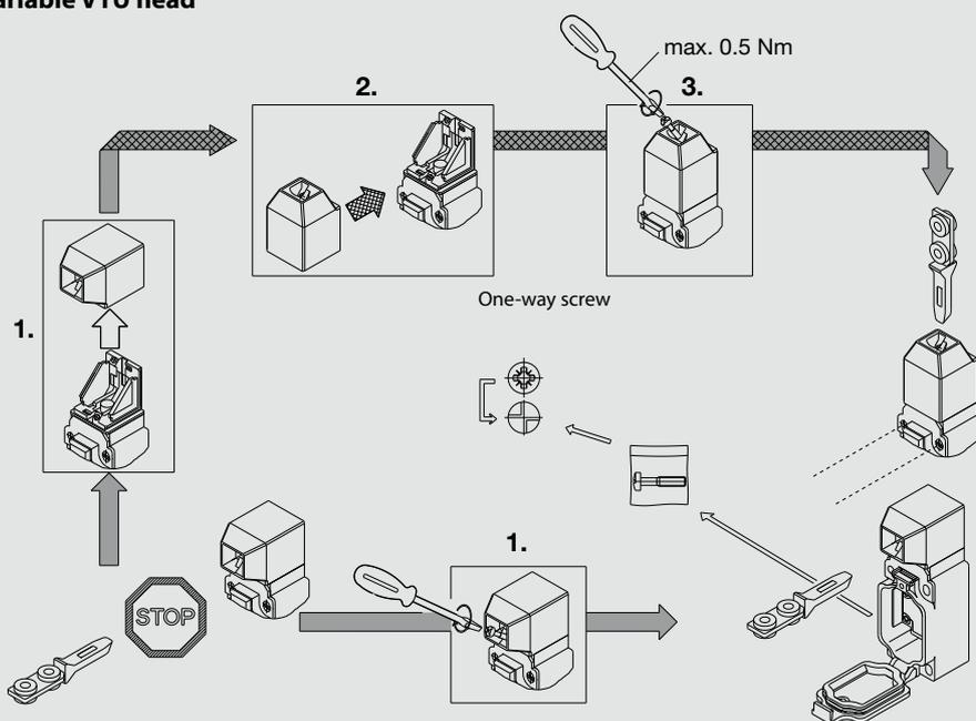
Repositioning the actuator head either in horizontal or vertical direction results in 8 approach actuator directions.
