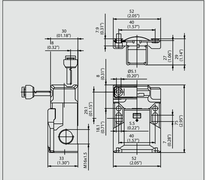
In terms of lengths, the SKC safety position switch is the 15 mm shorter variant of the SK. This makes it the right choice for confined installation conditions.
