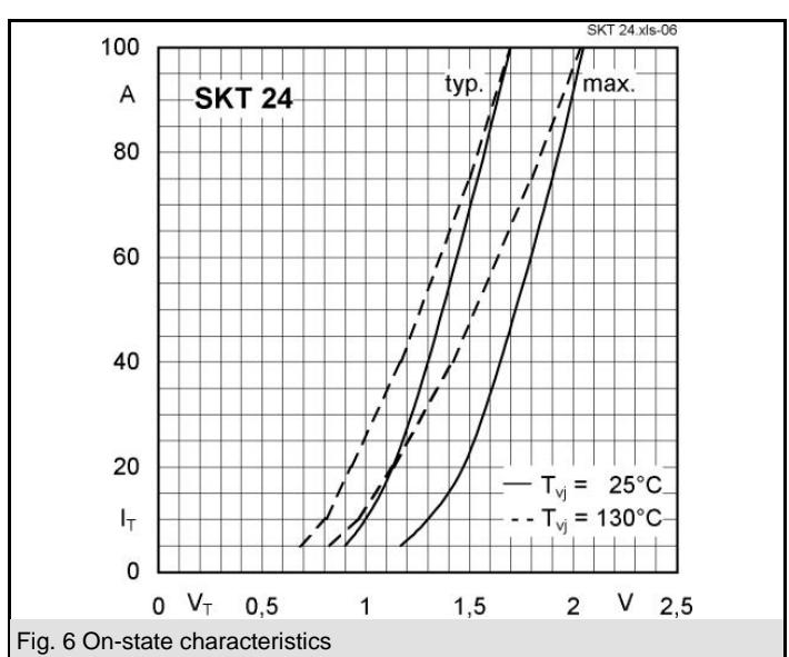
Fig. 6 On-state characteristics
