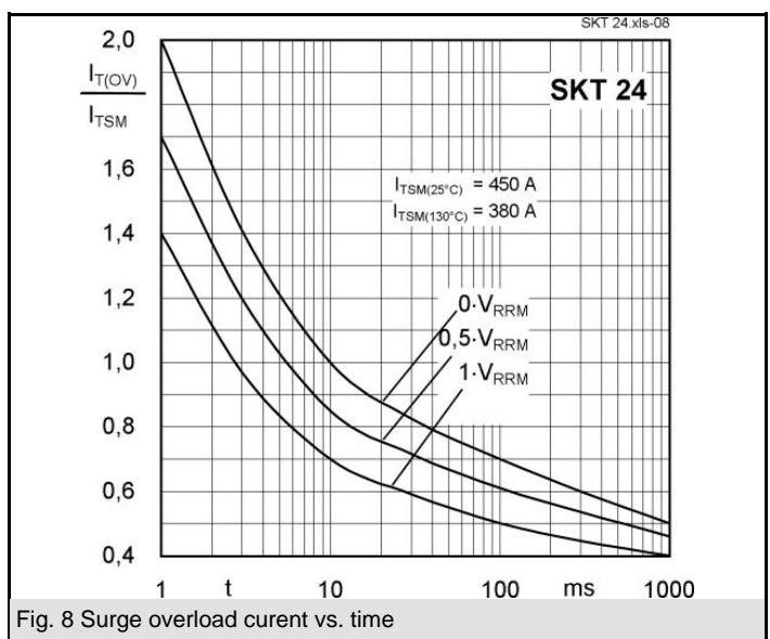
Fig. 8 Surge overload current vs. time
