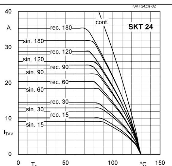
Fig. 2 Rated on-state current vs. case temperature
