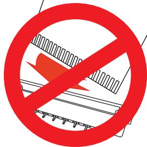
**Do not keep FFC inclined when insertion**
