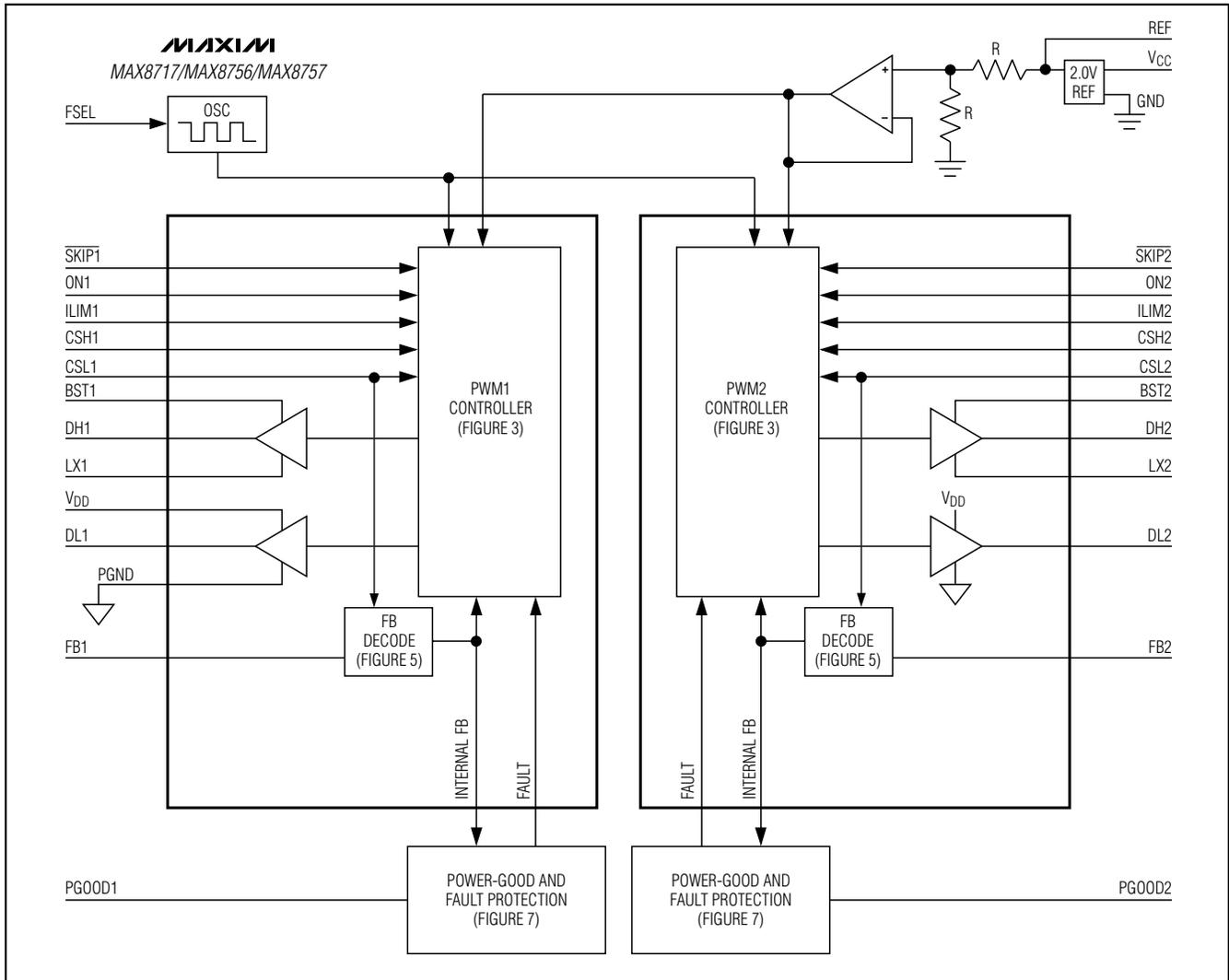
Figure 2. Functional Diagram
