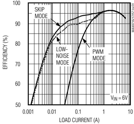
**3.3V OUTPUT EFFICIENCY vs. LOAD CURRENT**
