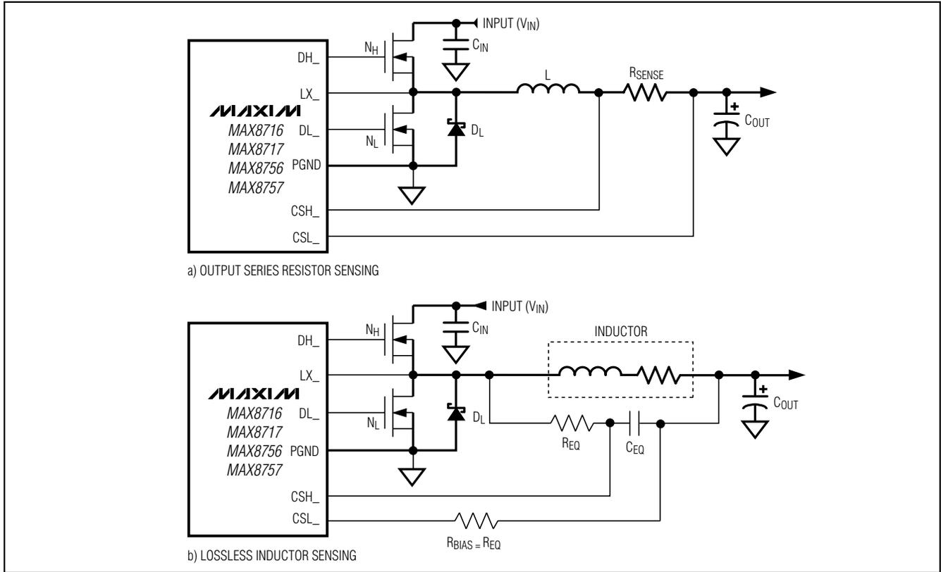
Figure 8. Current-Sense Configurations
