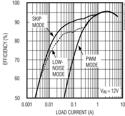
**3.3V OUTPUT EFFICIENCY vs. LOAD CURRENT**
