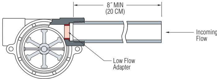
Except for straight-thread versions, RotorFlow sensors connect to piping via NPT mating thread forms. The use of an appropriate thread sealant is necessary to assure a leak-tight connection. Permatex "No More Leaks" or 2 wraps of Teflon tape are the only sealants recommended for GEMS flow sensors. Straight-thread versions require an O-ring for sealing.
