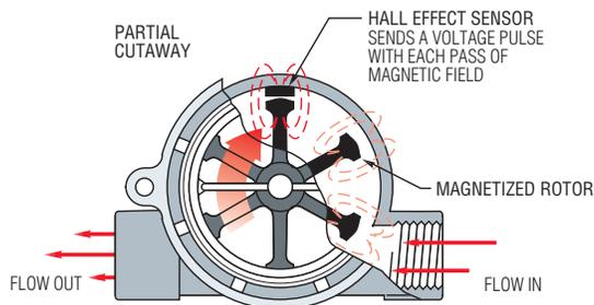
1. As liquid passes through the RotorFlow body, the magnetic rotor spins at a rate proportional to flow. This causes a series of magnetic fields (the rotor vanes) to excite the Hall Effect sensor, producing a series of voltage pulses.
