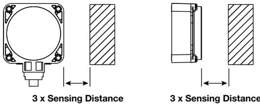
**Sensor-to-Sensor Isolation Minimum Distances**
