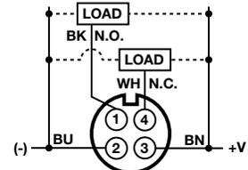
*Auto-Configure enables load to be wired to +V or (-)*
