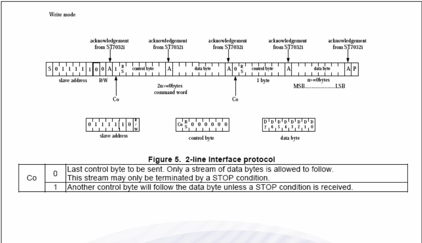
During write operation, two 8-bit registers are used. One is data register (DR), the other is instruction register (IR).
