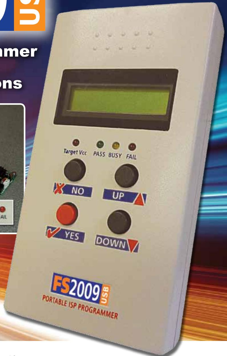
The **FS2009USB** is a **portable ISP programmer** designed for field-service and production programming applications. The programmer is capable of operating in '**Standalone Mode**' (without PC) allowing an operator to select from 1 of 64 '**Standalone Programming Projects**' using the display and keypad. A single '**Autoprogram**' key is then used to repetitively program the selected project.
