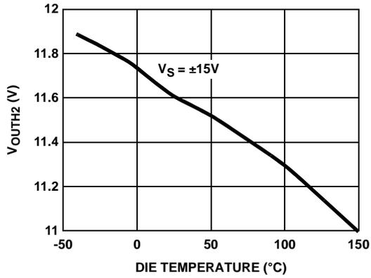
FIGURE 47. LOADED POSITIVE OUTPUT SWING vs TEMPERATURE
