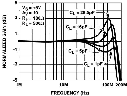
FIGURE 11. NON-INVERTING FREQUENCY RESPONSE FOR VARIOUS  $C_L$
