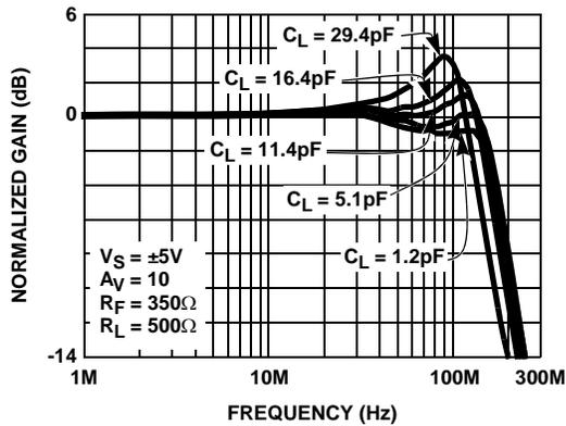
FIGURE 13. INVERTING FREQUENCY RESPONSE FOR VARIOUS  $C_L$
