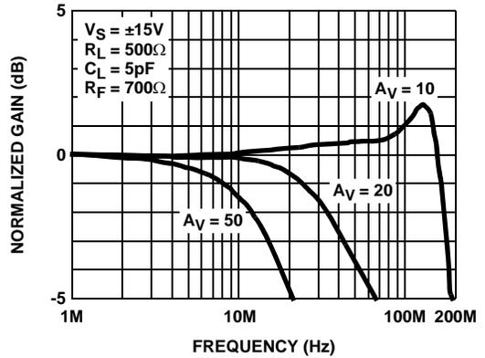
FIGURE 6. NON-INVERTING FREQUENCY RESPONSE FOR VARIOUS GAIN
