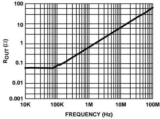
FIGURE 31. CLOSED LOOP OUTPUT IMPEDANCE vs FREQUENCY
