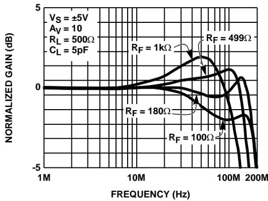
FIGURE 1. NON-INVERTING FREQUENCY RESPONSE FOR VARIOUS  $R_F$
