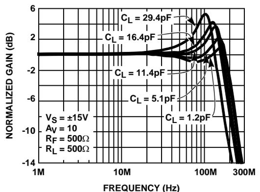
FIGURE 14. INVERTING FREQUENCY RESPONSE FOR VARIOUS  $C_L$
