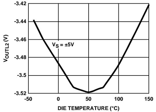
FIGURE 44. LOADED NEGATIVE OUTPUT SWING vs TEMPERATURE
