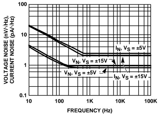
FIGURE 26. VOLTAGE AND CURRENT NOISE vs FREQUENCY
