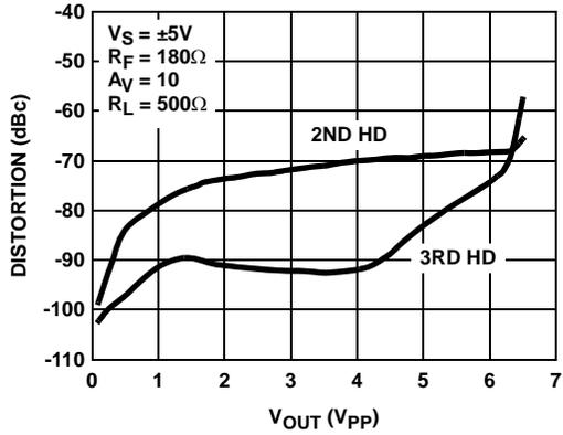
FIGURE 23. 1MHz HARMONIC DISTORTION vs OUTPUT SWING
