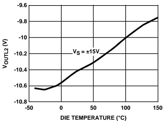
FIGURE 45. NEGATIVE OUTPUT SWING vs TEMPERATURE
