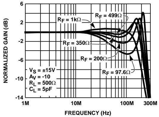
FIGURE 4. INVERTING FREQUENCY RESPONSE FOR VARIOUS  $R_F$
