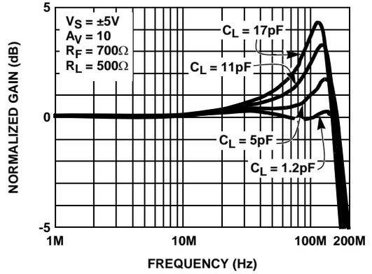
FIGURE 12. NON-INVERTING FREQUENCY RESPONSE FOR VARIOUS  $C_L$
