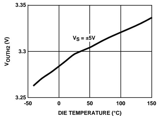
FIGURE 46. LOADED POSITIVE OUTPUT SWING vs TEMPERATURE
