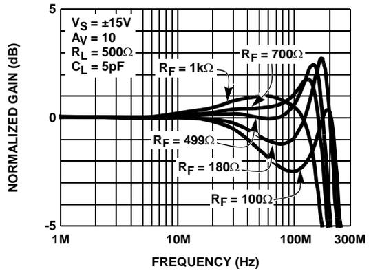
FIGURE 2. NON-INVERTING FREQUENCY RESPONSE FOR VARIOUS  $R_F$
