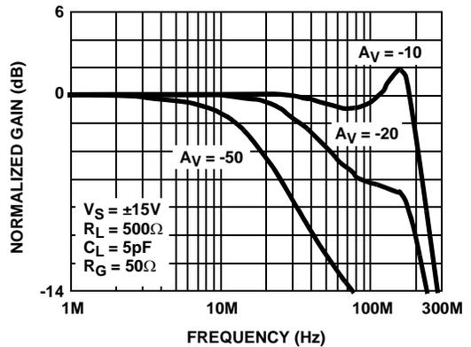
FIGURE 8. INVERTING FREQUENCY RESPONSE vs GAIN
