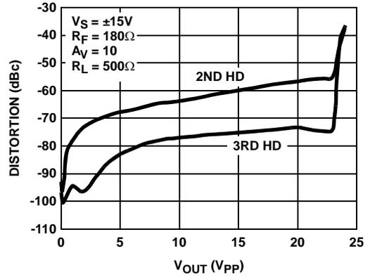
FIGURE 24. 1MHz HARMONIC DISTORTION vs OUTPUT SWING
